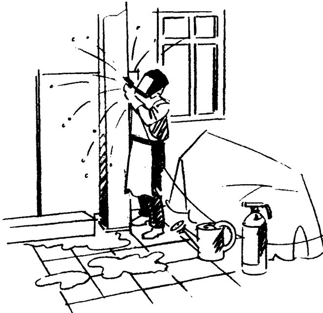
Figure 1.29 Risks are greatest in connection with temporary work in premises or areas not normally intended for welding
