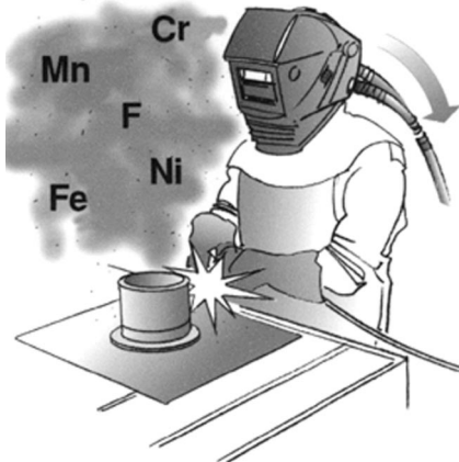
Figure 5.19 When welding in confined spaces where there is a risk that the concentration of fumes and gases could be too high, the welder must use breathing protection with a supply of clean air.
