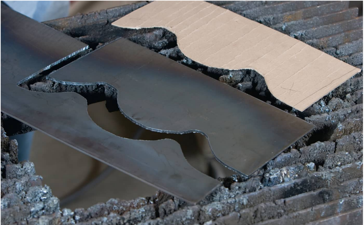
Cardboard templates can be folded or rolled into shapes for practice before bending the sheet-metal pieces.
