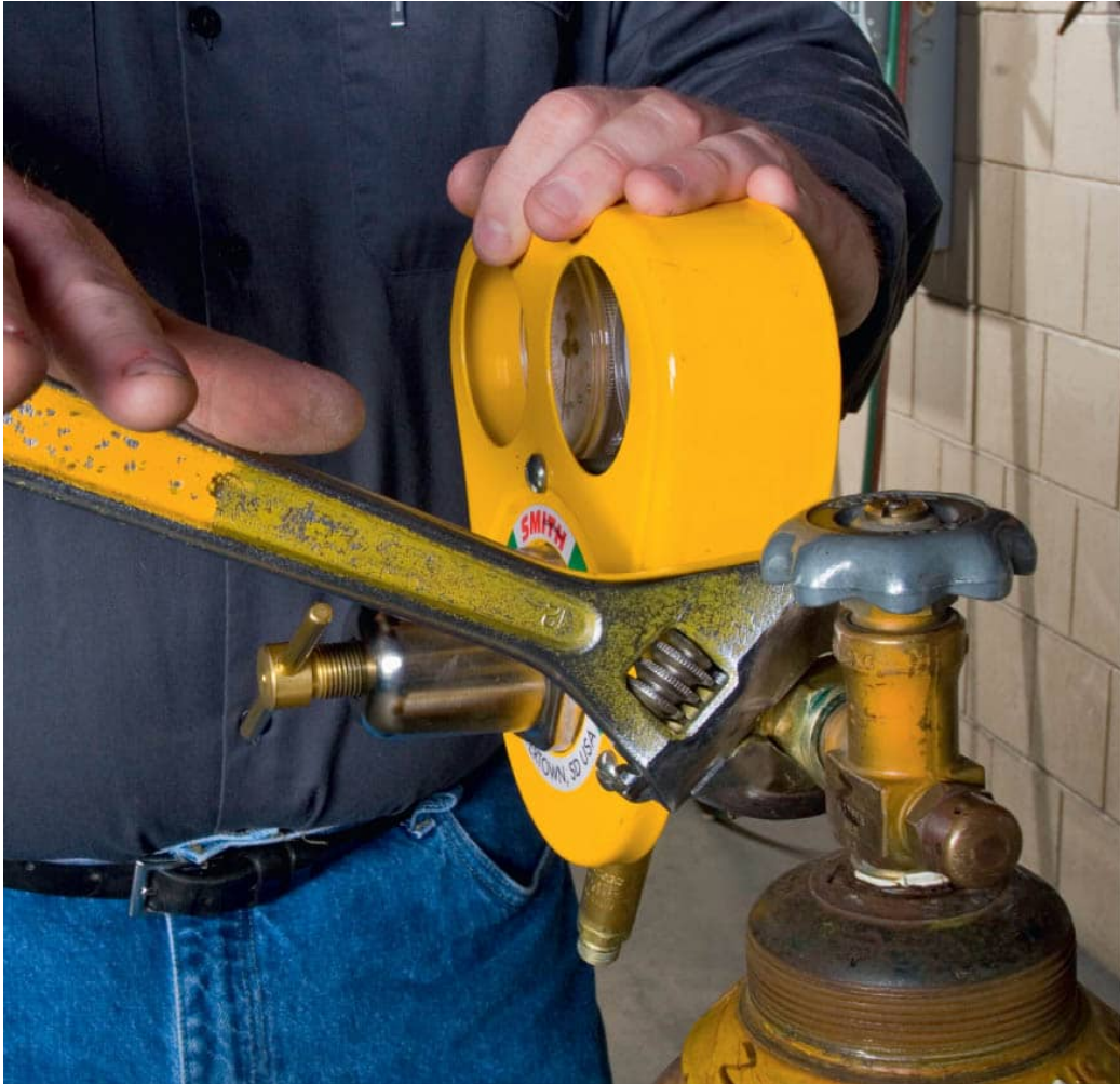
Use care with wrenches. Most fittings are made of soft brass and can easily be damaged.
