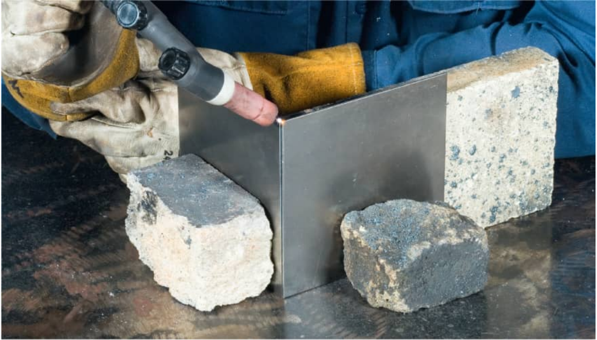
You can use almost any objects to keep parts in place when tacking as long as they can withstand high temperatures. These fire bricks are made to be safe around high heat.
