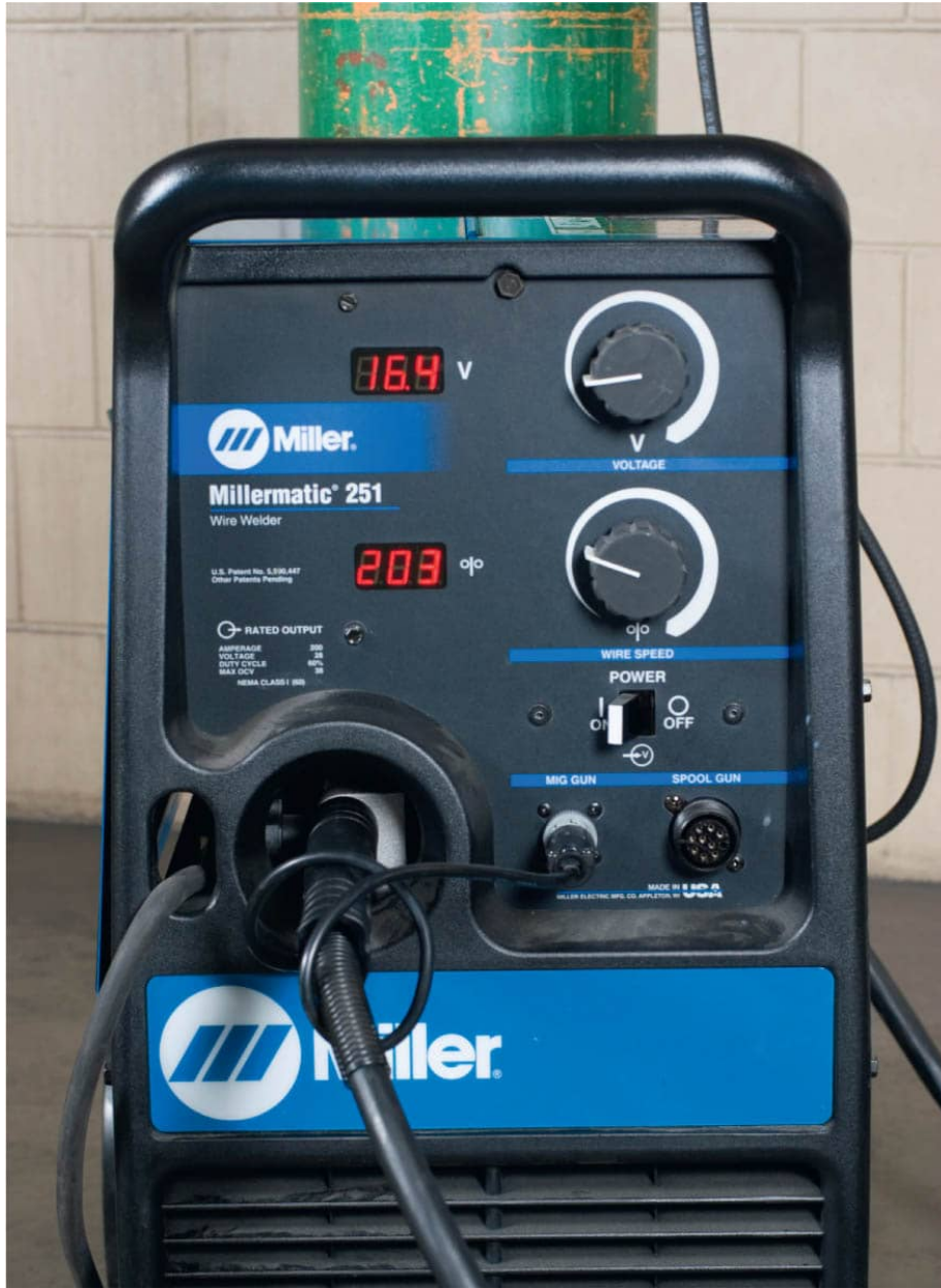
Voltage and wire feed speed are set on a constant-voltage machine for MIG welding.
