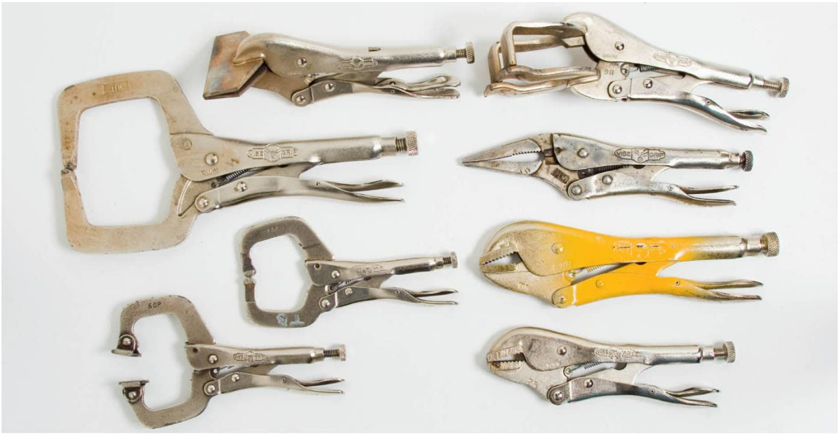
Vise-Grips come in a wide variety of shapes and sizes for general and specialized uses.
