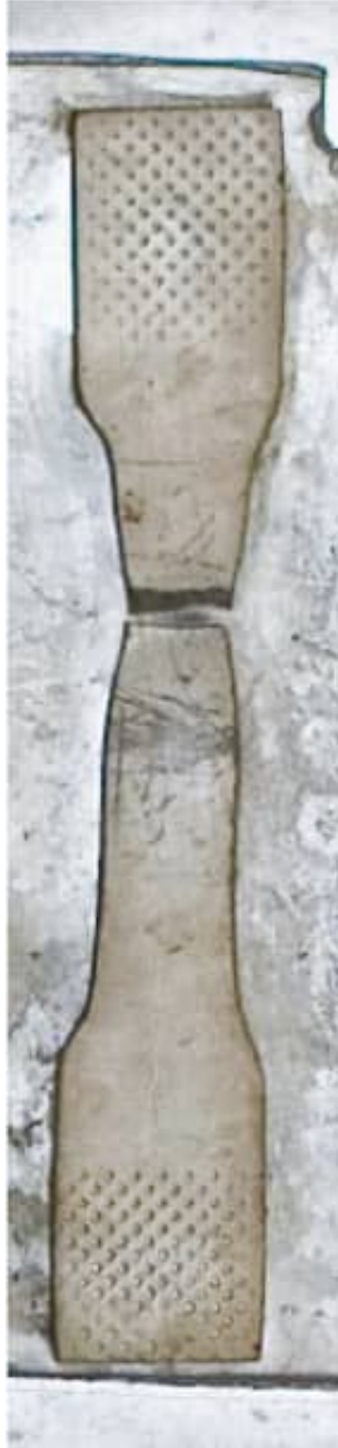
This tensile test example pulled apart under a heavy load. Notice how the metal stretched before breaking.
