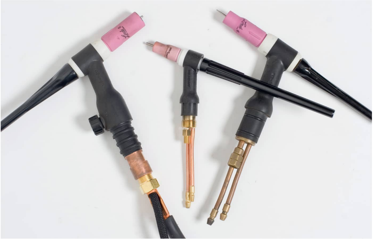
Air-cooled and water-cooled torches contain small parts. Be careful not to bend or overtighten the components.
