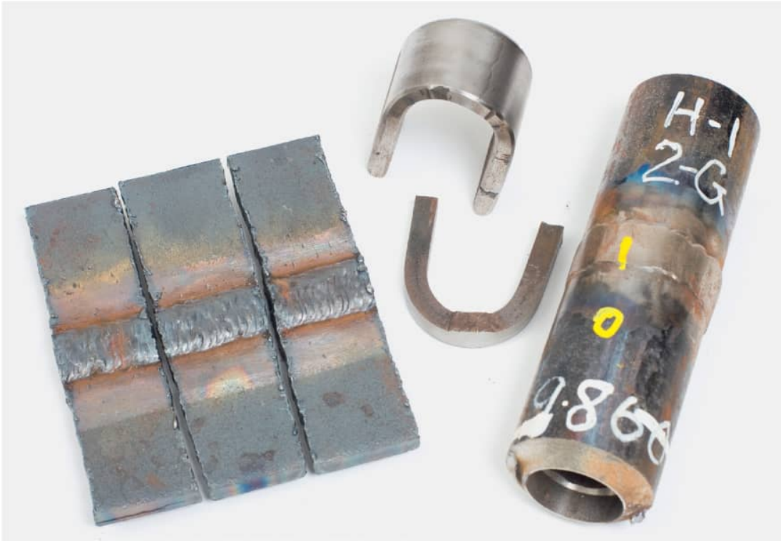
Weld tests on pipe and plate are cut into strips and bent to test the strength of the welds.
