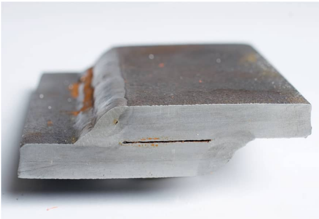
A lap joint cross-section shows two fillet welds. The welder used multiple passes to make “full-sized” welds.
