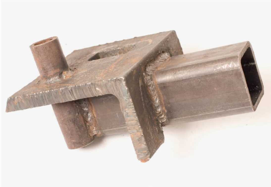
Short pieces of tube and angle can be cut, notched, and welded for practice to simulate the joint on an actual project.
