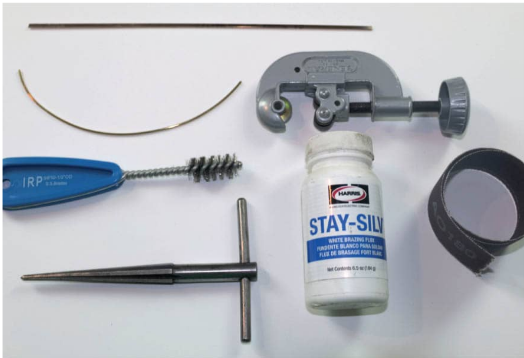
Tools for brazing include flux, brazing alloy, sandpaper, a wire brush for cleaning the inside of the tube, a tube cutter, and a reamer for deburring.
