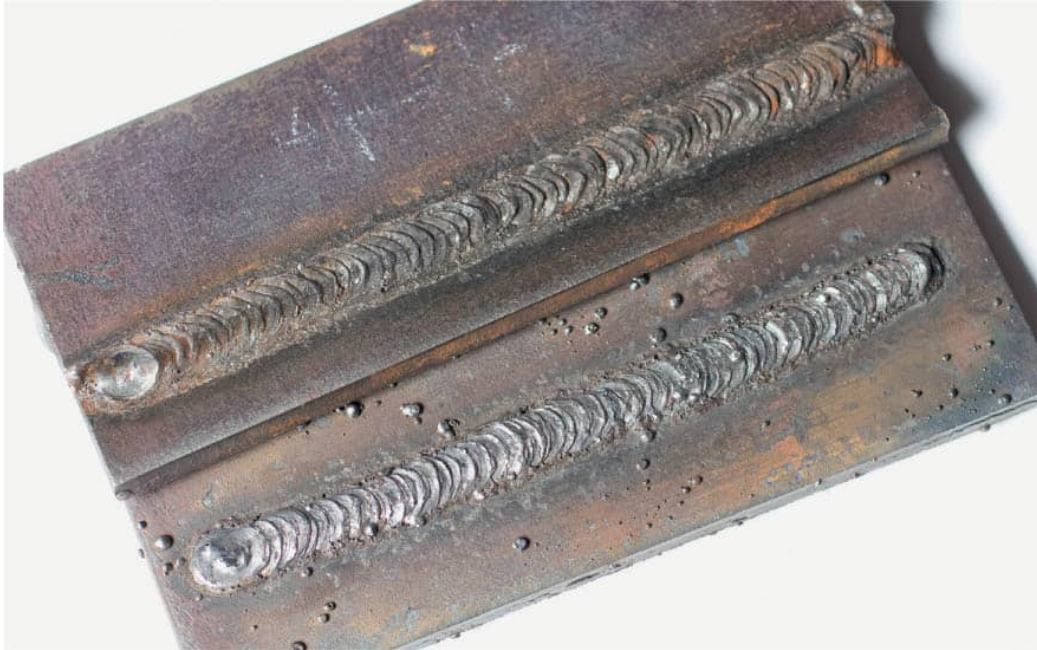
6010 and 6011 welds can have a stacked coin appearance using the whip technique.
