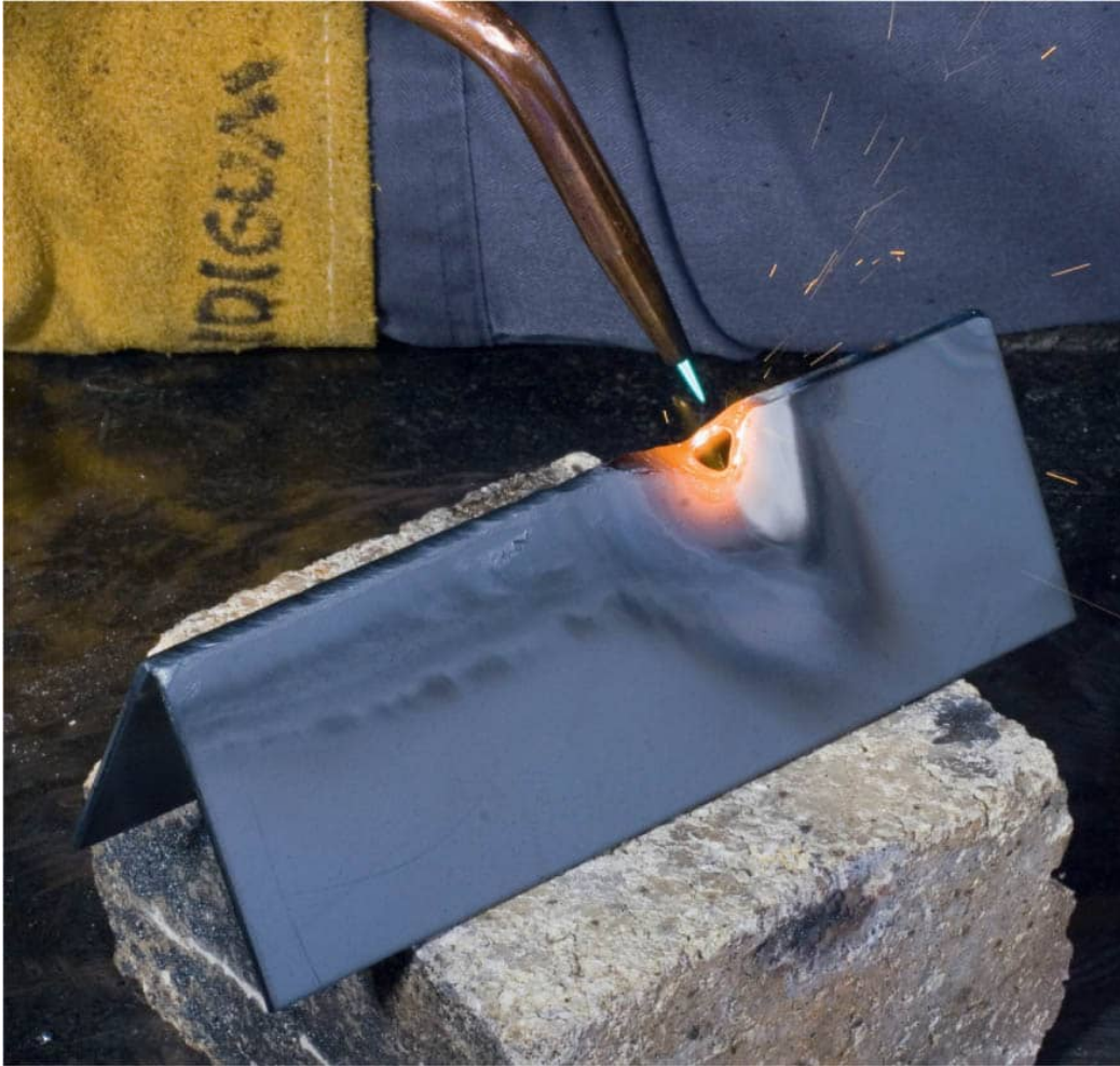
Traveling too slowly on thin metal can cause burn-through, creating a hole in the metal.
