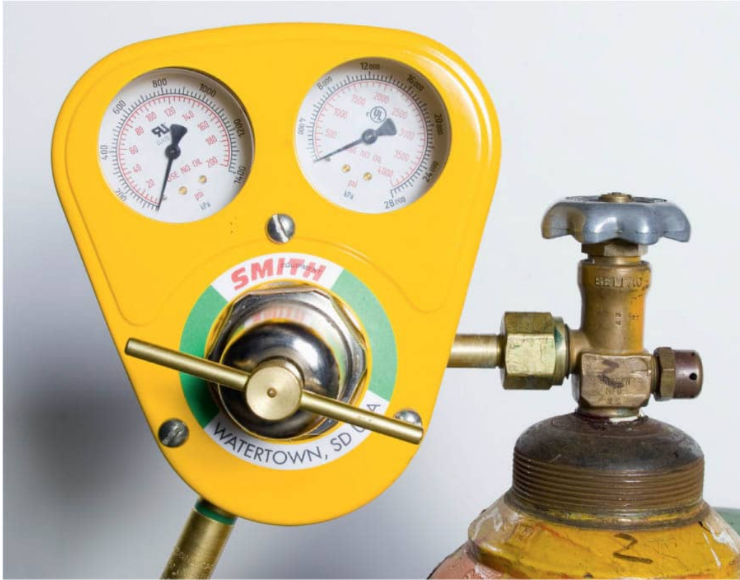
Both regulator gauges read 0 pressure, which means there is no gas in the hose and the cylinder valve is closed.
