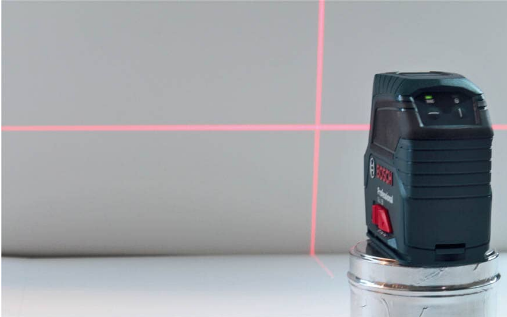
Self-leveling lasers used for fabrication and construction display perfectly horizontal and vertical lines.
