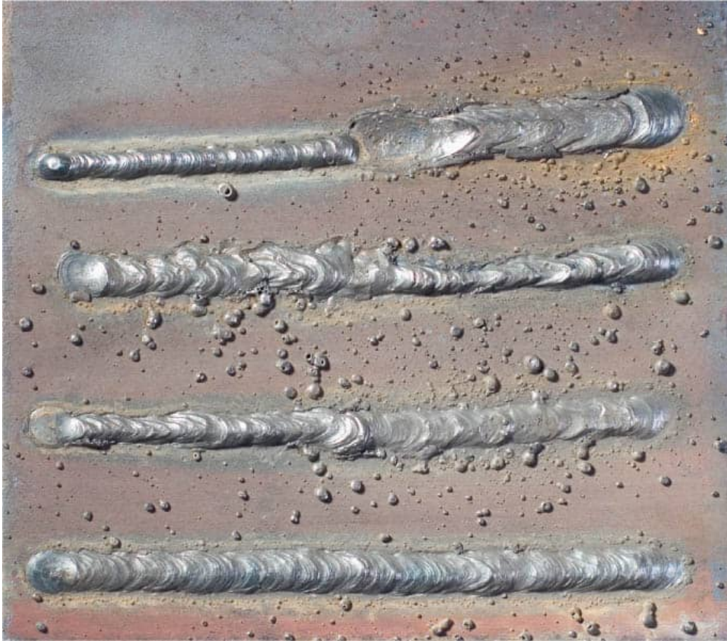
Beads from top to bottom: amps too low or too high; arc too long; incorrect angle; bead correct with uniform width and even ripples.
