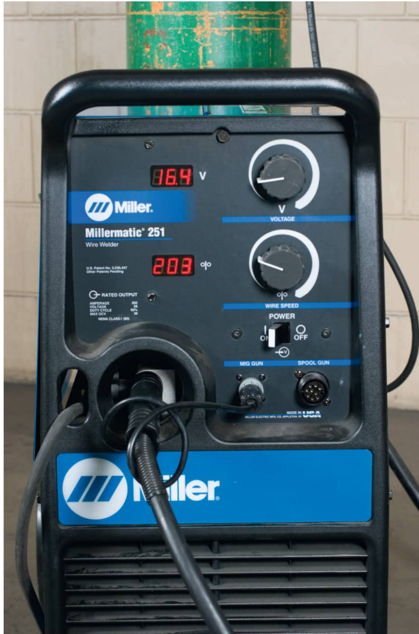
Two controls are used to adjust heat for wire-feed welding. This machine is set at 16.4 volts and a wire-feed speed of 203 inches per minute.
