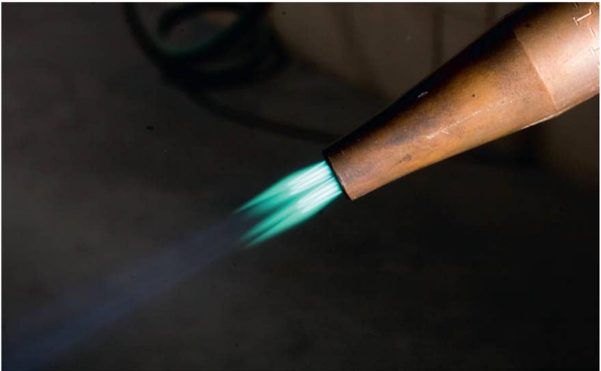
With the cutting jet lever pressed down, a feather appears, indicating a slightly carburizing flame.
