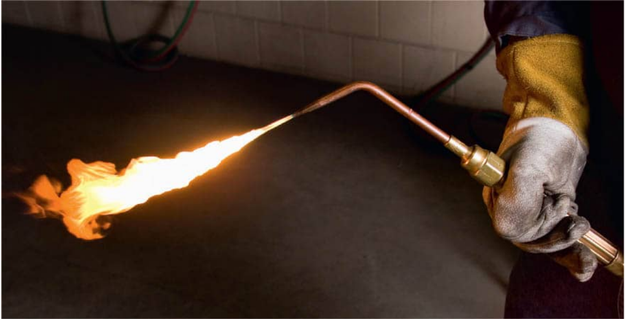
Adjust the acetylene gas first before adding oxygen to control the volume of heat in the oxy/acetylene flame.
