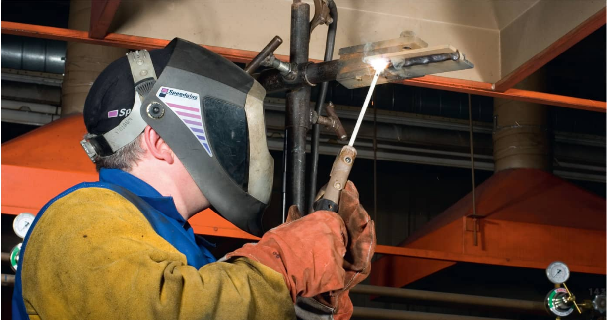
When working overhead, try to get underneath the bead for the best view of the weld as you are making it.
