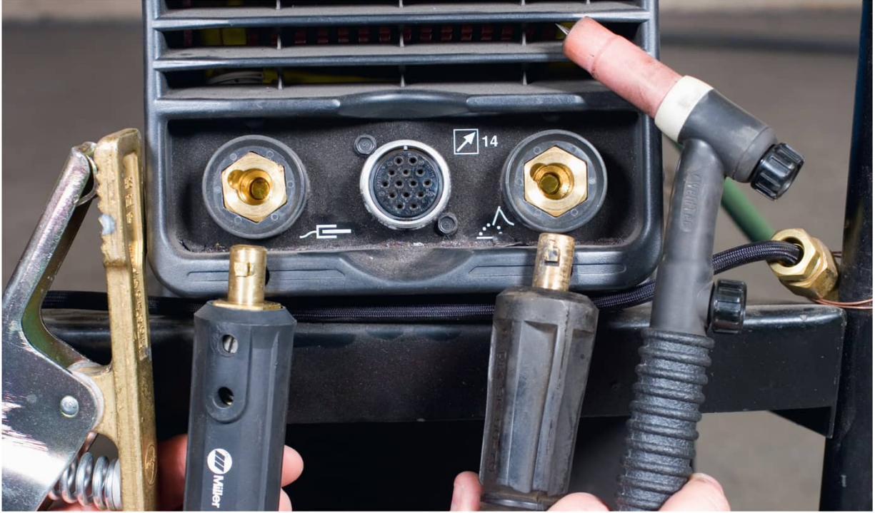
These Dinse-type connectors twist into place. DCEN is used when the torch is negative and the work clamp is positive.
