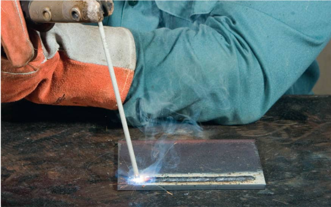
Proper electrode travel angle is almost 90 degrees to the piece being welded. This allows the arc to better penetrate the metal.
