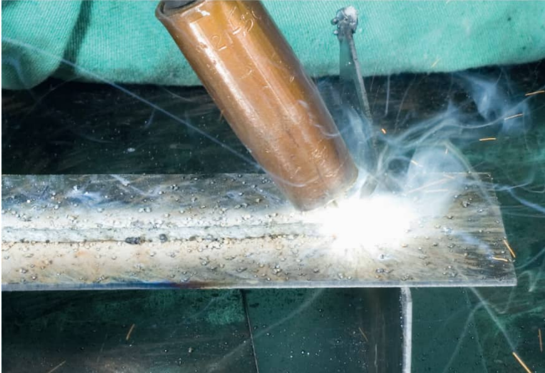
Self-shielded flux-core wires create a shielding vapor around the weld. No shielding gas is used with this type of wire.
