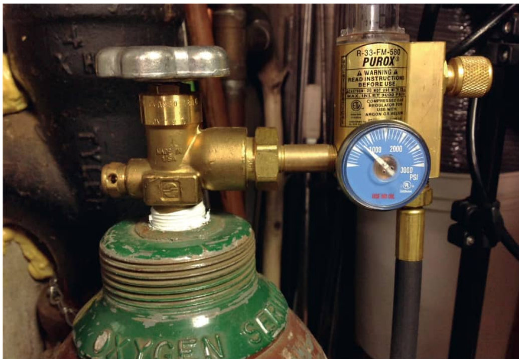
The flow meter gauge indicates there are 650 pounds per square inch (psi) of argon gas left in this cylinder.
