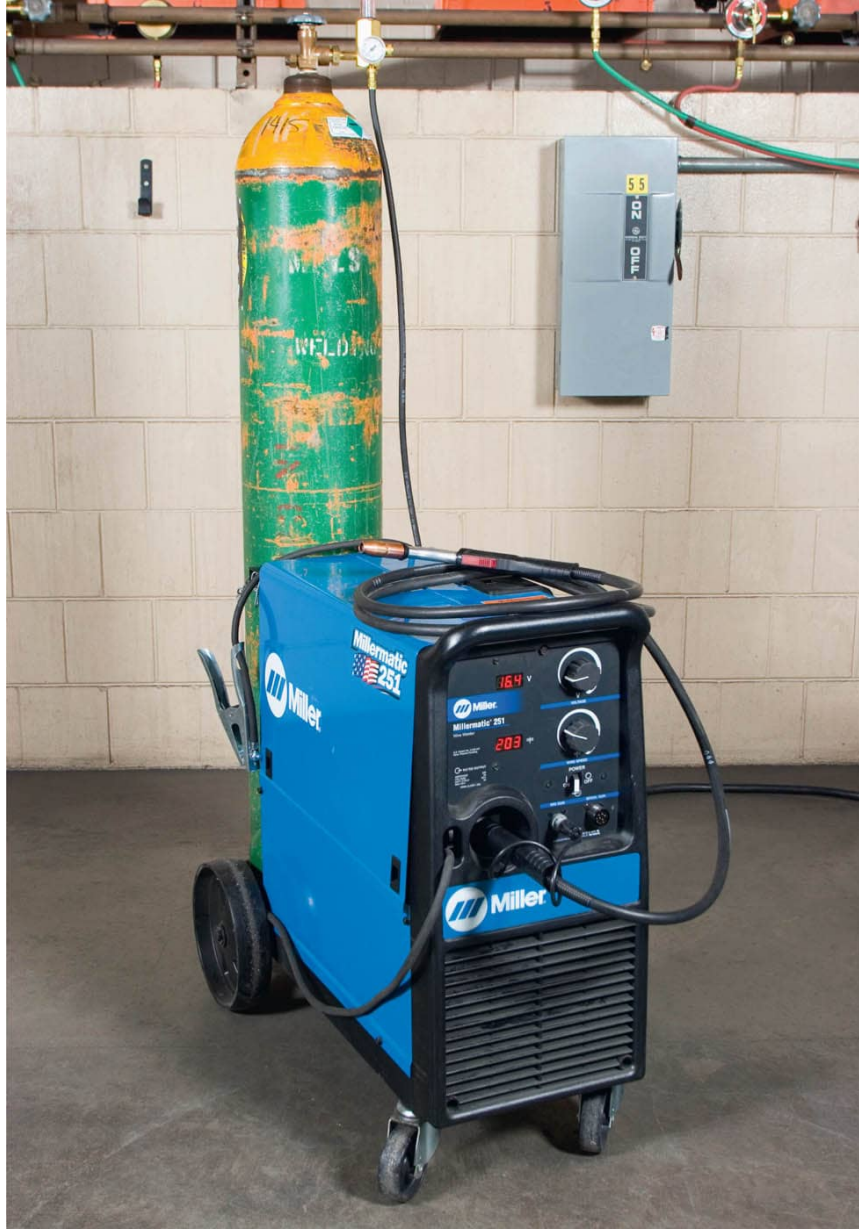
A spool gun is available for this wire feed machine to weld aluminum. In addition, a 100 percent argon shielding gas is required.
