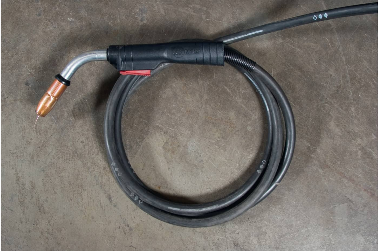
Wire feed gun cables have a liner that can be damaged if the cable is bent or tightly coiled.
