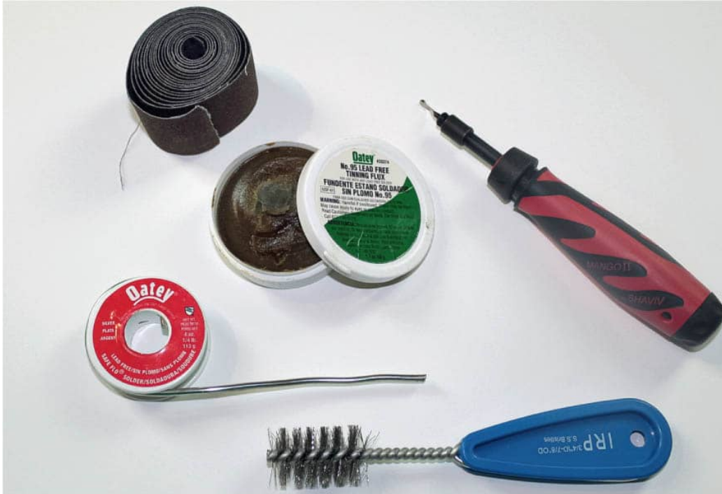
Tools for soldering include flux, solder, sand cloth, a wire brush, and a tool for deburring the tube after it is cut.
