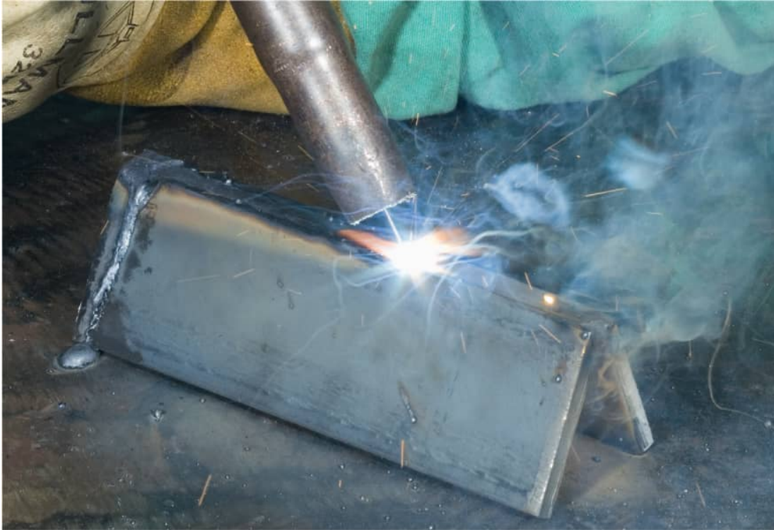
Gas-shielded flux-core wires work well for welding steel plates. After welding, a slag coating covers the bead.
