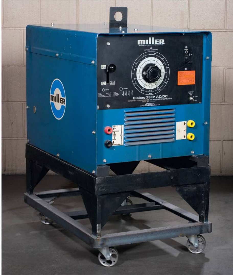
Transformer-rectifier welding machines are big and heavy. Fabricating a frame with wheels makes it easier to move around.
