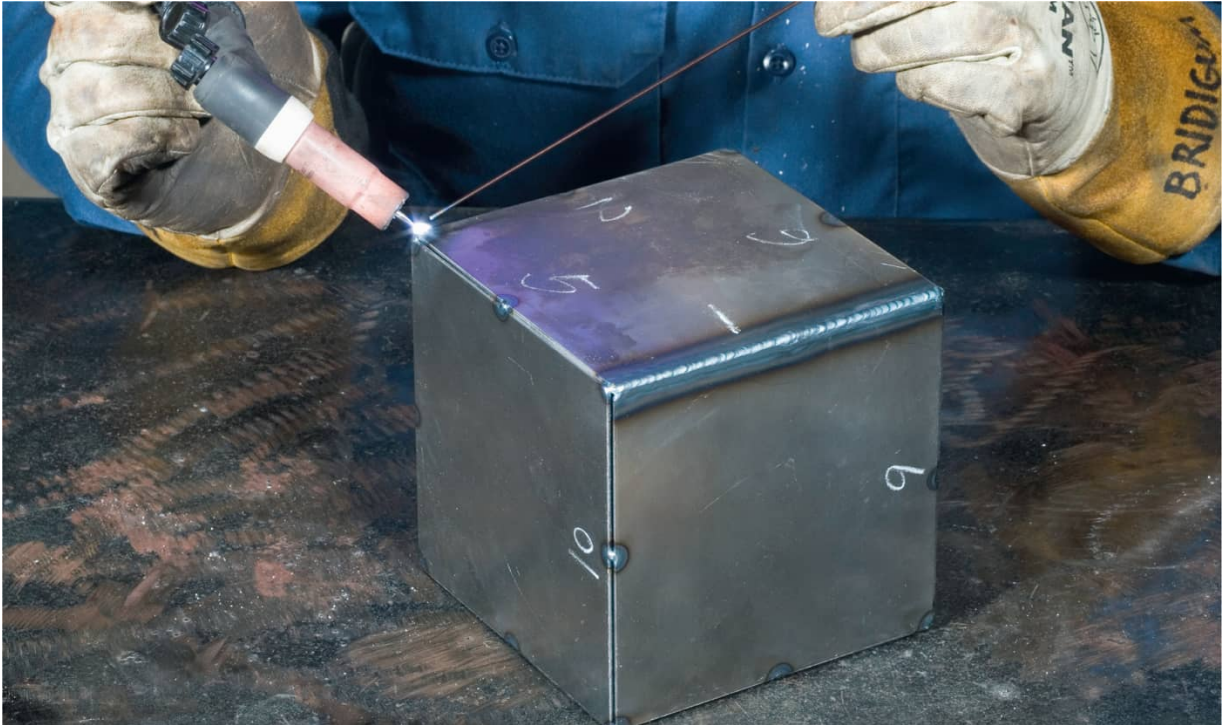
Numbers were put on this cube project to keep track of the weld sequence. Distortion is reduced by skipping around to different areas.
