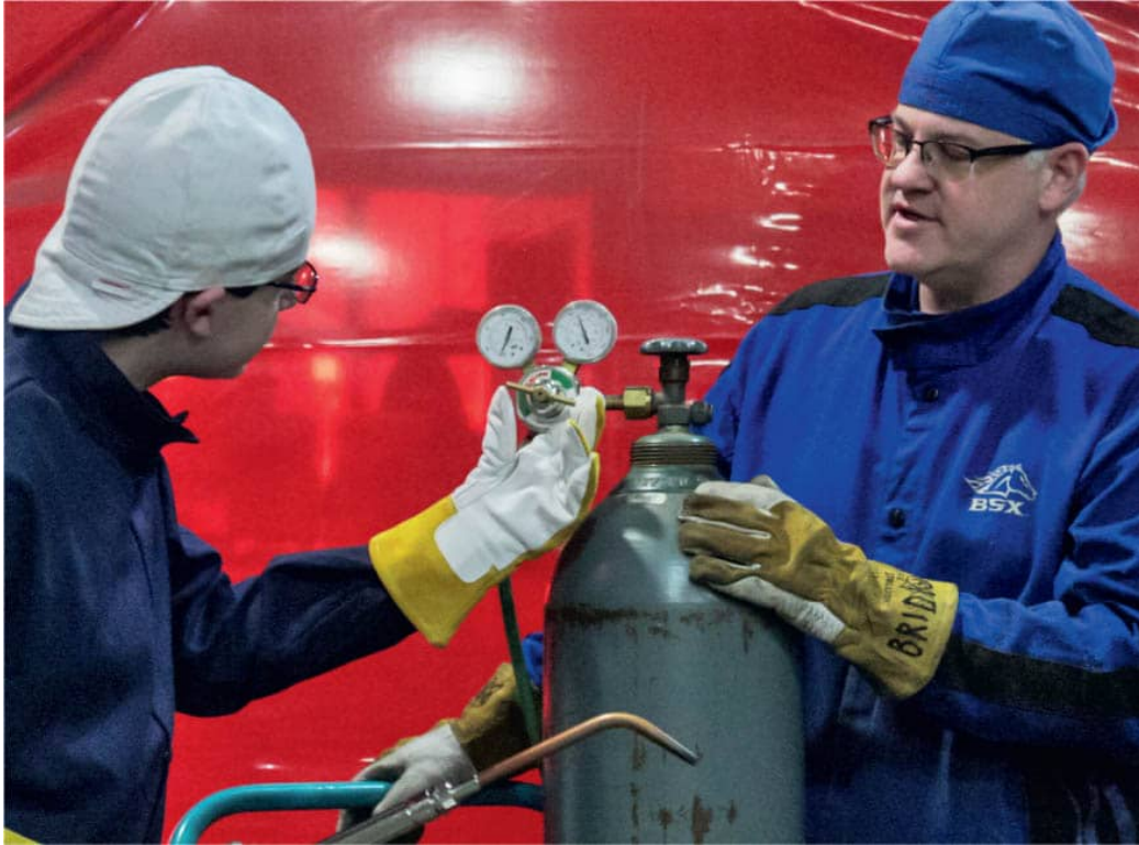
As you turn the regulator adjusting screw clockwise, watch the low-pressure gauge to see how much gas is entering the hoses.
