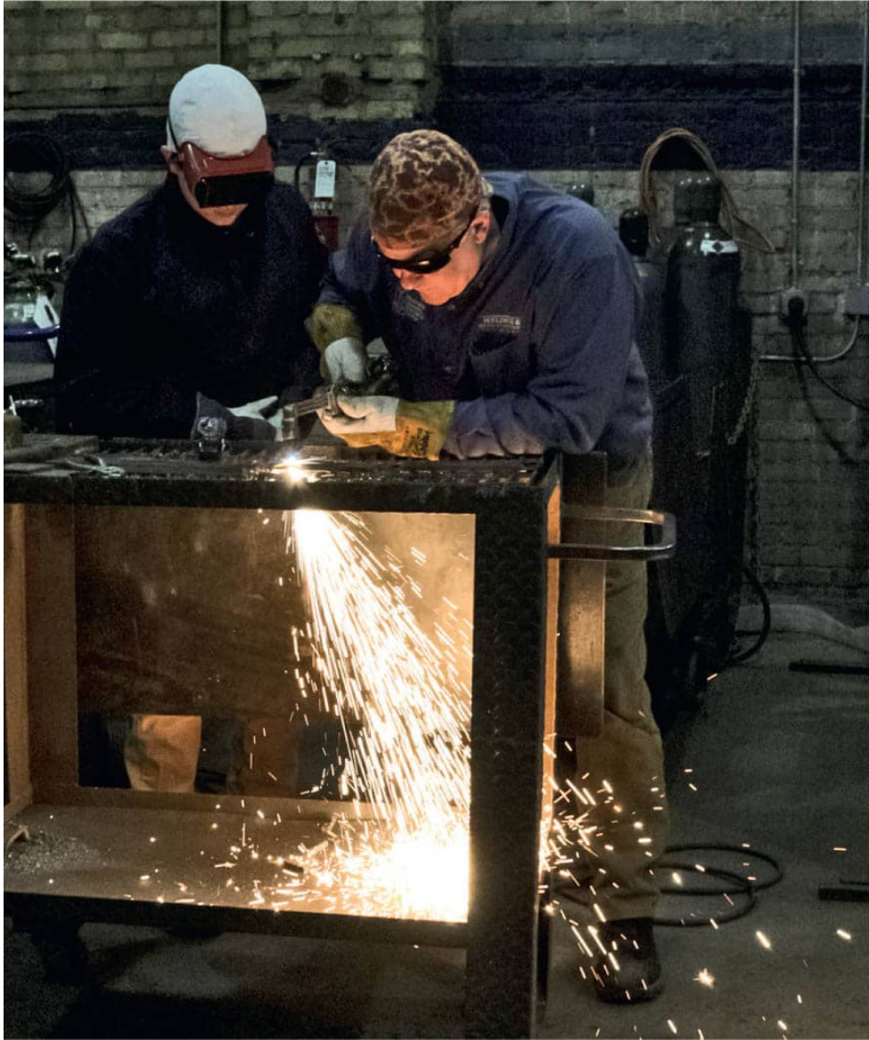
Resting one arm on the table for stability is easier with thick gloves and a welding jacket providing protection from the heat.
