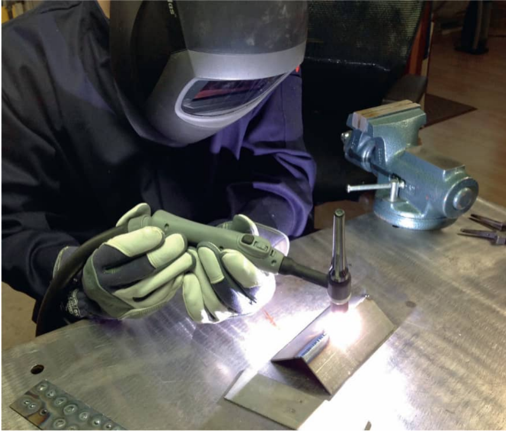
Start to learn TIG welding by holding only the torch and fusing two pieces of metal together.
