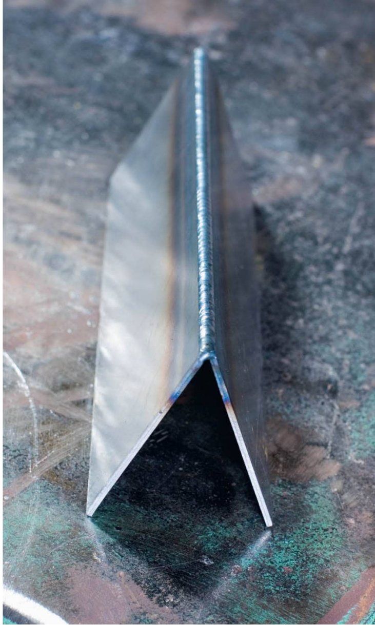
Open corner joints have welds that are evenly rounded on the face with a smooth transition to the sides.
