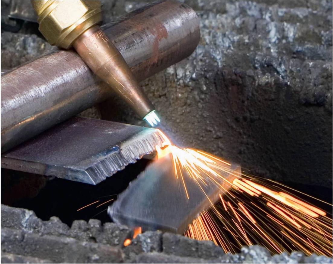
An oxygen jet leaves small grooves in the cut metal, which you can polish out with a grinder.
