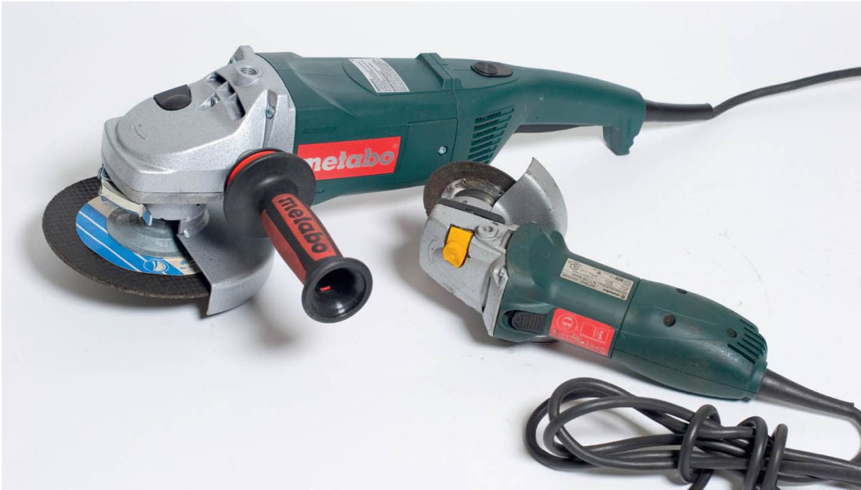
Grinders may have different wheels attached for removing and smoothing metal surfaces.
