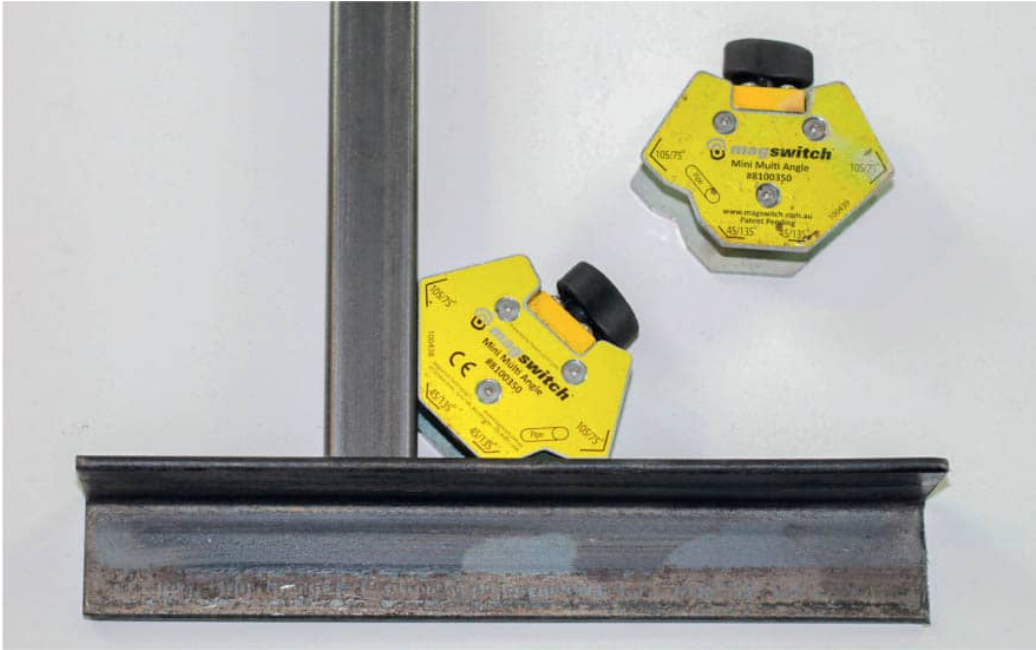
Switchable magnets hold steel parts together and are easy to clean because the magnet can be turned on and off.
