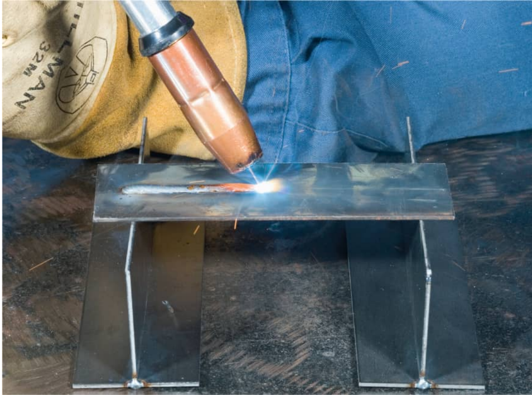
Short-circuit MIG uses a solid wire and shielding gas, making the weld easy to see.
