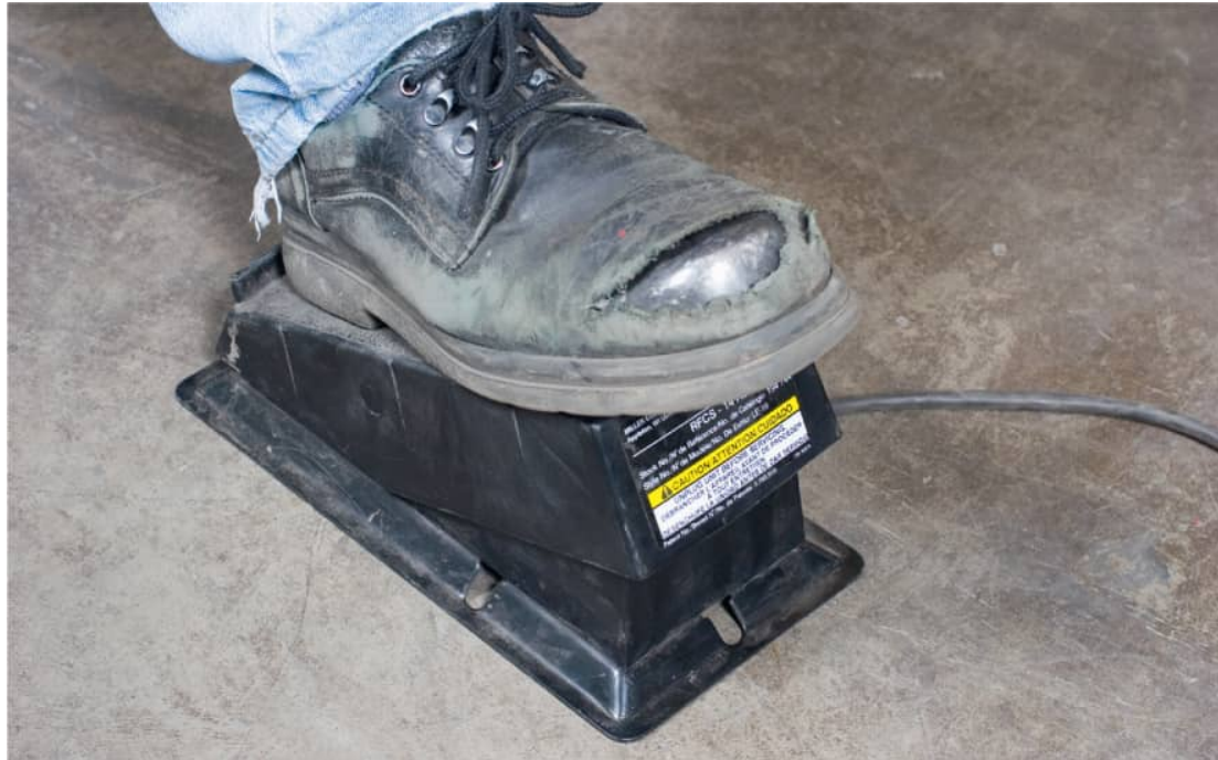
Remote start controls, such as foot pedals, are used to establish the arc and to increase or decrease the amount of heat.
