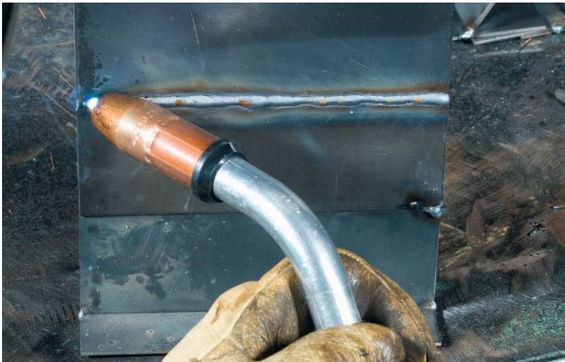
Push a MIG gun when welding horizontally on thin sheet metal to reduce the chances of burning through.
