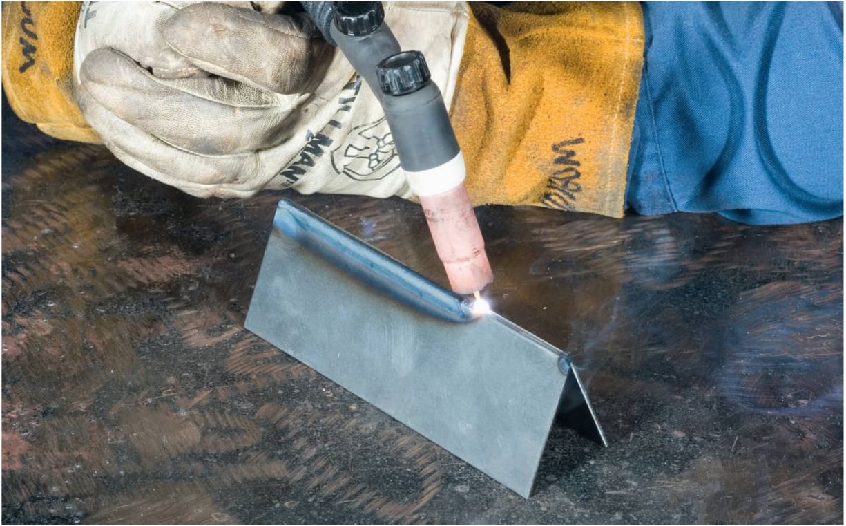
You can use a TIG torch to fuse metals together without using a filler rod. This is called an autogenous weld.
