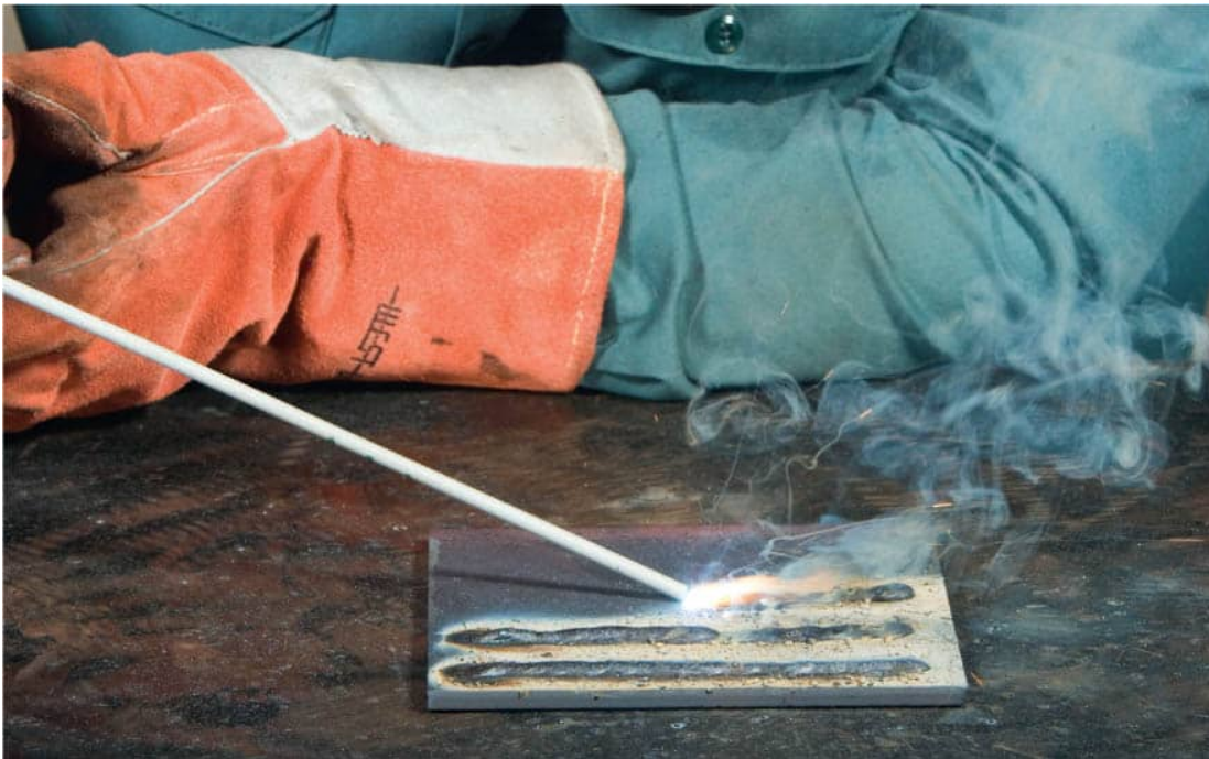
Shallow electrode angles cause the arc to bounce off the metal with little penetration.
