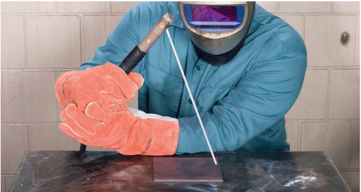
Placing welding rods at different angles in an electrode holder makes it easier to maintain the correct angle.
