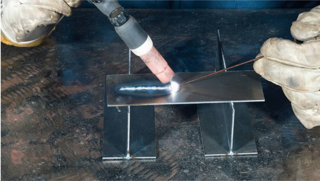
TIG and oxy/acetylene torches work in similar ways. Use a push technique and add filler metal by dipping it in the puddle.
