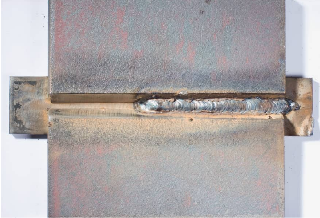
Thick plate butt joints often have beveled edges and a root opening to achieve better penetration. A backup bar bridges the gap between pieces.
