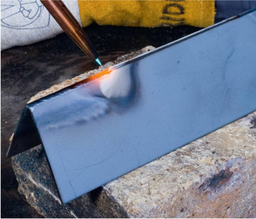
Use a push technique for oxy/acetylene welding: point the torch in the direction of travel.
