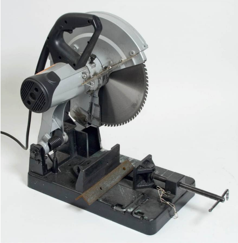
Metal-cutting chop saws cut a wide variety of structural shapes, including tubing, angle iron, and channel.
