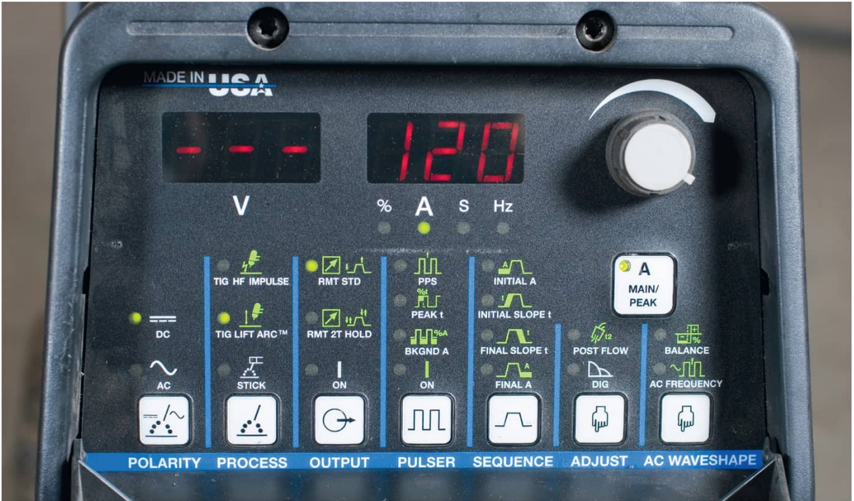
TIG power sources can have many different controls. This machine is set for 120 amps, which is enough heat to weld 1/8-inch-thick metal.
