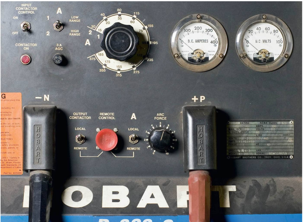
This older stick machine has two meters indicating the actual voltage and amperage while the weld is being made.
