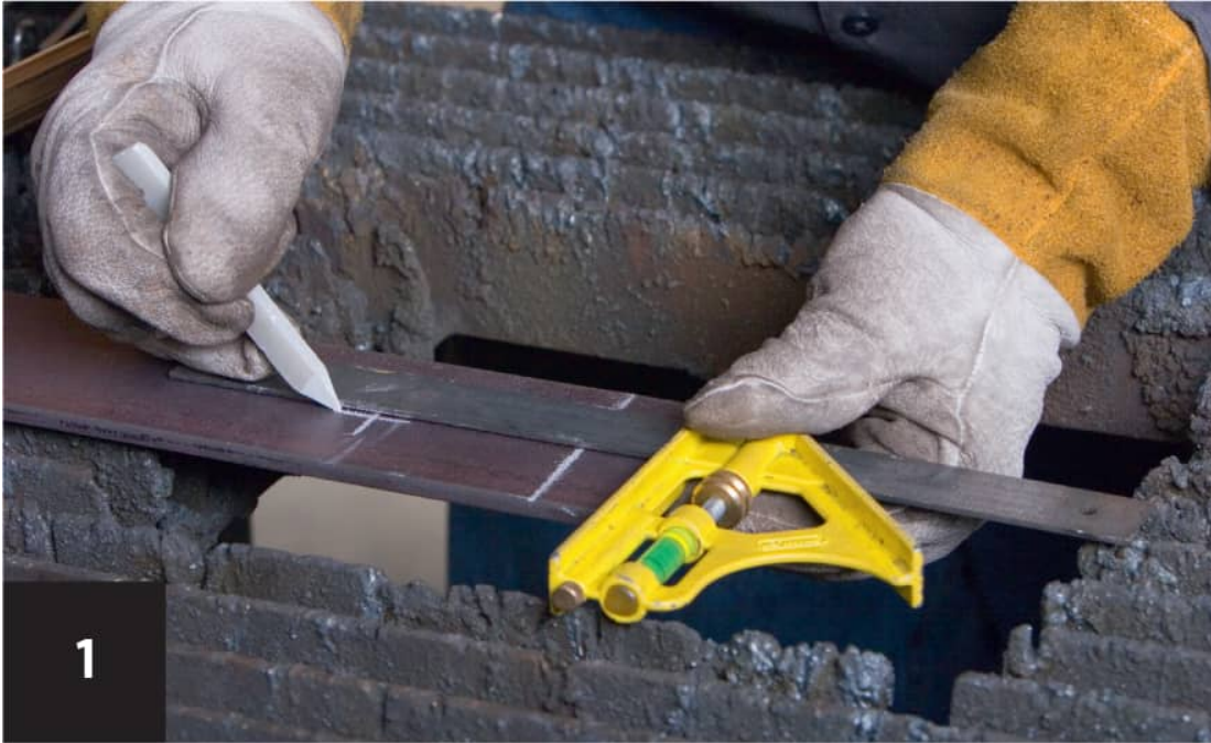
A combination square works well for laying out cut lines with soapstone.
