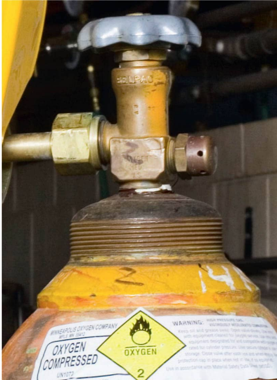
Oxygen cylinder valves are opened all the way, allowing oxygen to flow into the attached regulator on the left.
