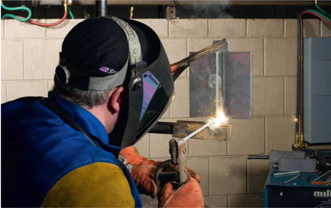
Stick welding vertically requires less heat than welding horizontally. Turn down the amperage until the weld puddle stays in the joint.
