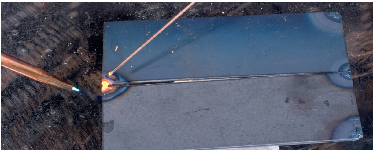
Tacking two pieces together with a gap between them allows penetration into the center of the joint.
