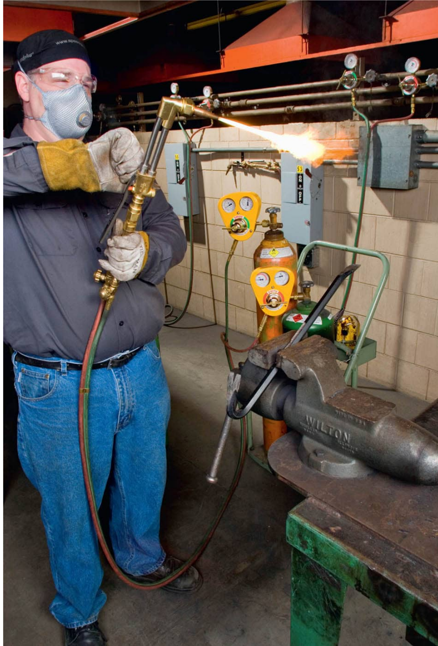
Wear a respirator when heating or welding metals that are painted or coated.
