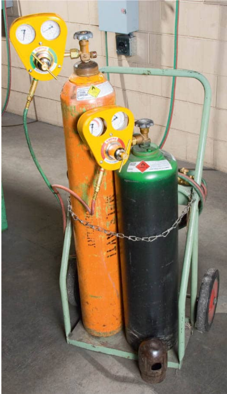
Larger oxy/acetylene torch setups are usually put on a two-wheel cart to make it easier to move around the work area.
