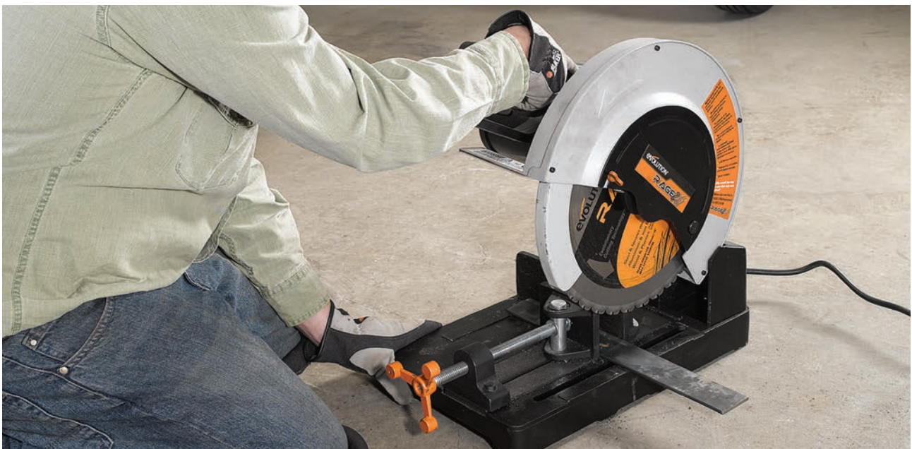
Cut the coupler plates to size using a chop saw.
