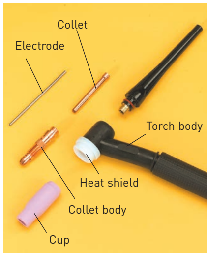
Parts of a gas tungsten arc welding torch.
