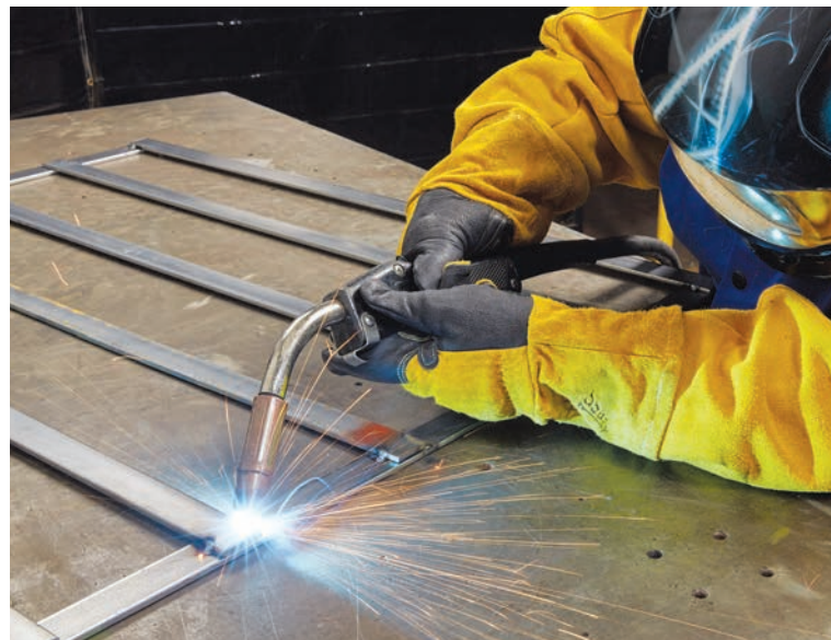
Position five pieces of part B at 6" on-center intervals across the frame. Measure to ensure both sides are evenly spaced, and then tack the pieces in place. Weld the assembly.
