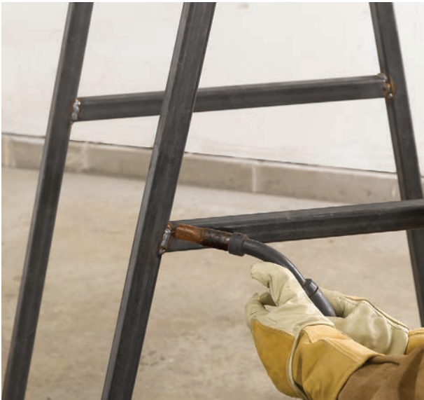
Tack the horizontal leg connectors (G) and then center cross piece (H) that spans between the two leg connectors.
