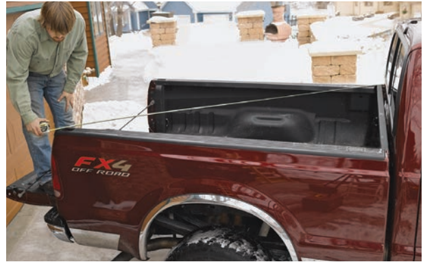
Measure from corner to corner of the truck bed for square.
