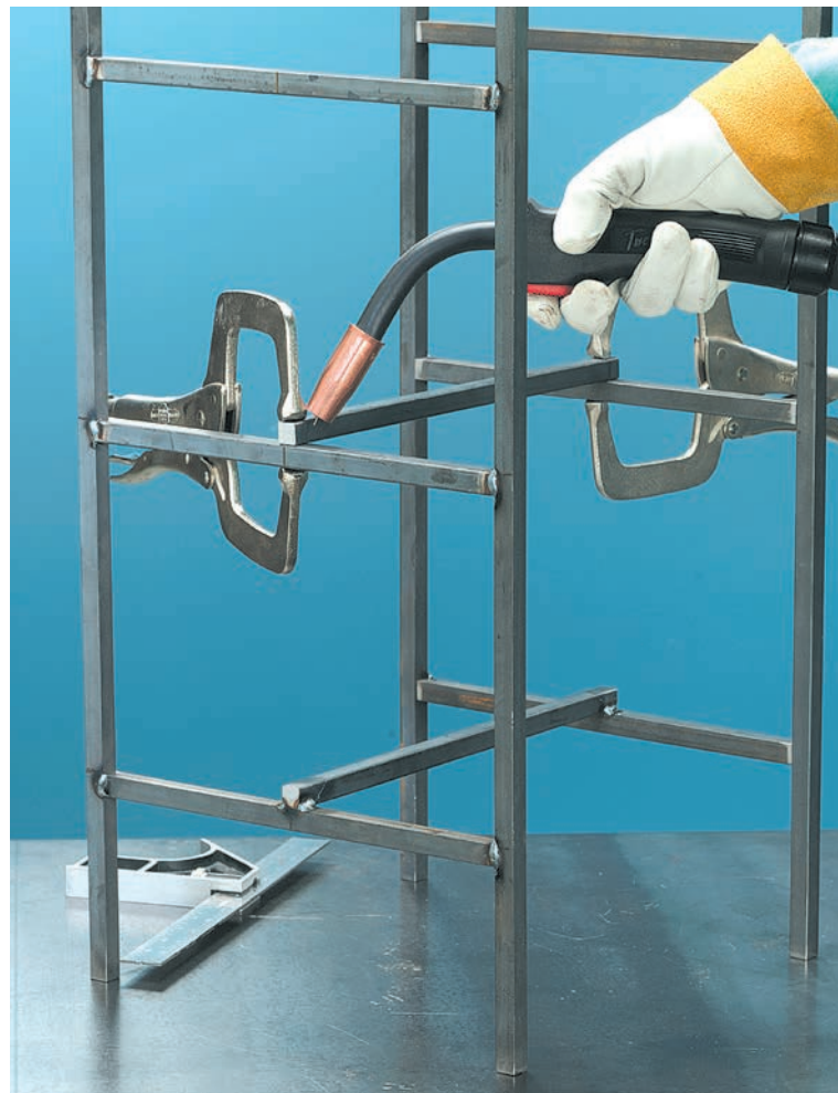
Clamp the center bottle holders to the leg assemblies and tack weld in place.
