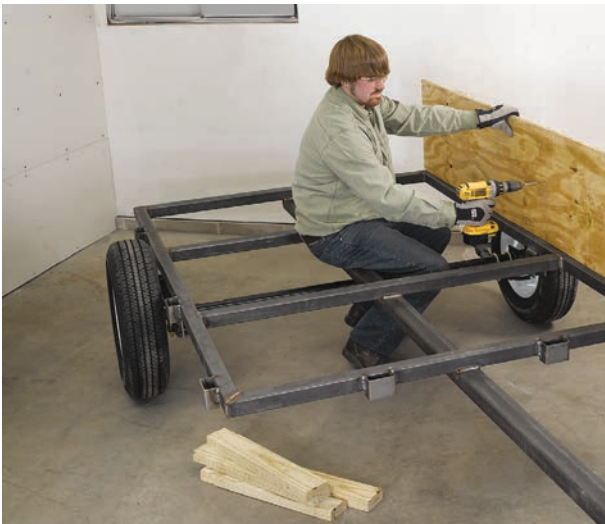
Fasten ¾"-thick plywood trailer sides to the exterior-rated 2 × 4 stakes.
