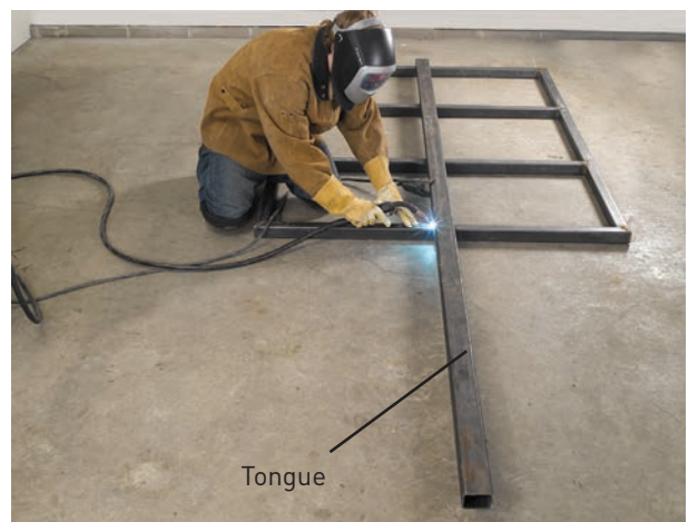
Weld the trailer tongue to the underside of the frame.
