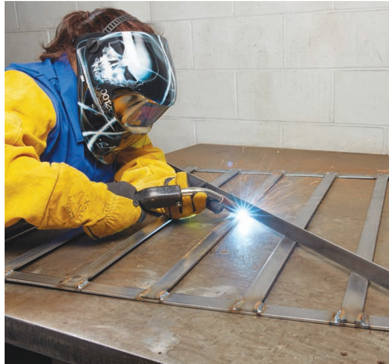
Place and weld the stiffener on its edge.
