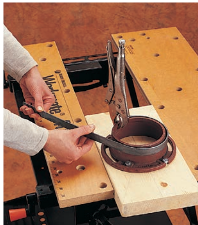
Use locking pliers to hold the metal to the jig. Wrap the metal around the jig in a smooth motion.
