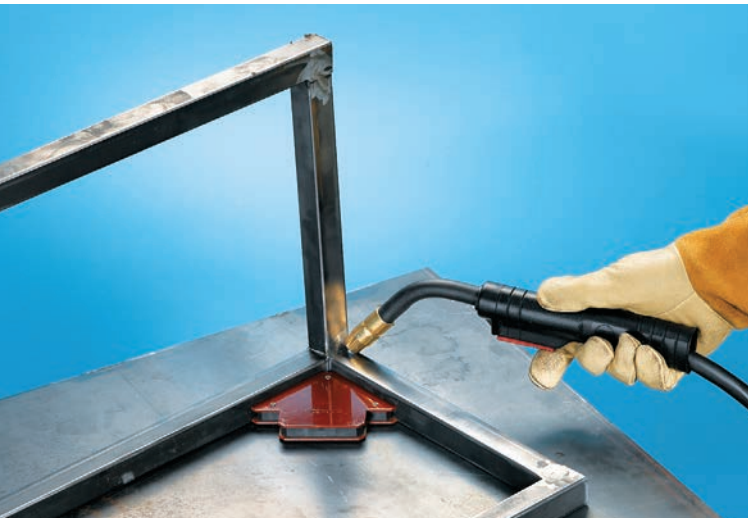
Attach the third leg and crosspieces to create a 90° angle.
