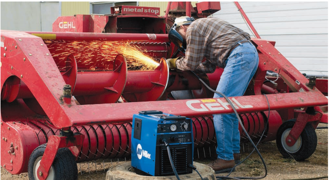
A Miller plasma cutter is being operated by a gasoline generator and an air compressor to make a repair on this hay baler. When the broken part is removed, a replacement will be welded on by a wire-feed machine.
