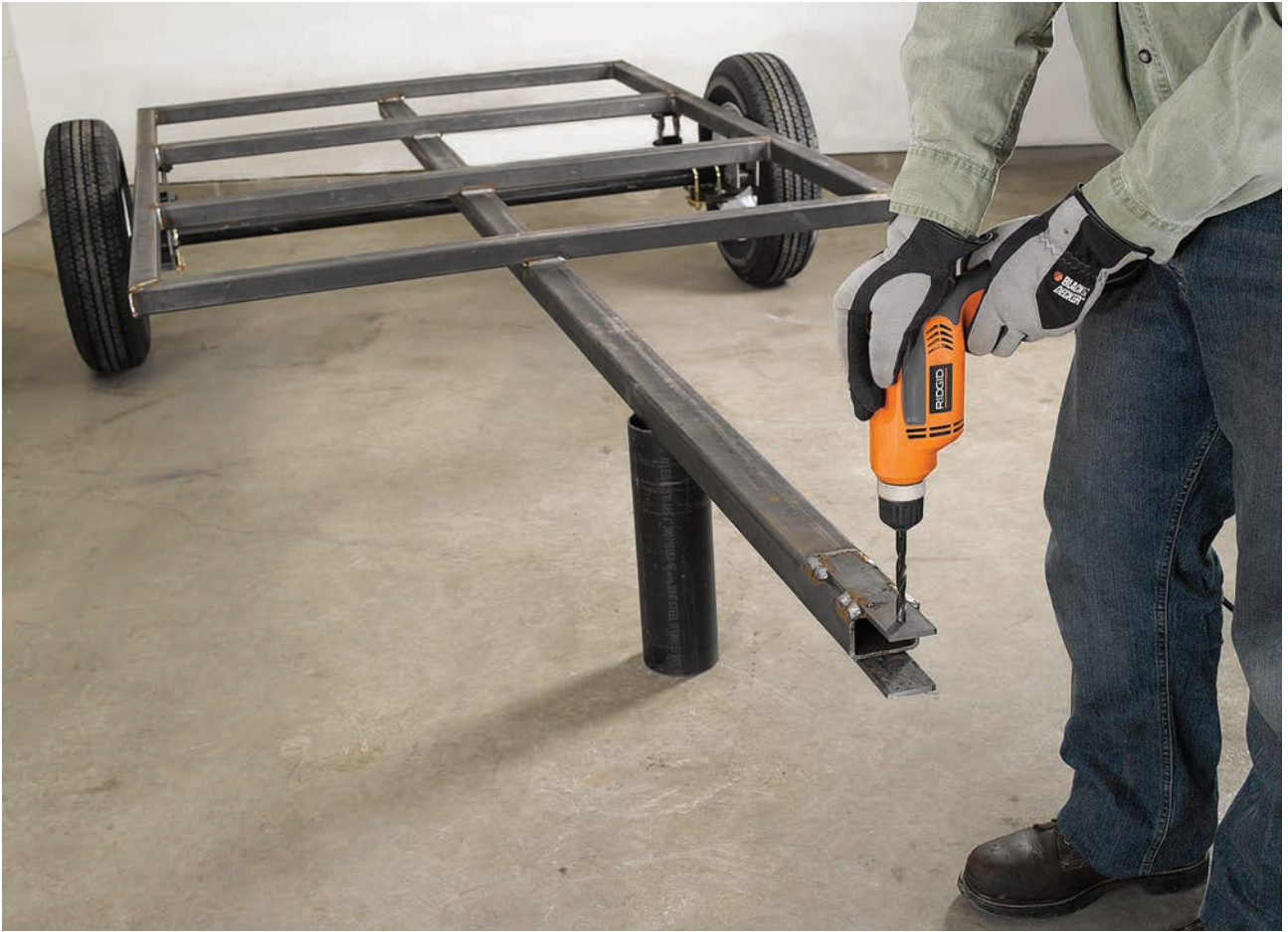
Drill holes into the coupler plates according to the coupler specifications.
