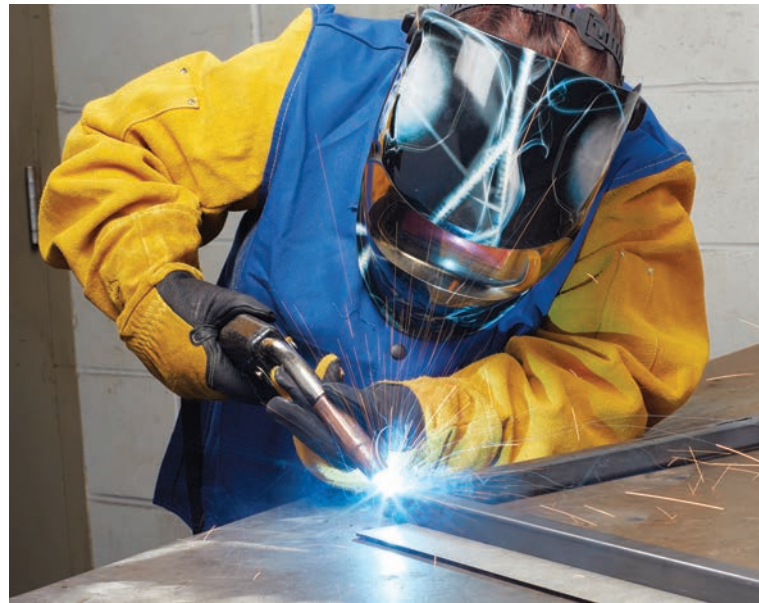
Weld flat bar support tabs in place.
