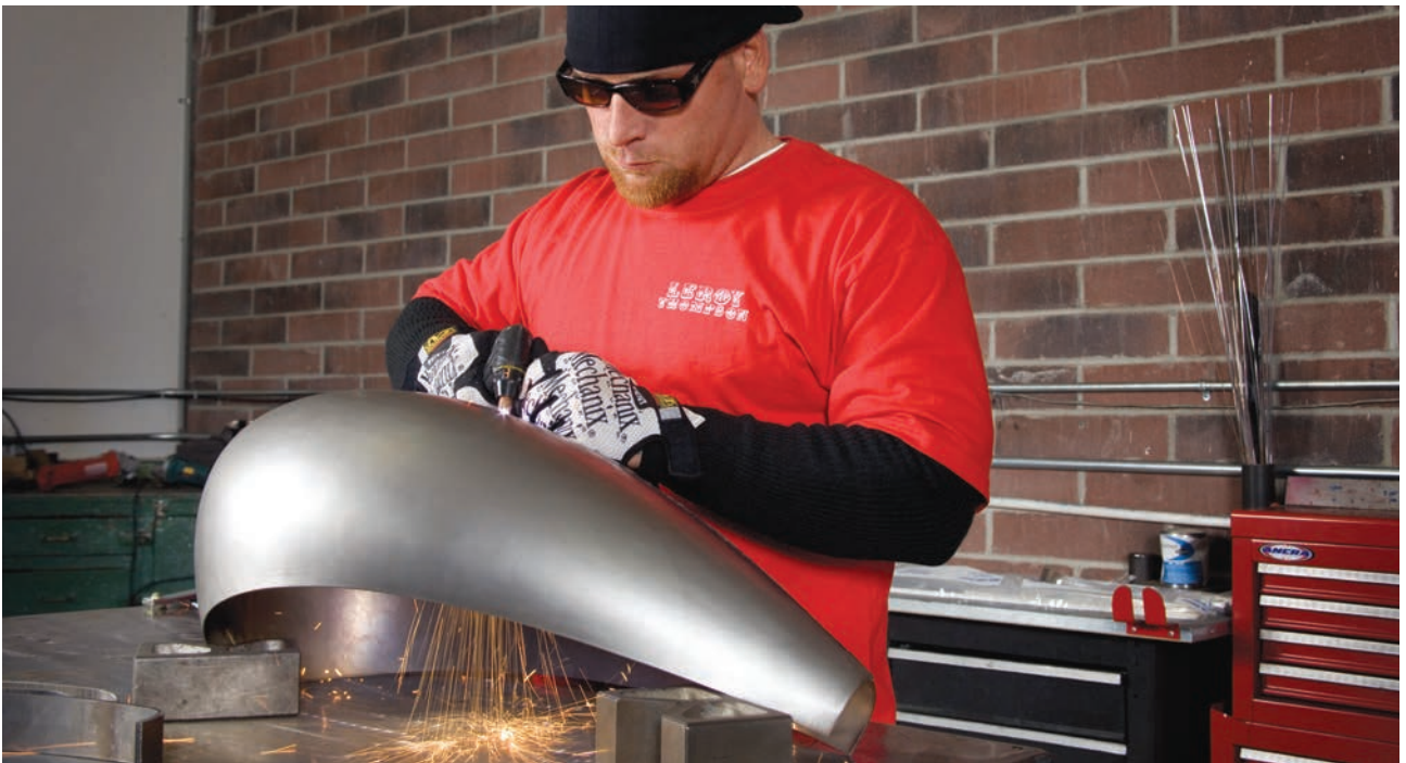
Here, custom motorcycle builder Scott Webster (of Leroy Thompson choppers) uses the Pro-Cut 55 to cut a piece of steel over a barrel that catches the debris.
