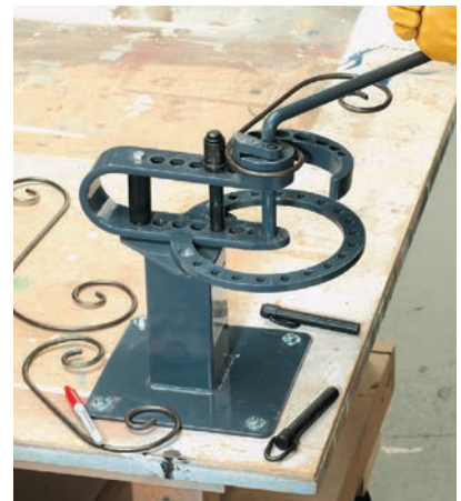
Use a scroll bender to bend decorative scrolls.
