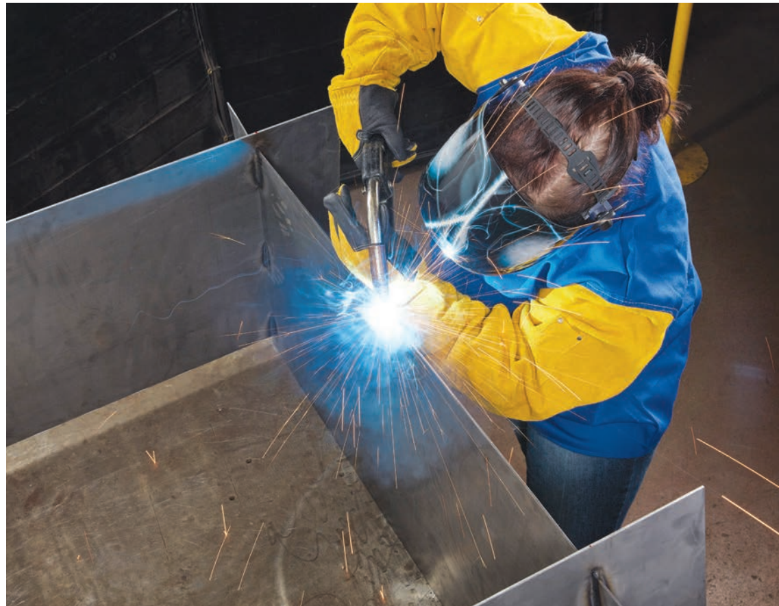
Place and weld the stiffener on its edge.
