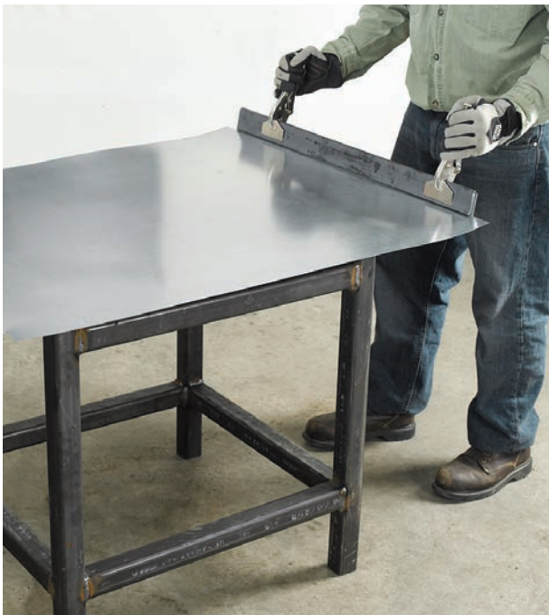
Use a strip of \frac{1}{8} "-thick steel as a bender. Clamp the bender to the tabletop sheet metal and bend up to 90°. Shown here: first make a bird's mouth cut on corners; bend those sides first so that the tabs are on the inside of the bend for a clean exterior edge.
