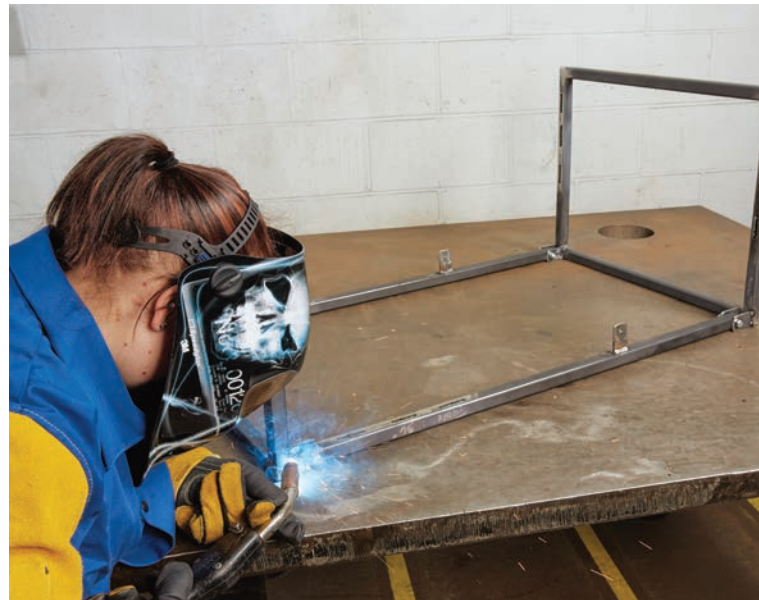
Tack weld the part E tabs in place.
