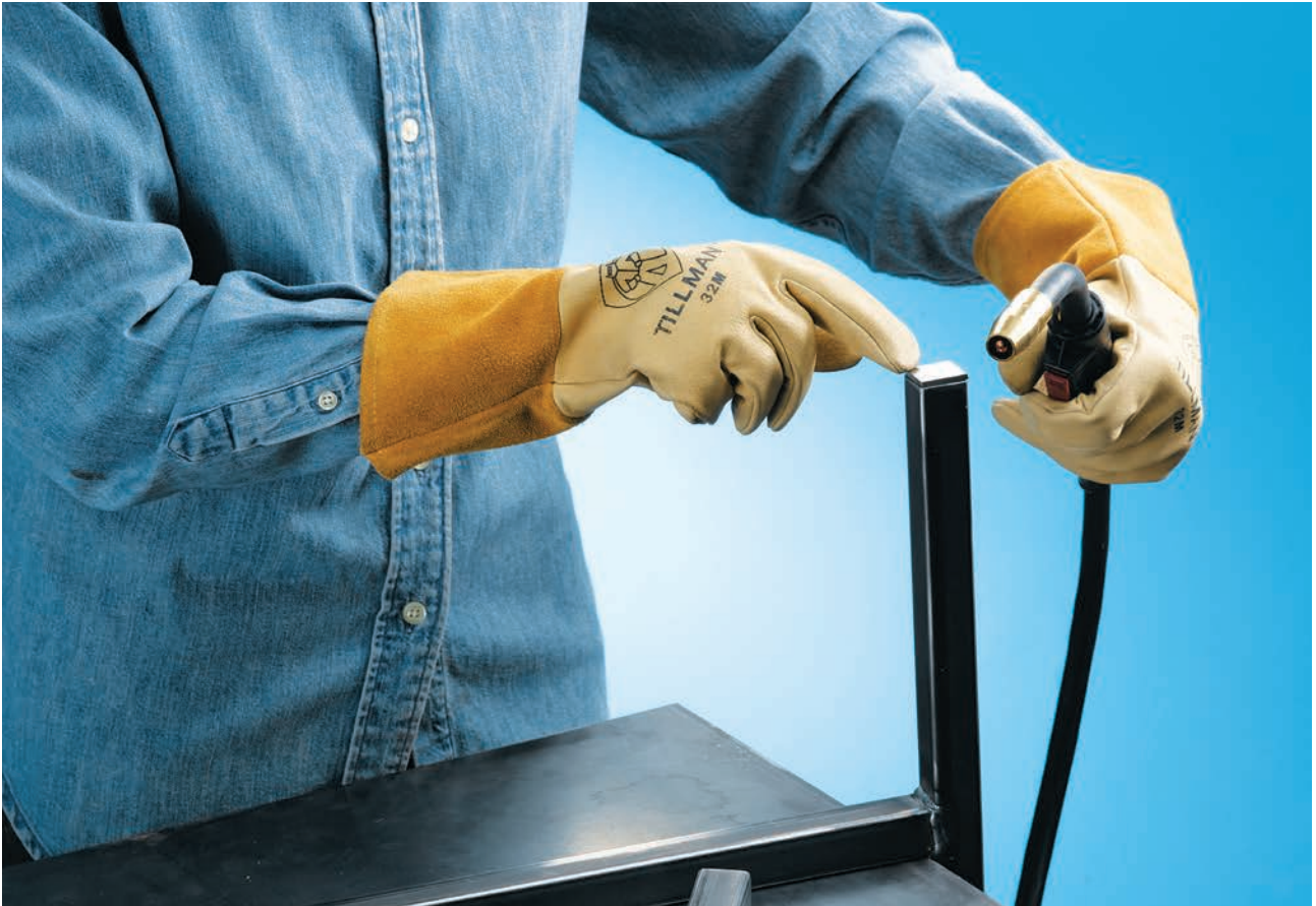
Tack weld the end caps in place, then weld and grind the welds smooth.
