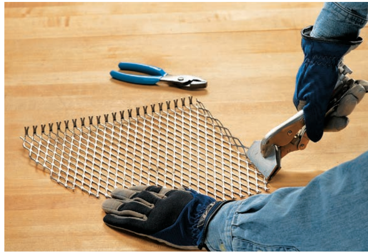
Use a hand seamer and pliers to bend the expanded sheet metal to fit inside the top and bottom crossbars.
