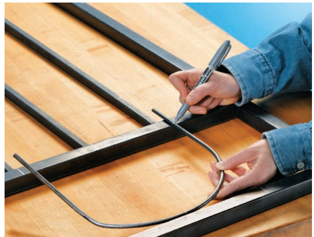
Align the top of the hoop with the top crossbar and mark where the legs cross the middle crossbar.
