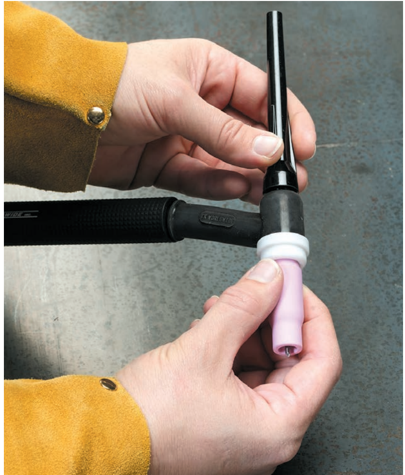
Tightening the back cap locks the tungsten electrode into place. The tip of the electrode should extend beyond the end of the cup by a distance of three times the electrode's diameter.
