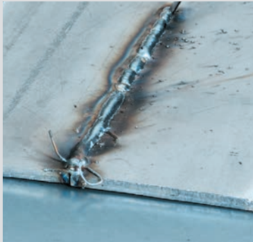
Stub out results in short sections of wire poking out of the weld.
