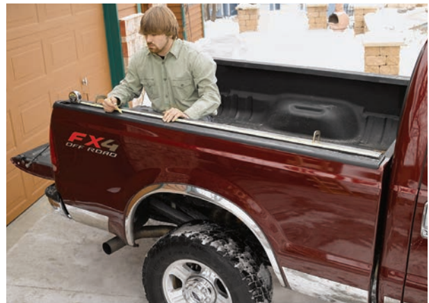
Measure in 6" from the tailgate ends of the angle iron, and make a mark for the tailgate uprights. Make a mark 2" in from the cab-side ends of the angle irons for cab-side uprights.
