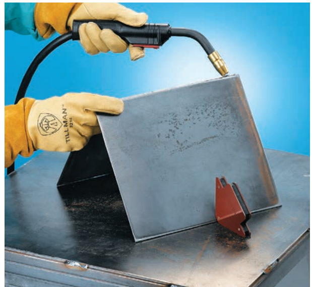
Form a V with rack sides and clamp with magnetic clamps. Weld the seam.
