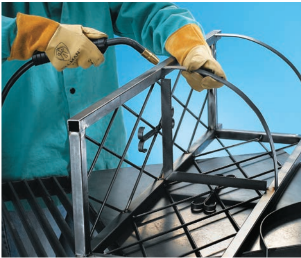
Weld the arched fronts to the sides, even with the crossbars.
