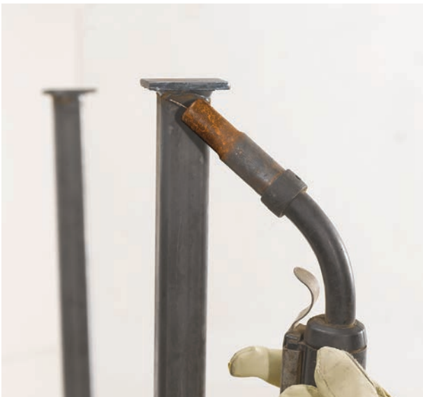
Flip the entire stand over and weld the leg feet (I) to the bottom side of the legs (A). If desired, casters could be added to the bottom for increased mobility. Be sure to pick casters that can lock.
