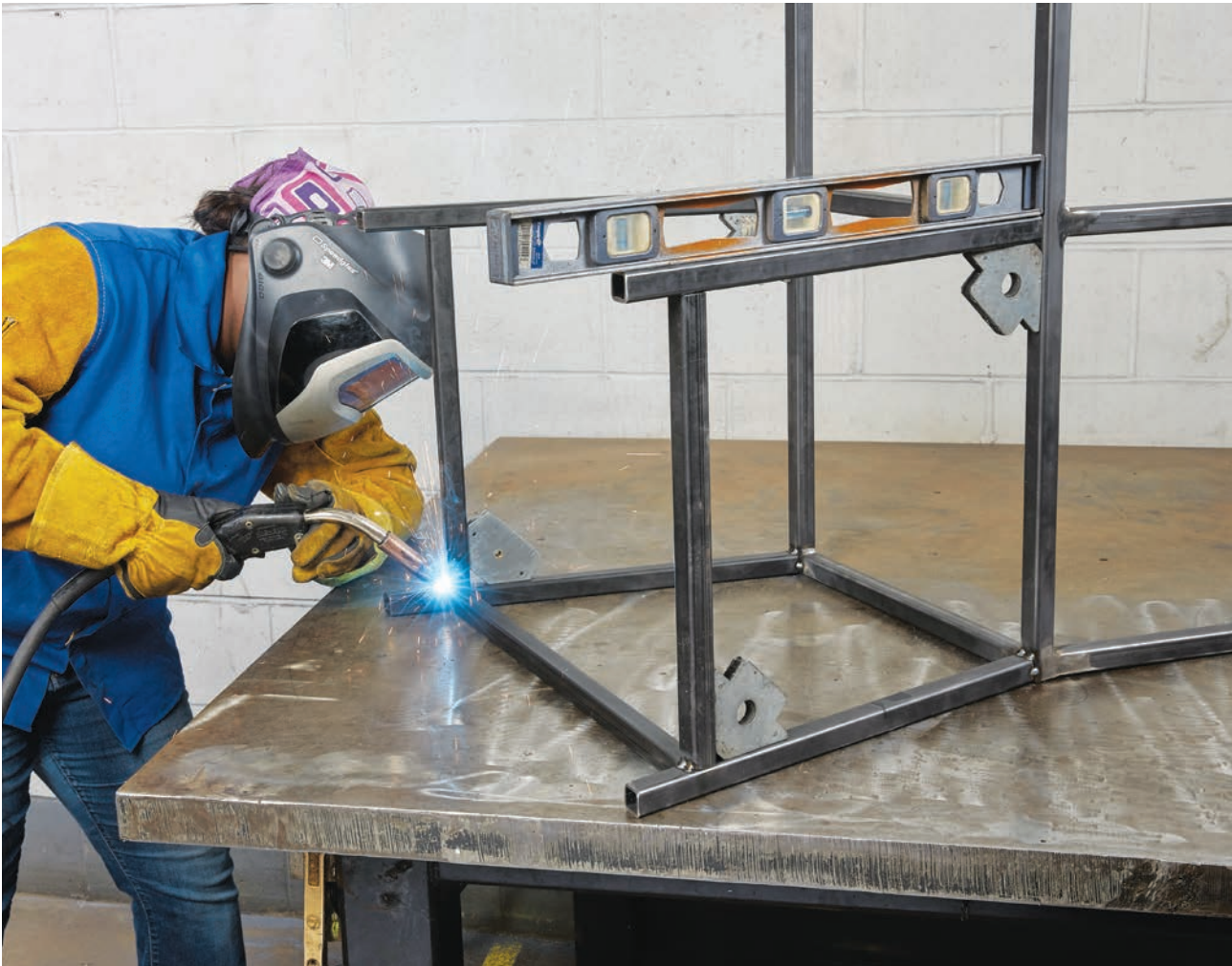
Tack weld brace F to brace D.
