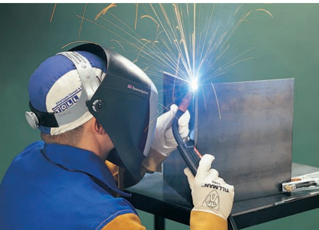
Gas metal arc welding (GMAW).
