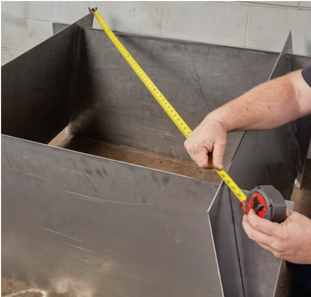
Measure diagonally to ensure you have a square.
