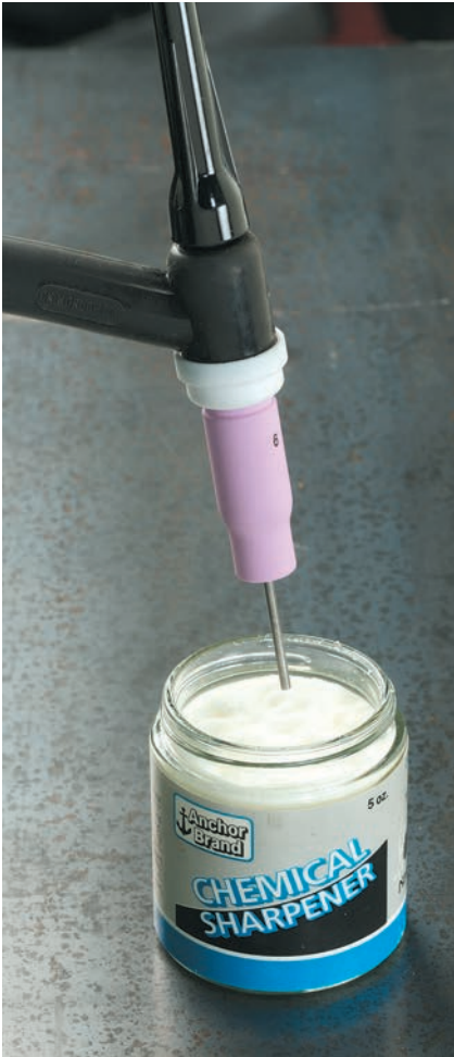
Chemical sharpeners are available for sharpening tungsten.
