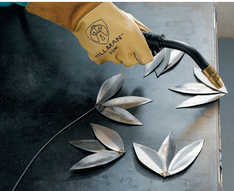
Arrange the leaves in sets of three. Weld the points together, then weld the stem to the leaf sets.
