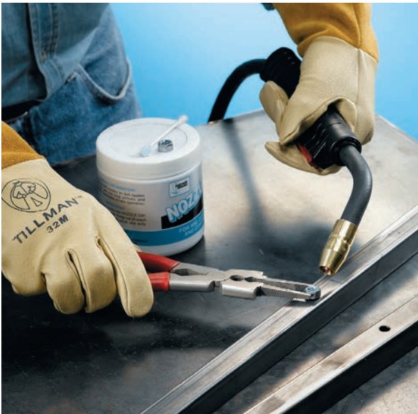
Weld the nuts over the holes in the frame sides before assembling the frame. Use anti-spatter gel to protect the nut threads.
