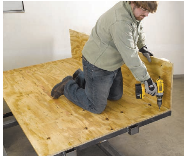
Drill the exterior-rated plywood sheet for flooring directly to the trailer frame.
