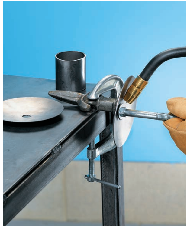
Create the finial assembly by welding the finial to the drip tray, then welding the bolt to the drip tray.
