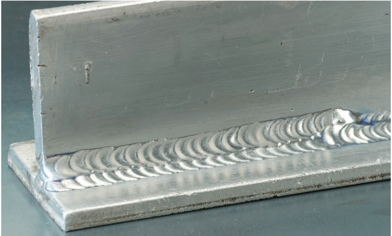
A well-done gas tungsten arc weld on aluminum has even ripples and good penetration. This sample weld shows two passes to create a fillet weld on \frac{1}{8} " stock.
