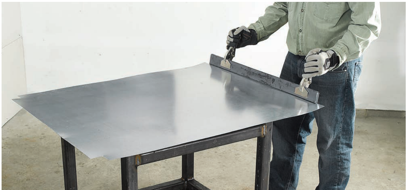
Use a flat bar and locking pliers to bend sheet metal.
