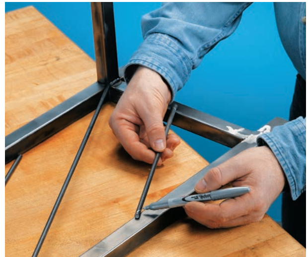
After cutting the diagonals to approximate length, mark the angles where the diagonal crosses the framework.
