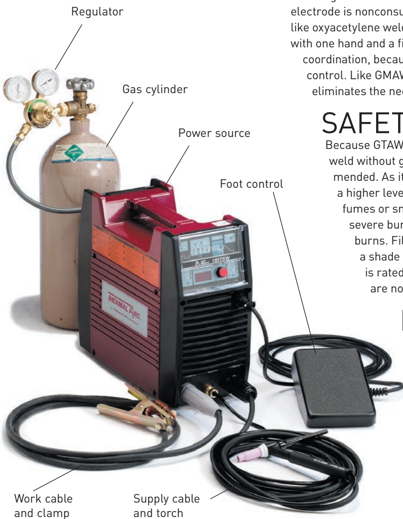
A gas tungsten arc welding setup.
