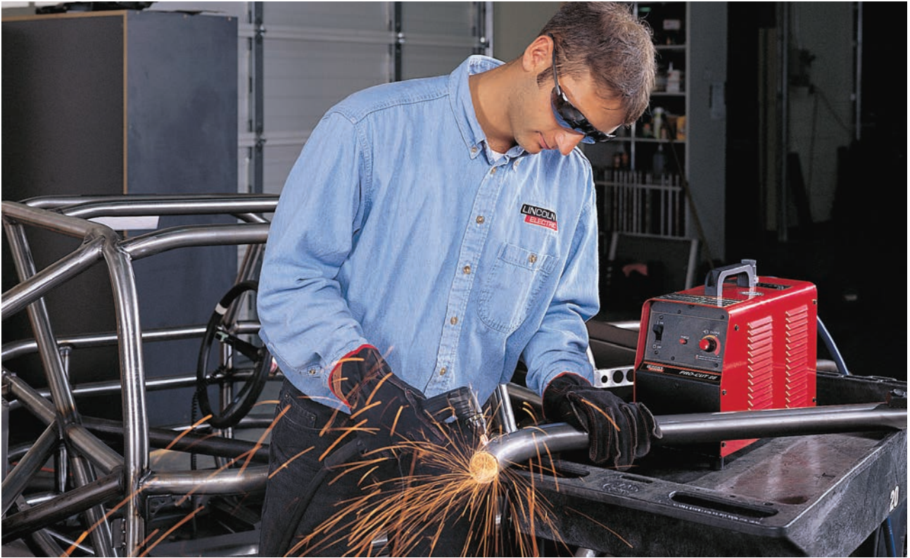
The Lincoln Pro-Cut 25 plasma cutting machine is good for fish-mouth fitting tubing, including tailpipe tubing. After the cut is made, a die grinder removes slag from the cut line.
