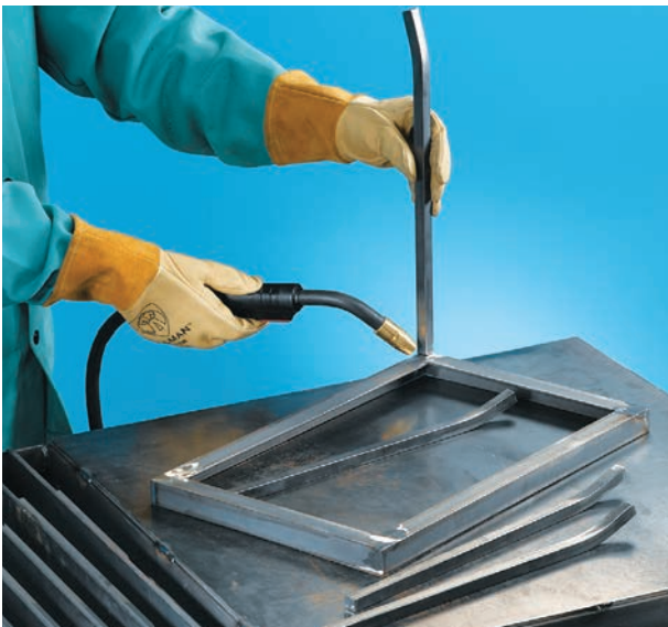
For a tiled tabletop, weld the legs to the flat underside so that the flanges form a cradle for the tile and backing material.
