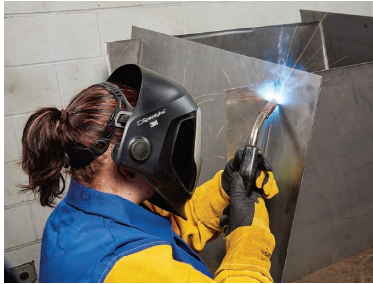
Tack all four corners, and then measure and stitch-weld the four seams.
