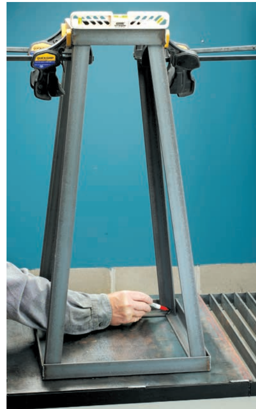
Assemble the grinder stand using clamps. Mark the top and bottom of each leg and cut to fit.
