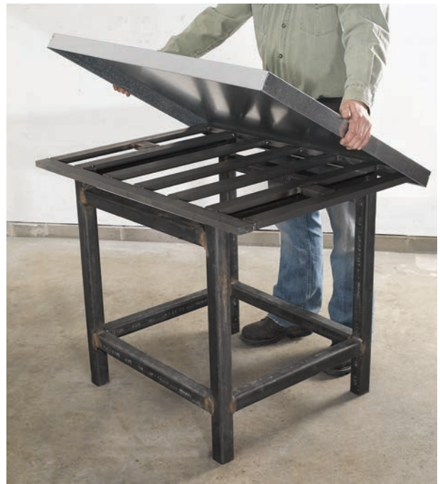
Lower the finished tabletop onto the table frame.
