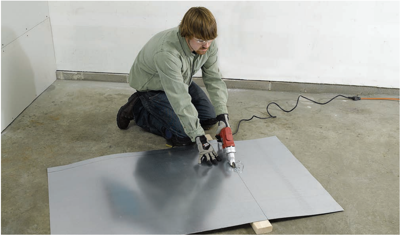
Cut the sheet metal top to 38 × 48 using a portable metal shears.
