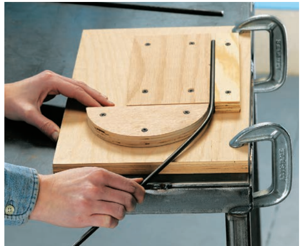
Make a bending jig to create the hoops for the decorative arches.
