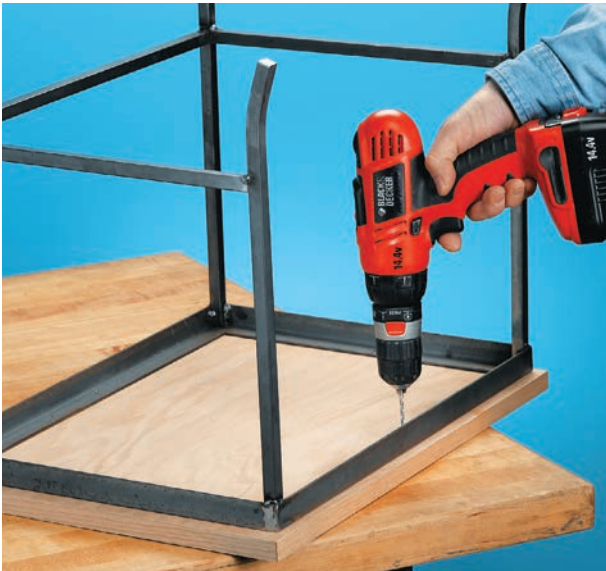
After drilling holes in each of the table's sides, align the wood top and drill pilot holes for the mounting screws.
