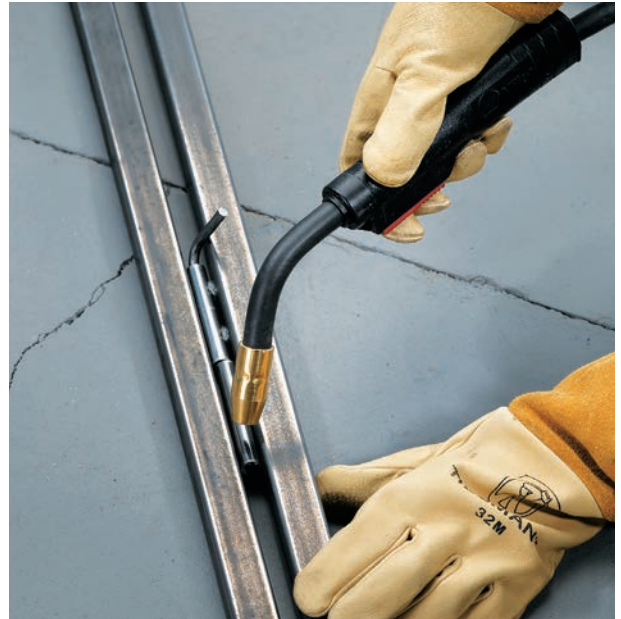
Insert a hinge pin into two hinge barrels. Place the hinge between two side panels, and weld one barrel to one panel and the other barrel to the adjoining panel.
