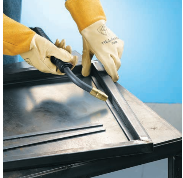
From the back, weld the inside frame to the frame. A small weld every 3" to 4" is sufficient.
