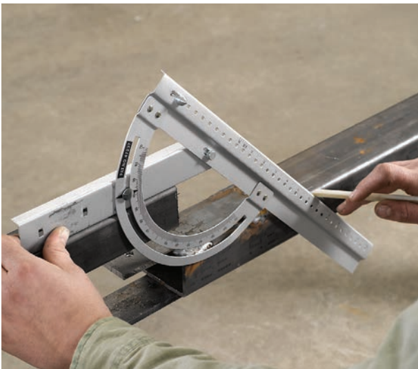
To determine the angle for the trailer tongue, align an angle finder on your truck or ATV hitch and on the trailer tongue. Mark this angle at the appropriate location on the tongue.
