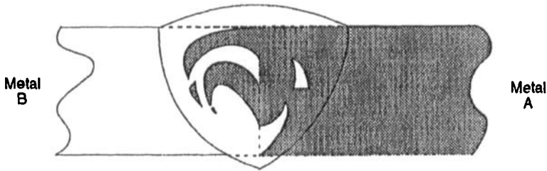
Figure 10.10 Schematic of macrosegregation in a weld pool, as affected by convection or its absence, when different base metals (A and B) are welded autogenously.
