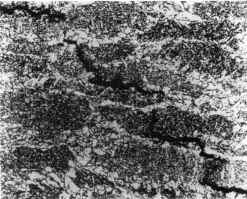
8.47 A chevron crack located in the recrystallized region of a weld metal (photograph courtesy of Cranfield Institute of Technology).
