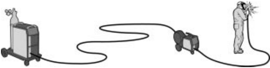
2.17 An intermediate wire feeder is useful at yards or other places where long reaching is essential (ESAB).
