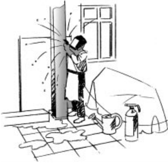
10.17 Risks are greatest in connection with temporary work in premises or areas not normally intended for welding.
