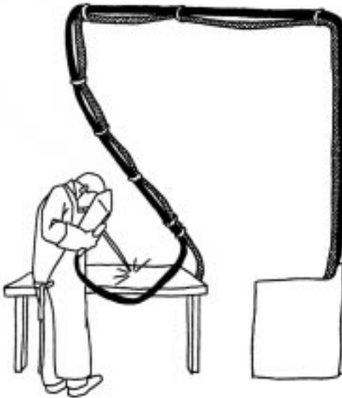
10.4 If the welding cable and return cable are kept close together their respective fields will cancel one another out.
