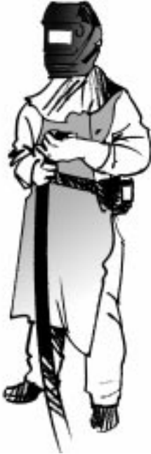
10.13 Protective clothing for thermal radiation and spatter.
