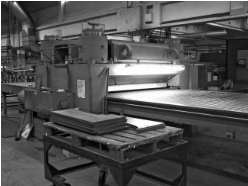
18.2 Straightening of steel plates.
