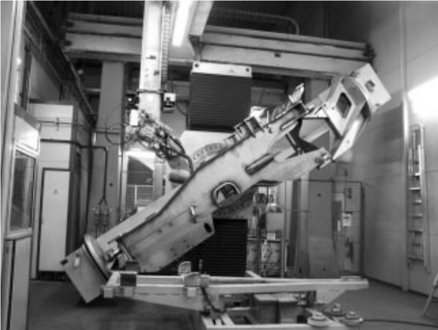
18.4 Gantry robot with tandem arc welding equipment.
