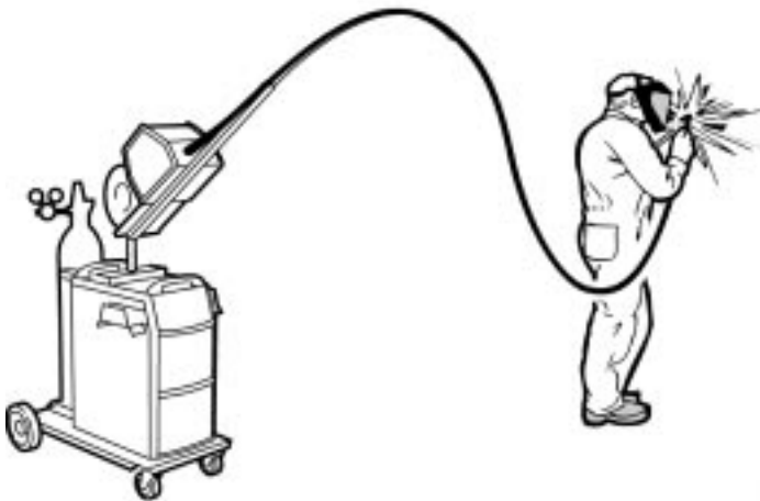
10.16 A counterbalance arm reduces the weight of the hose bundle over the entire working area.
