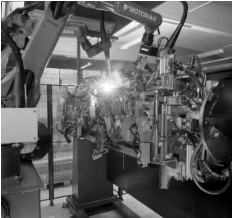
16.5 Cooperation between two robots and one positioner.
