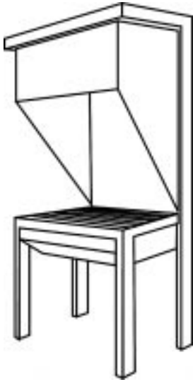
10.10 A welding bench with fume extraction.
