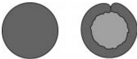
1.15 Cross-section of solid and cored wire.
