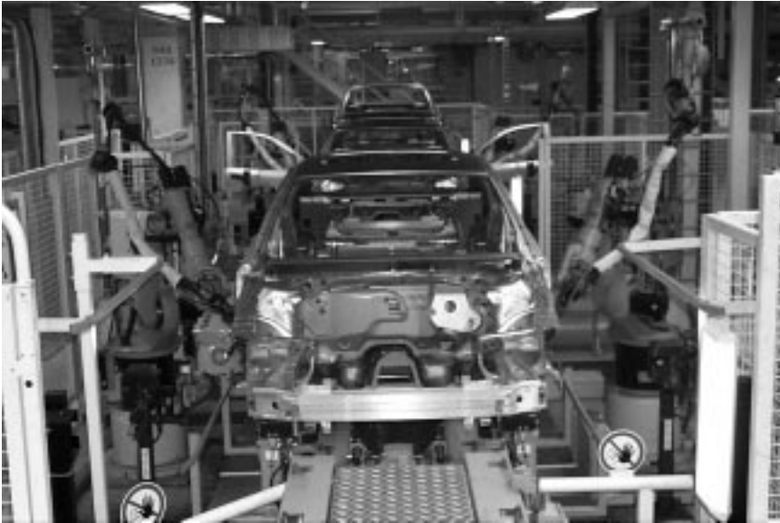
17.5 Robot station in the complete-body assembly line.
