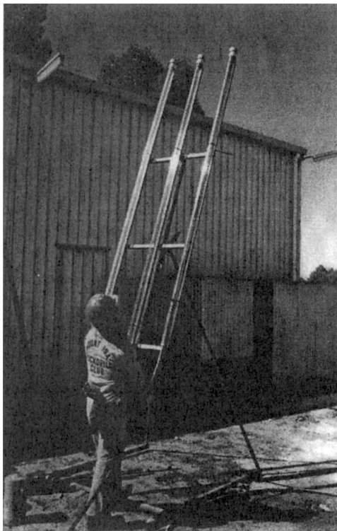
Figure 5. Experimental set-up used to grout transparent pipes.
