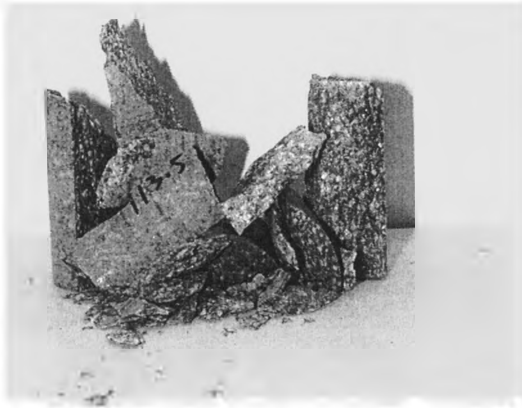
Figure 16. Unsprayed porphyry core tests.
