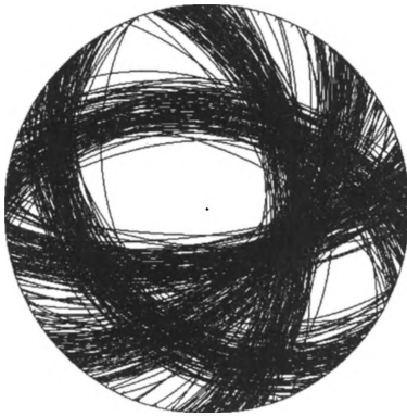
Figure 6. The arcs of great circles of the planes corresponding to the 500 simulated normals.
