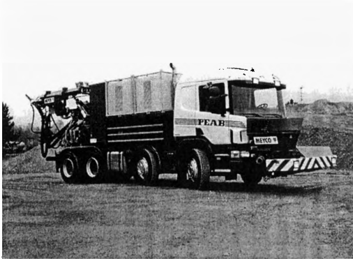
Figure 6: MEYCO® Roadrunner: This mobile spraying system contains all specified equipment of a spraying mobile, mounted on a roadworthy truck. All equipment can be powered either from an external source or by its own Diesel motor.
