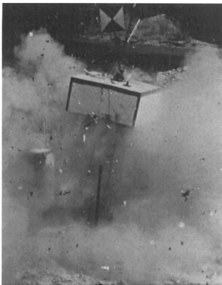
Figure 2. Failure of support in an impulse load test
