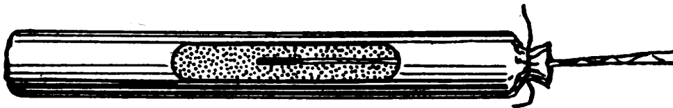
Fig. 10.—Tamping bag or cartridge filled with blasting powder and primed with an Electric Squib.
