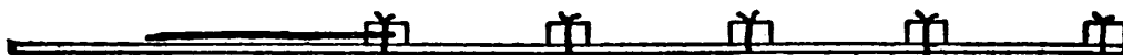
Fig. 100.—The size of each cartridge and distance apart on the stick are changed to suit the condition of the ground.
