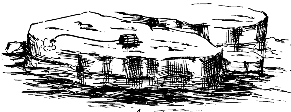
Fig. 109. —Showing bundle of cartridges tied together with fuse and cap, used to mudcap floating pieces of ice.
