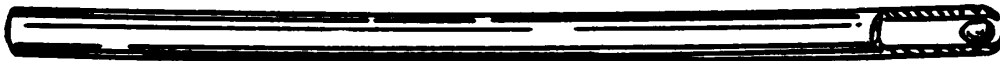
Fig. 81.—Another type of spoon, which is a modification of the pump for shallow bore holes.
