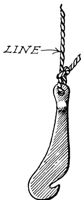
Fig. 139.—Special hook for bail of nitroglycerin container.
