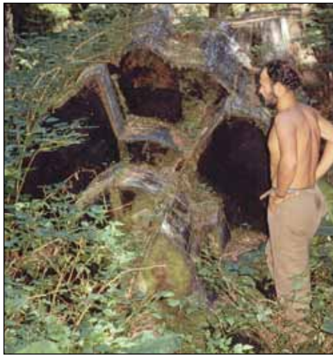
FIGURE 7 A fragment of a log cut 80 years ago in the Malcolm Knapp Research Forest showing negligible decay.
