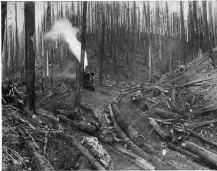
FIG. 34.—SKIDDING LOGS BY STEAM DONKEY ENGINE IN NORTHERN IDAHO.
