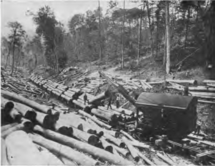
FIG. 31. — A STEAM LOG LOADER IN ACTION.
