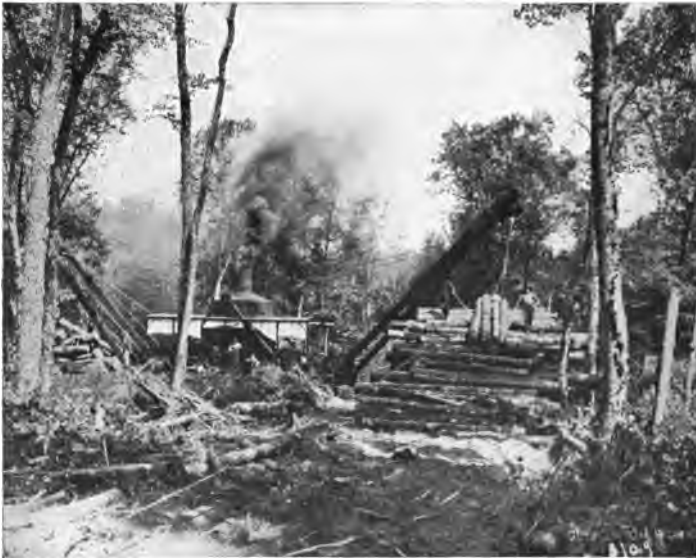
FIG. 33.— SKIDDING LOGS BY STEAM IN NORTHERN HARDWOOD FOREST.
