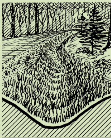
U-shaped, grass stabilized ditch
