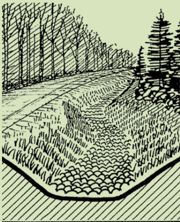
Grass and stone stabilized ditch
