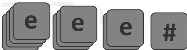
Figure 2.1 The stack of a PDA. As an element is read from the top, the next element appears as the new top if nothing is written to the stack.
