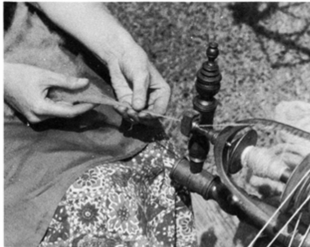
The right hand draws the fiber as the left hand regulates the amount of twist.
