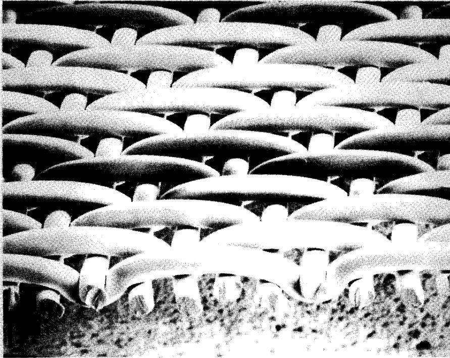
FIGURE 12.11 Five harness single layer forming fabric (courtesy of Asten Forming Fabrics, Inc.).
