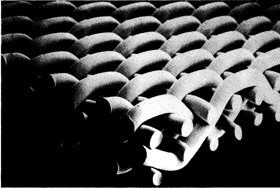
FIGURE 12.13 Photomicrograph of a standard two layer fabric (courtesy of Asten Forming Fabrics, Inc.).
