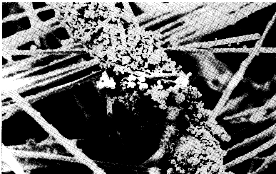
FIGURE 8.12 Electromicroscopic photograph of Tefaire® nonwoven filter fabric (courtesy of DuPont).
