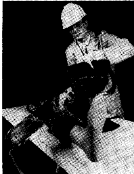
FIGURE 13.18 Chain saw chaps provide effective cut and slash protection (courtesy of DuPont).
