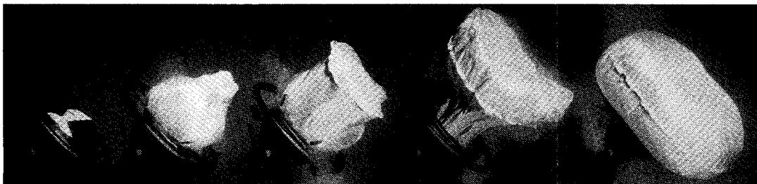
FIGURE 15.6 Deployment of an airbag (courtesy of Sulzer Ruti).
