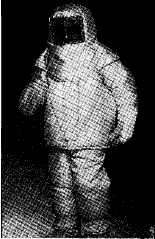
FIGURE 13.11 Fire entry suit. This suit is designed for short duration entry into total flame engulfment or furnace. It consists of separate coat and pants constructed from multiple layers of glass insulation, aluminized glass, and non-aluminized glass surface (courtesy of Fyrepel Products).
