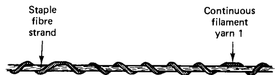
Figure 14.4 first-stage selfil yarn
