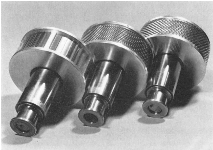
Plate 26. Interchangeable opening rollers for rotor spinning machine. The 80 mm diameter opening rollers, which can rotate at speeds from 3000 to 9000 rev/min, can be changed easily and quickly by releasing a clamp. Viewed from left
