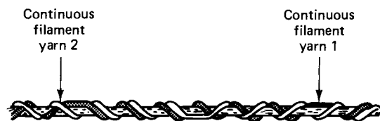
Figure 14.5 Final selfil yarn
