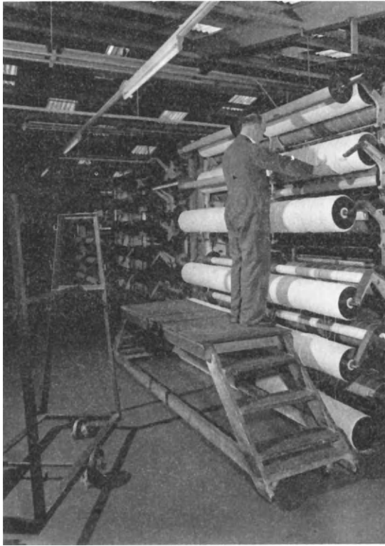
Plate 6. Six-tier twelve-drum tape condenser. The full condenser bobbins of the four lower tiers have been doffed and replaced by empty condenser bobbins which can be seen resting against the surface drums which drive them. The right-hand condenser bobbin next to the top is about to be doffed. This condenser is 2.5 m wide and delivers 144 slubbings from the 1.5 m working width card which is feeding it. Production rates vary widely according to the type of material and the slubbing count delivered. For example, when producing slubbings of 50 to 125 tex from 100% Shetland or a blend with man-made fibre, the output would be from 10 to 50 kg/h. Courtesy of Haigh-Chadwick Ltd
