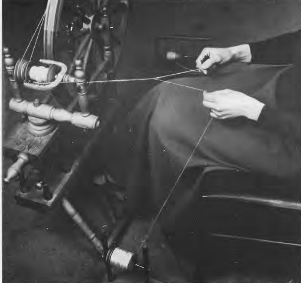
96 Plying, with independent control on the tension of a yarn
