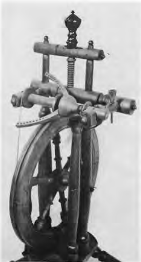
27 Detail of a German spinning wheel showing a flyer drag with friction band across the hollow shaft and the flyer with holes instead of hooks.
