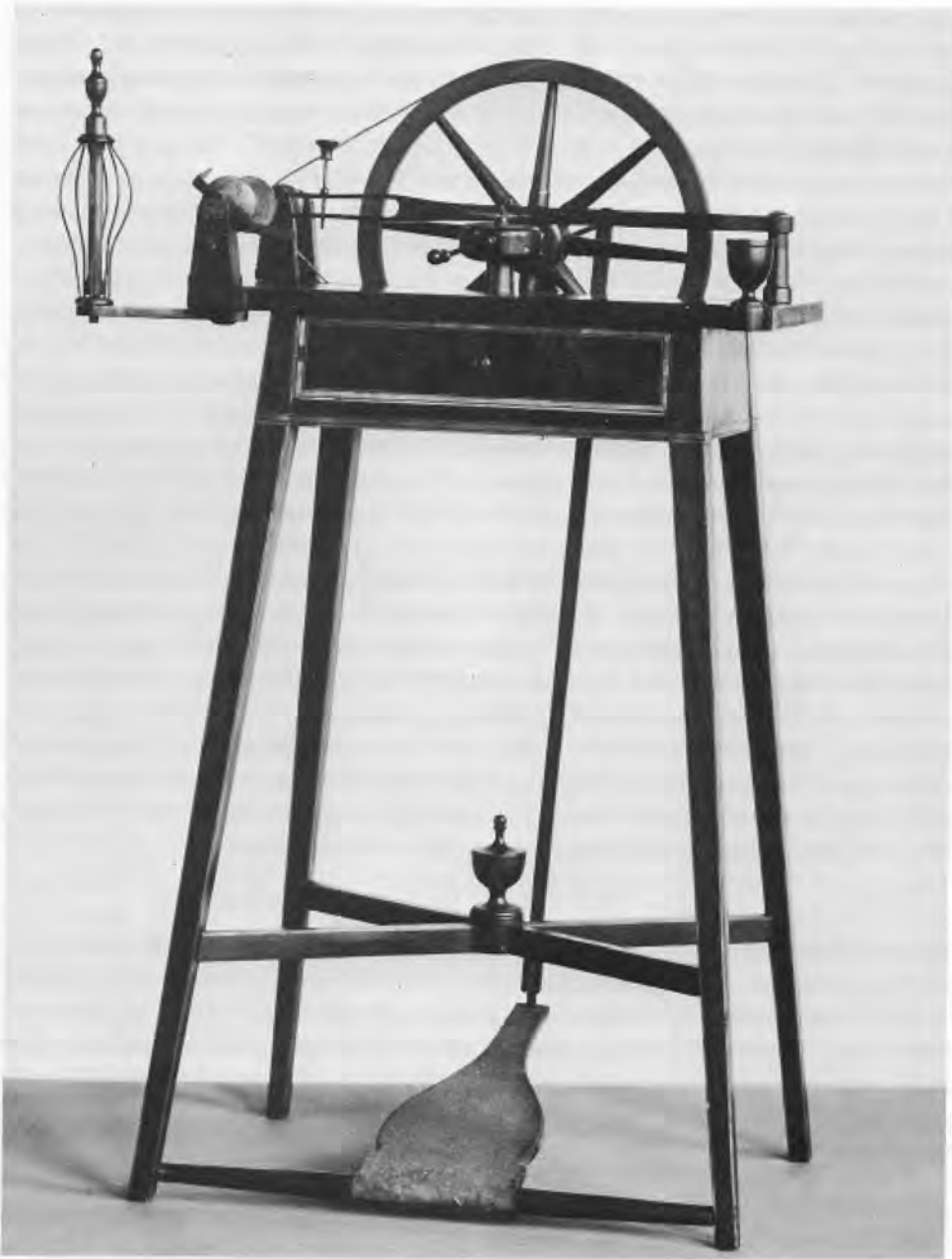
68 Mahogany spinning wheel in the Sheraton style made by John Planta of Fulneck near Leeds, c.1800. Wheel diameter 11\frac{1}{4} in. (28.5cm.). Now in the Science Museum, London.
