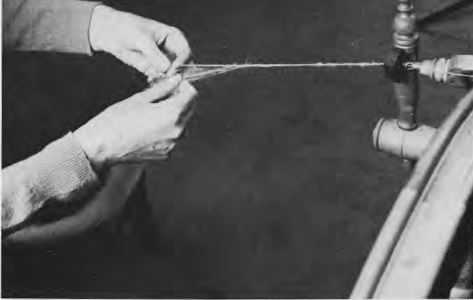
80 Woollen spinning (a), joining
