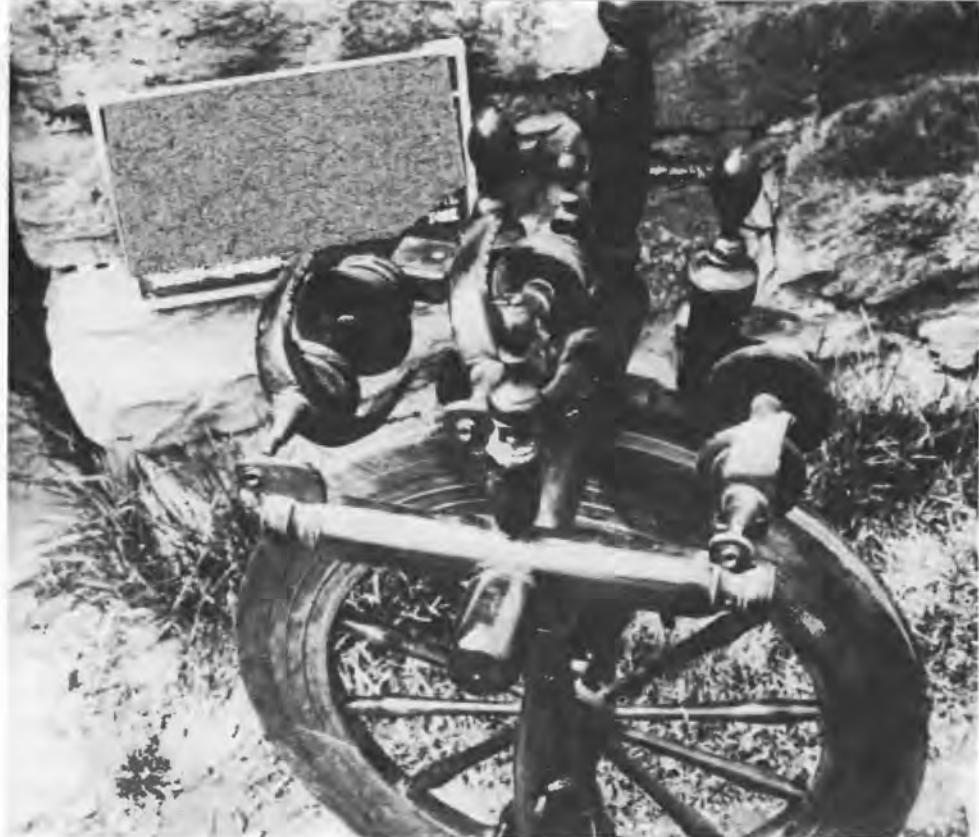
62 Scottish vertical spinning wheel with three flyers.
