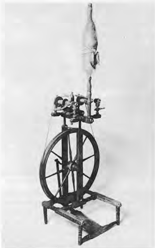
61 Nineteenth-century double flyer vertical spinning wheel from South Germany. Photograph: Deutsches Museum, Munich
