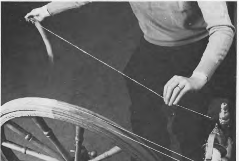
83 Woollen spinning; fibres fully attenuated
