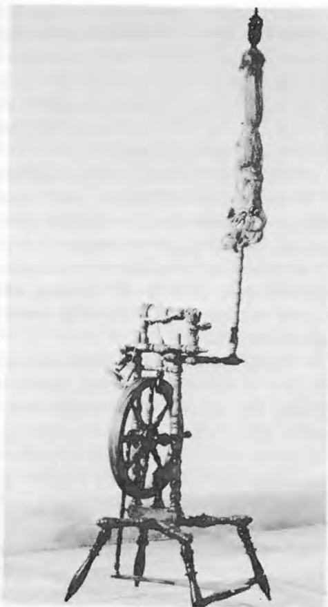
51 Vertical spinning wheel from the Tyrol with an X-shaped base, and flyer drag. Wheel diameter 12\frac{1}{2} in. (31.5cm.).
