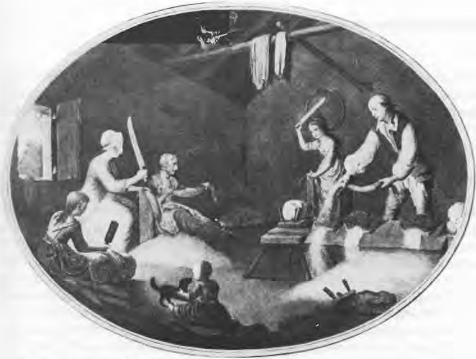
4 After plate IV (1791) of a series of 12 engravings illustrating the processes in the eighteenth-century Northern Ireland linen industry, by William Hincks. It shows beetling or flax breaking with a mallet, scutching and hackling
