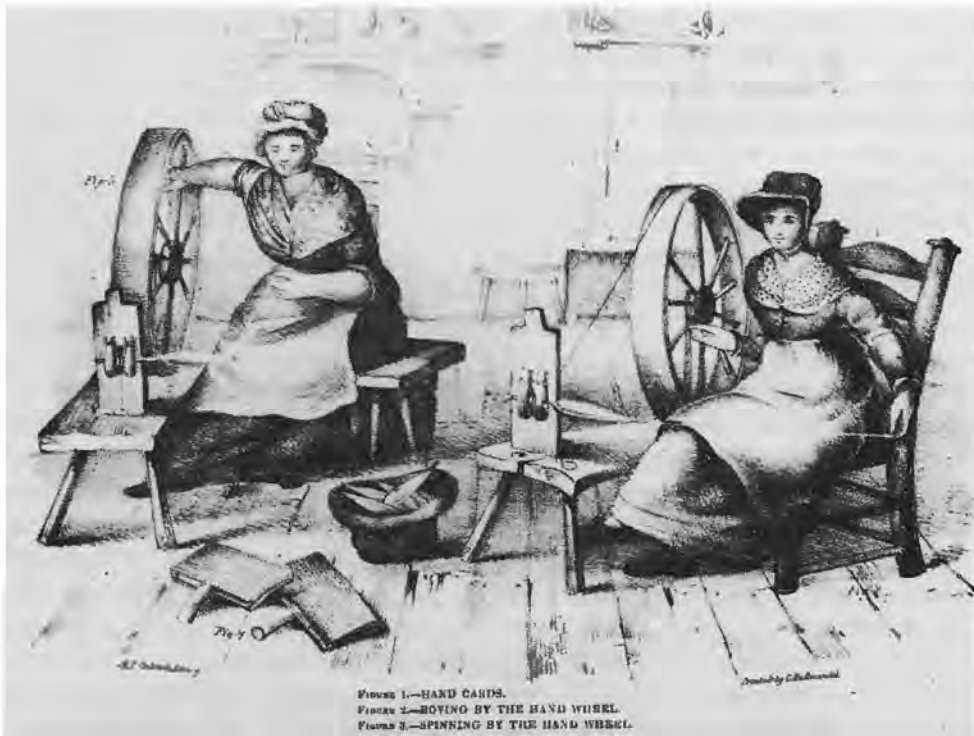
72 Plate 3 from R. Guest's A Compendious History of the Cotton Manufacture , 1823. Two cotton workers (left, spinner; right, rover).
