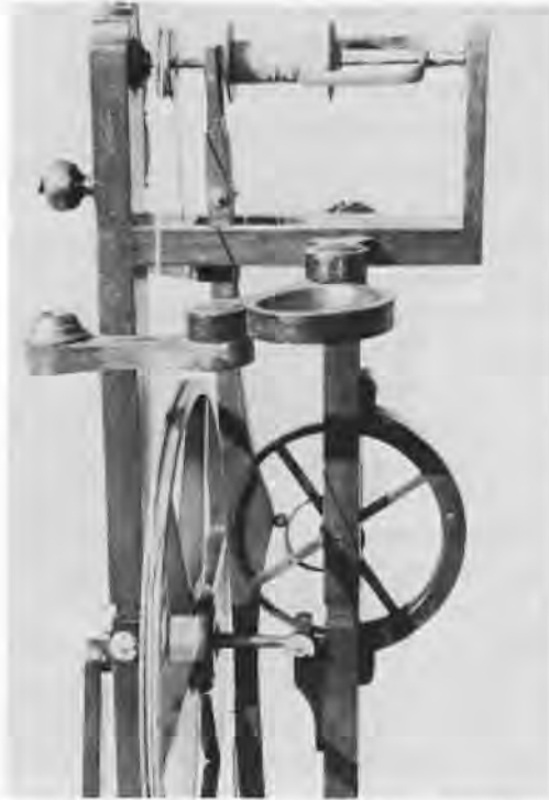
67 Detail of spinning wheel by Doughty of York, c.1795–1800. Made of mahogany with brass wheel, diameter 12in. (30·5cm.). It shows the mechanism for automatically winding the yarn evenly on to the bobbin. Photograph: Castle Museum, York
