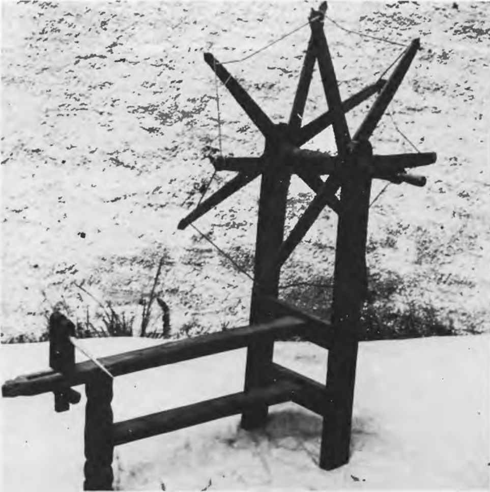
13 A European rimless spindle wheel from Hinterrhein, Canton Graubünden, Switzerland. Wheel diameter approximately 28in. (71cm.). Photograph: Dicziunari Rumantsch Grischun
