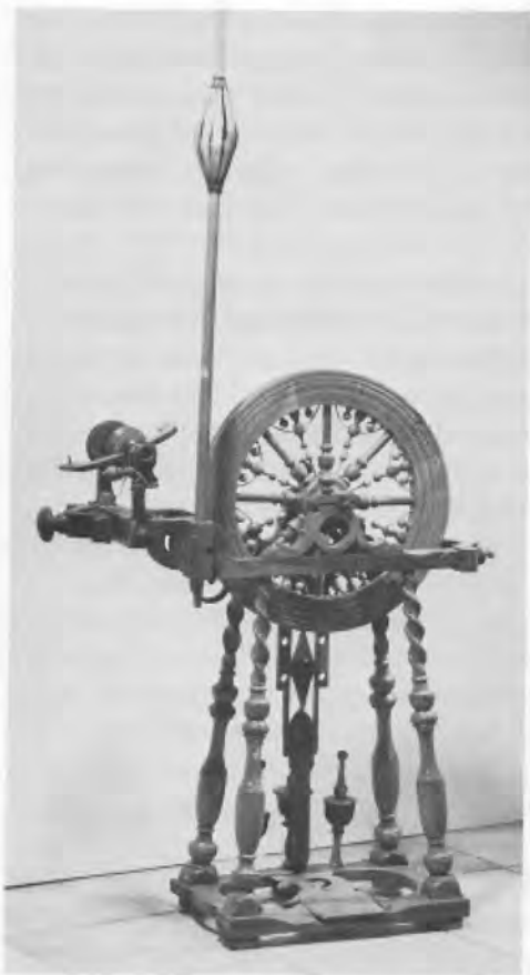
50 Horizontal spinning wheel with frame and lozenge-shaped distaff from the Tyrol. Wheel diameter 14\frac{1}{2} in. (37cm.).
