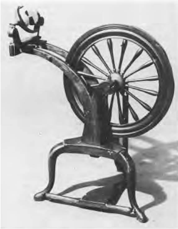
53 A spinning wheel from north-east Scotland with boomerang supports. Wheel diameter 15½ in. (39.5 cm.).
