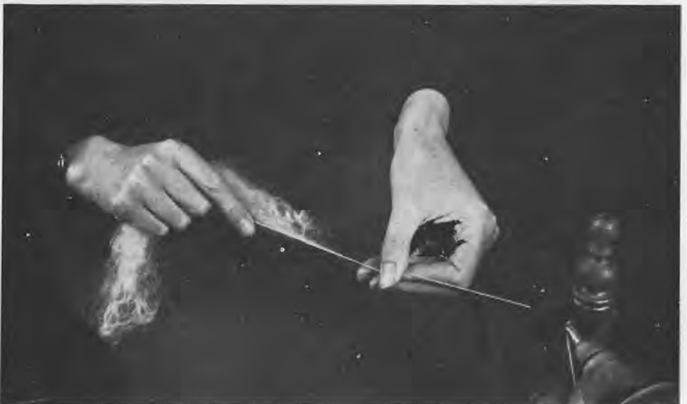
86 Worsted spinning (d), smoothing fibre-ends into the twist
