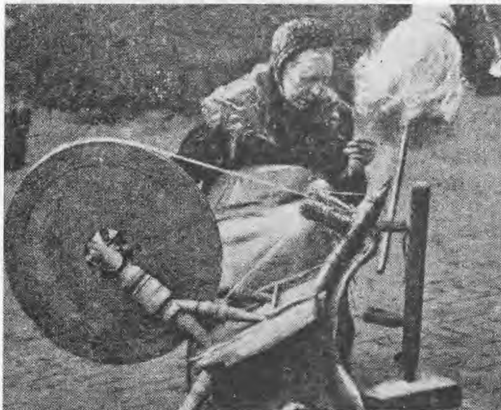
42 An old lady from the Courtrai district of Belgium spinning flax using a hand-turned disc wheel. After an old photograph
