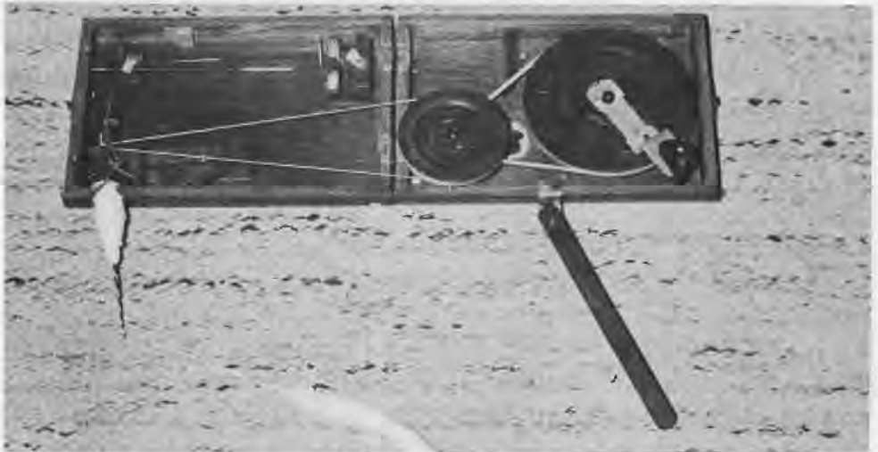
23 A modern Charka made in India on lines specified by Gandhi. The spindle folds away when the box is closed; larger wheel diameter
