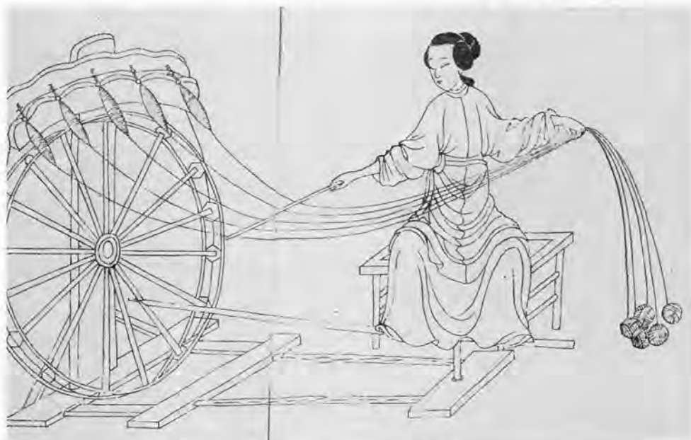
12 Illustration from Nung-cheng ch'üan-shu , 1562–1633 (Ser.d. 107/15 f.13a & b). Chinese multi-spindle spindle wheel with universal joint type of treadle being used for spinning from balls of rovings. Photograph: Curators of the Bodleian Library, Oxford
