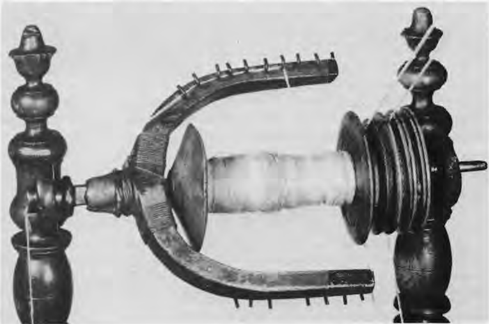
26 Detail of the flyer mechanism showing a bobbin lead, doubled band drive.
