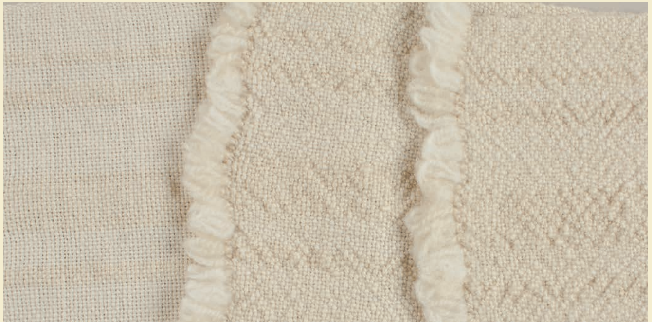
MERINO/BLUEFACED LEICESTER WARP WITH BLUEFACED LEICESTER WEFT. Left to right: unwashed; 15% shrinkage after five minutes of agitation; 16% after fifteen minutes.
