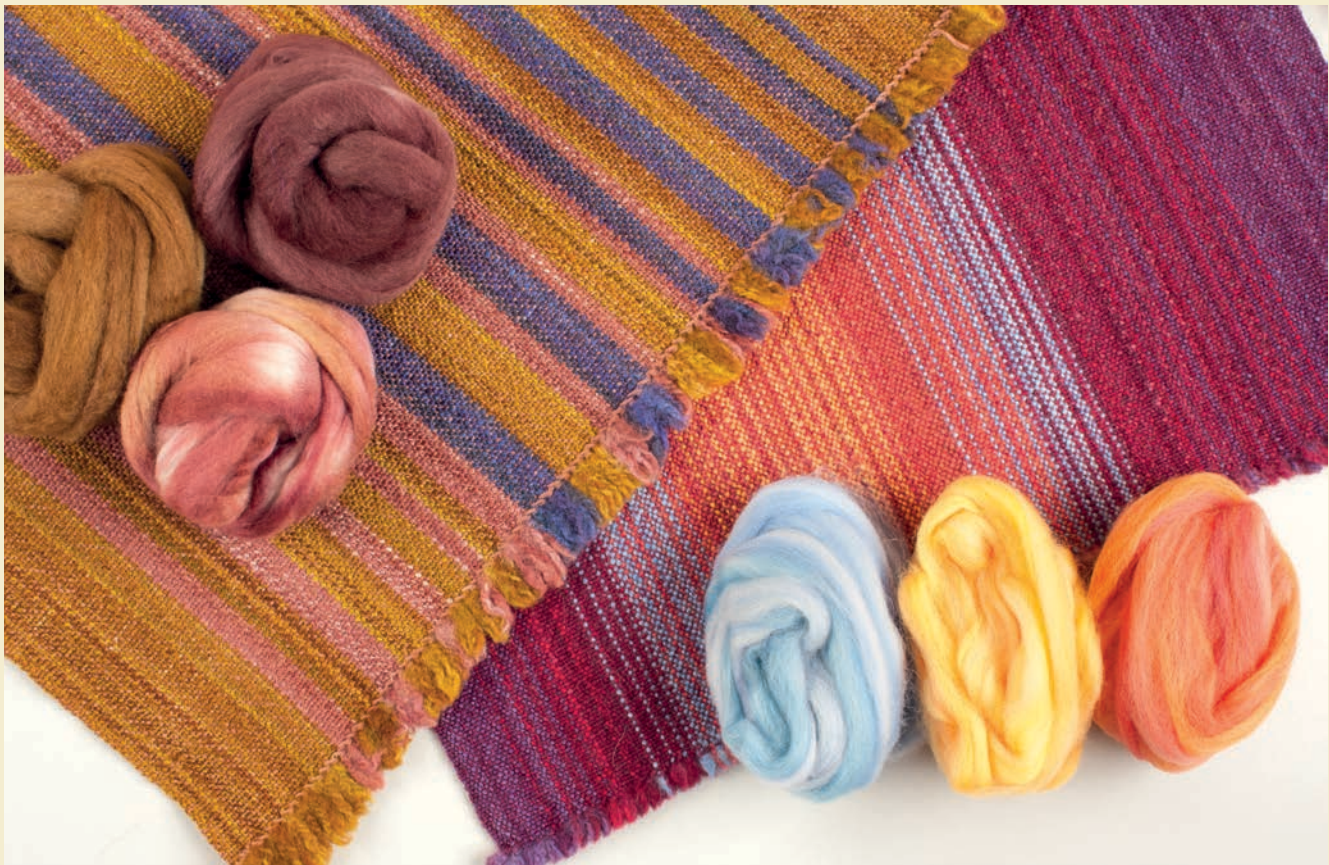
Fabric from wool spun from top (left) has a smooth surface; fabric from wool spun from roving (right) has a fuzzier surface.
