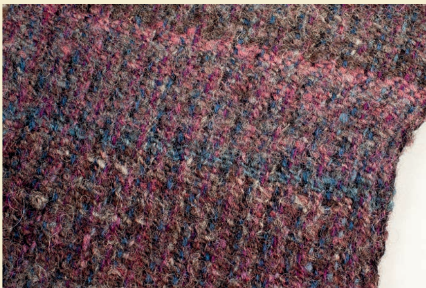
Varying amounts of twist in the weft yarns caused puckers in this wool fabric.
