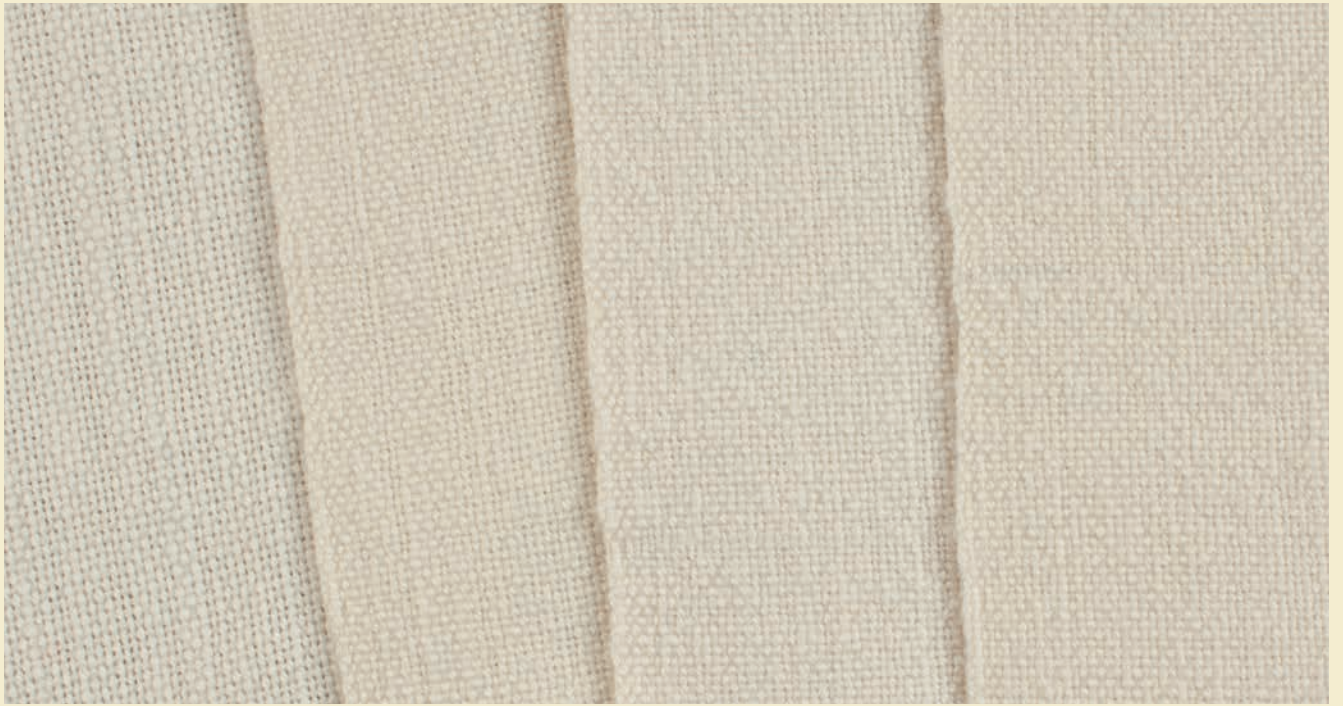
SUPERWASH MERINO. Left to right: unwashed; 10% lengthwise shrinkage after five minutes of agitation; 10% after ten minutes; 10% after fifteen minutes.
