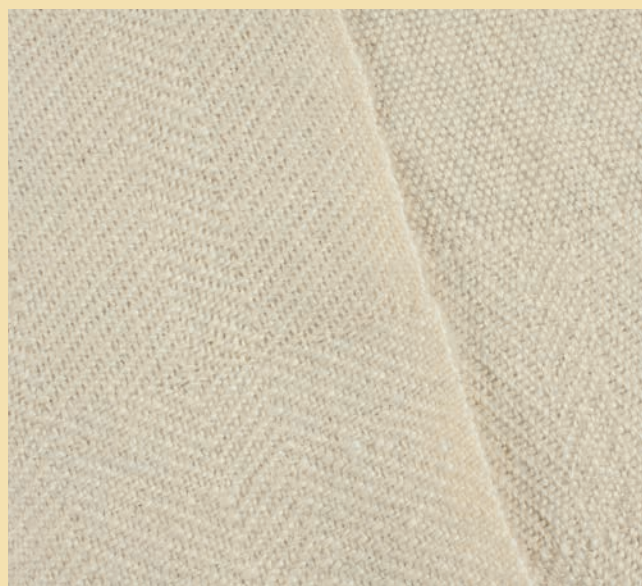
Twist direction warp stripes: 15 epi (left) and 12 epi (right).
