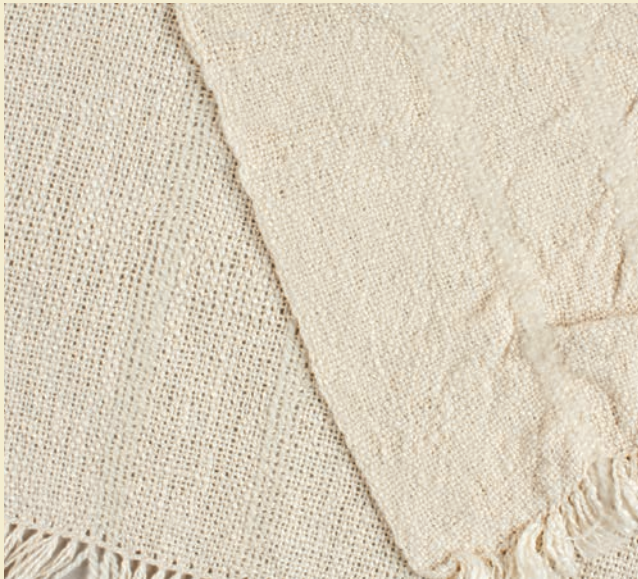
Grouped warp ends of Merino and silk will also create puckers as the wool shrinks with washing. Samples spun and woven by Amy Norris.
