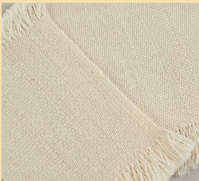
Tightly twisted Romney sett at 40 epi (left) and 30 epi (right).
