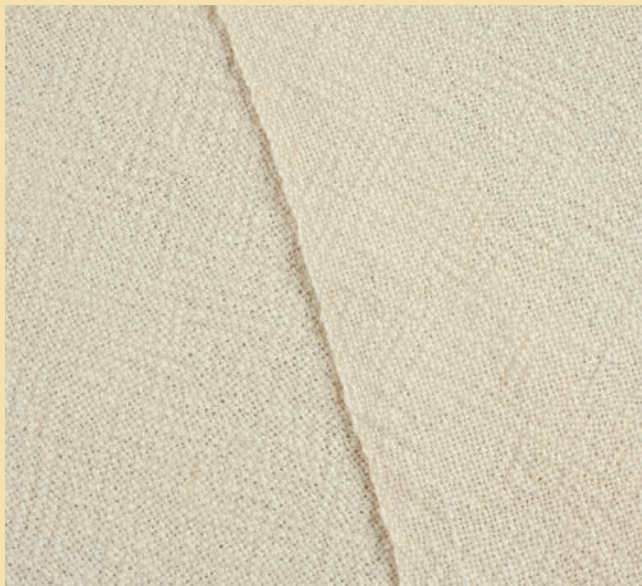
Romney plain weave z2s warp sett at 15 epi: z2s weft (left) and s2z weft (right).
