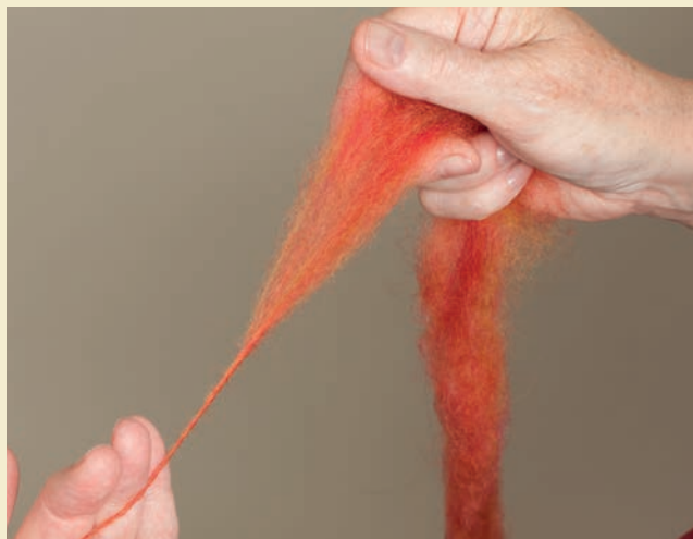
Fibers enter the twist zone in less alignment when spinning from roving.
