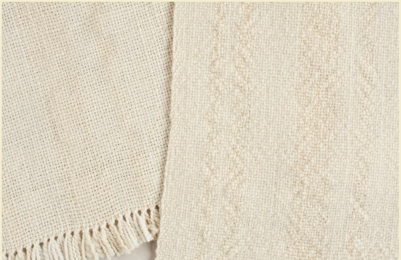
Different fibers behave differently in the same fabric, as illustrated by the Merino and Bluefaced Leicester stripes in the warp of these samples (left: unwashed; right: washed).
