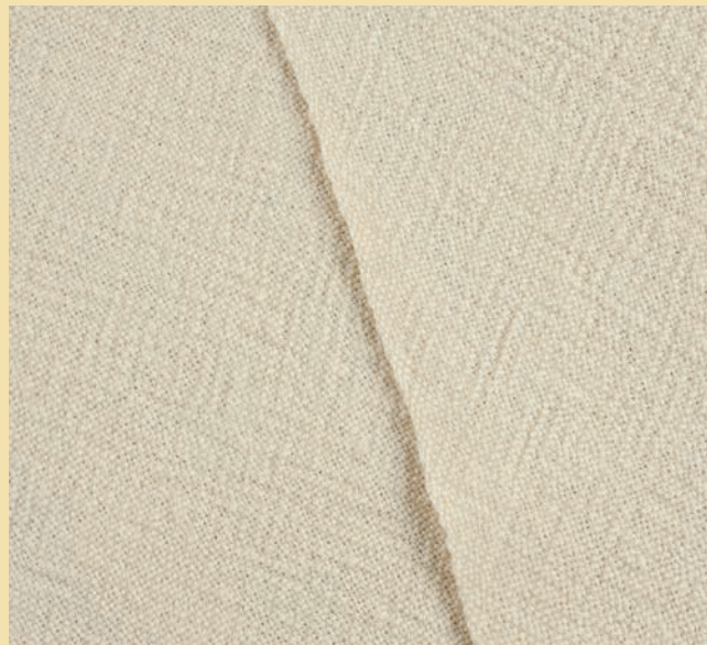
Romney plain weave z2s warp sett at 20 epi: z2s weft (left) and s2z weft (right).
