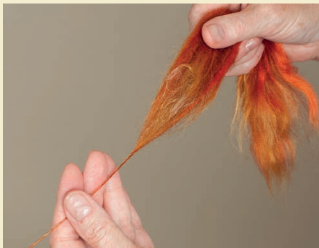
Fibers enter the twist zone in relative alignment when spinning from prepared top.
