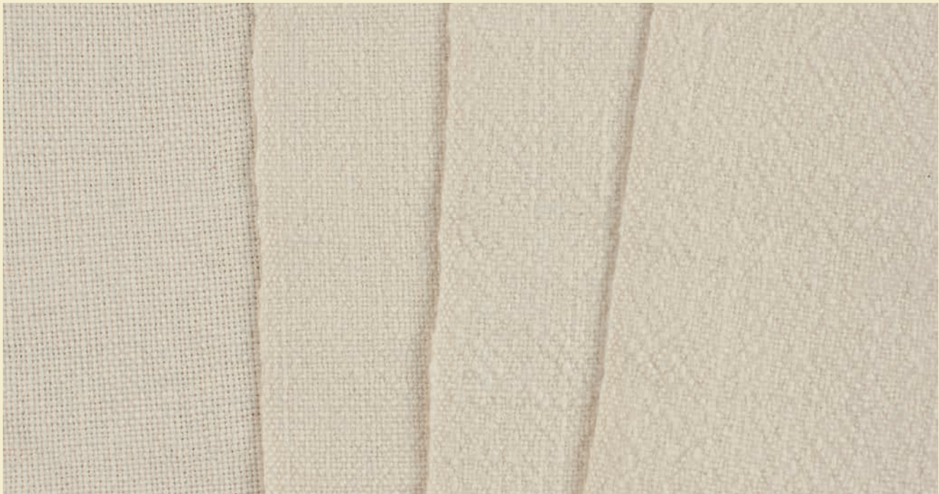
MERINO. Left to right: unwashed; 11% lengthwise shrinkage after five minutes of agitation; 13% after ten minutes; 14% after fifteen minutes.
