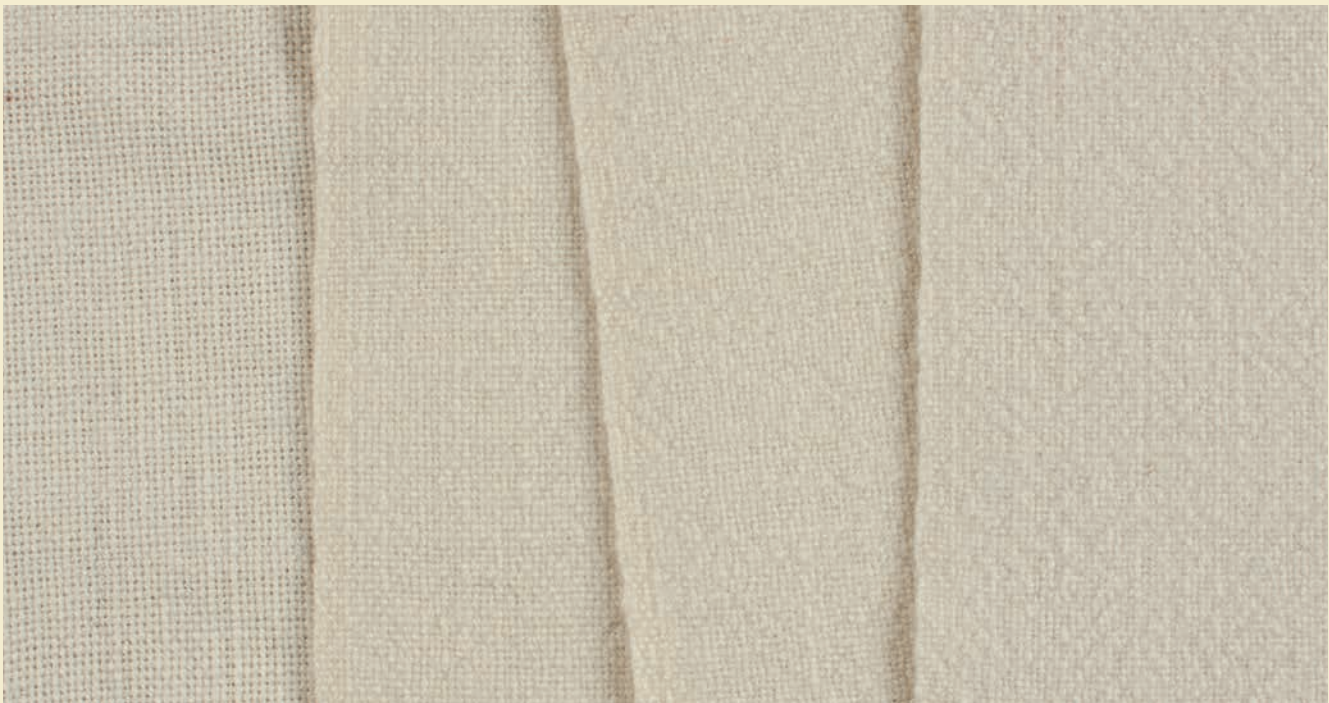
CORMO. Left to right: unwashed; 13% lengthwise shrinkage after five minutes of agitation; 13% after ten minutes; 13% after fifteen minutes.
