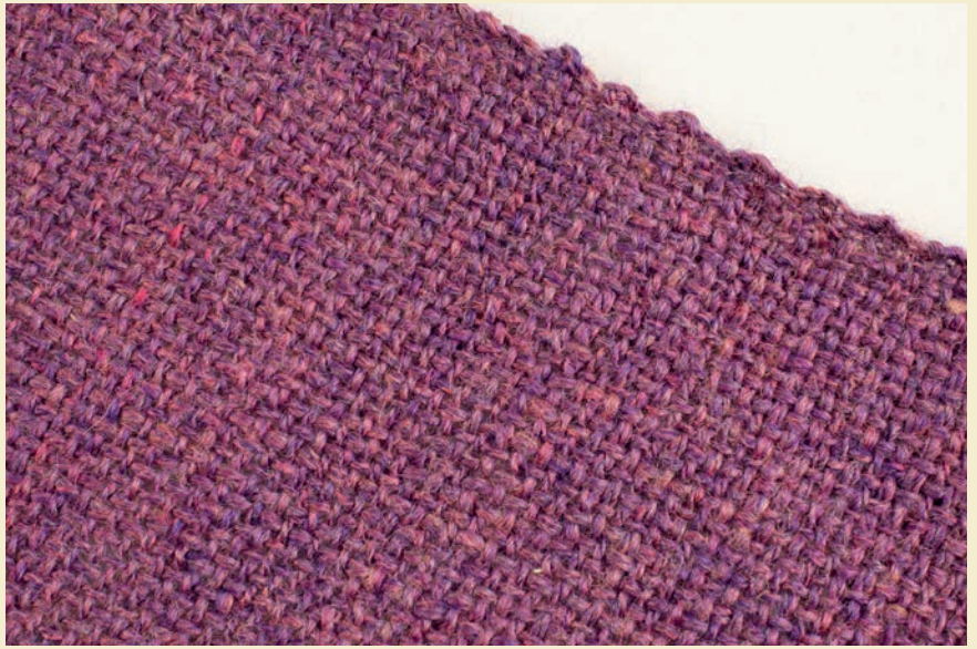
Alternate yarns in the warp and weft to minimize the overall effect of twist variations. In this sample, I alternated the warp and weft yarns end by end and pick by pick.
