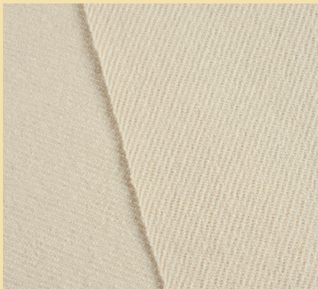
The same z2s warp and s2z weft was used in both of these twill samples. The twill direction in the left sample is from left to right; the twill direction in the right sample is from right to left. There is little difference between the two fabrics when viewed from the front.
