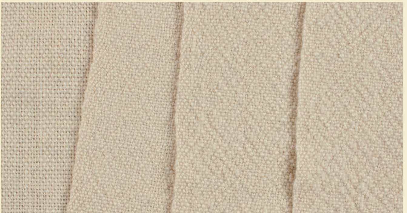
BLUEFACED LEICESTER. Left to right: unwashed; 9% lengthwise shrinkage after five minutes of agitation; 12% after ten minutes; 12% after fifteen minutes.
