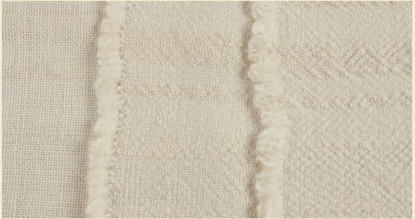
MERINO/BLUEFACED LEICESTER WARP WITH MERINO WEFT. Left to right: unwashed; 12% shrinkage after five minutes of agitation; 13% after fifteen minutes.
