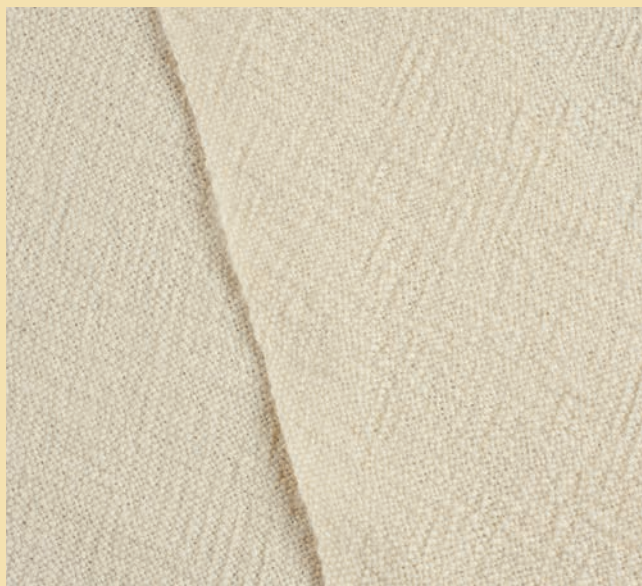
The same z2s warp was used in both of these plain-weave samples. Left: z2s weft at 11 picks per inch (ppi). Right: s2z weft at 13 ppi.
