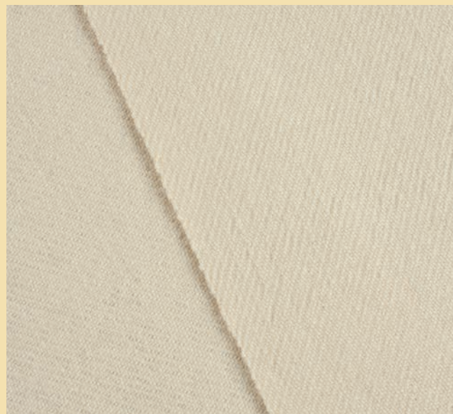
The same z2s warp and z2s weft was used in both of these twill samples. Left: twill direction from left to right. Right: twill direction from right to left.
