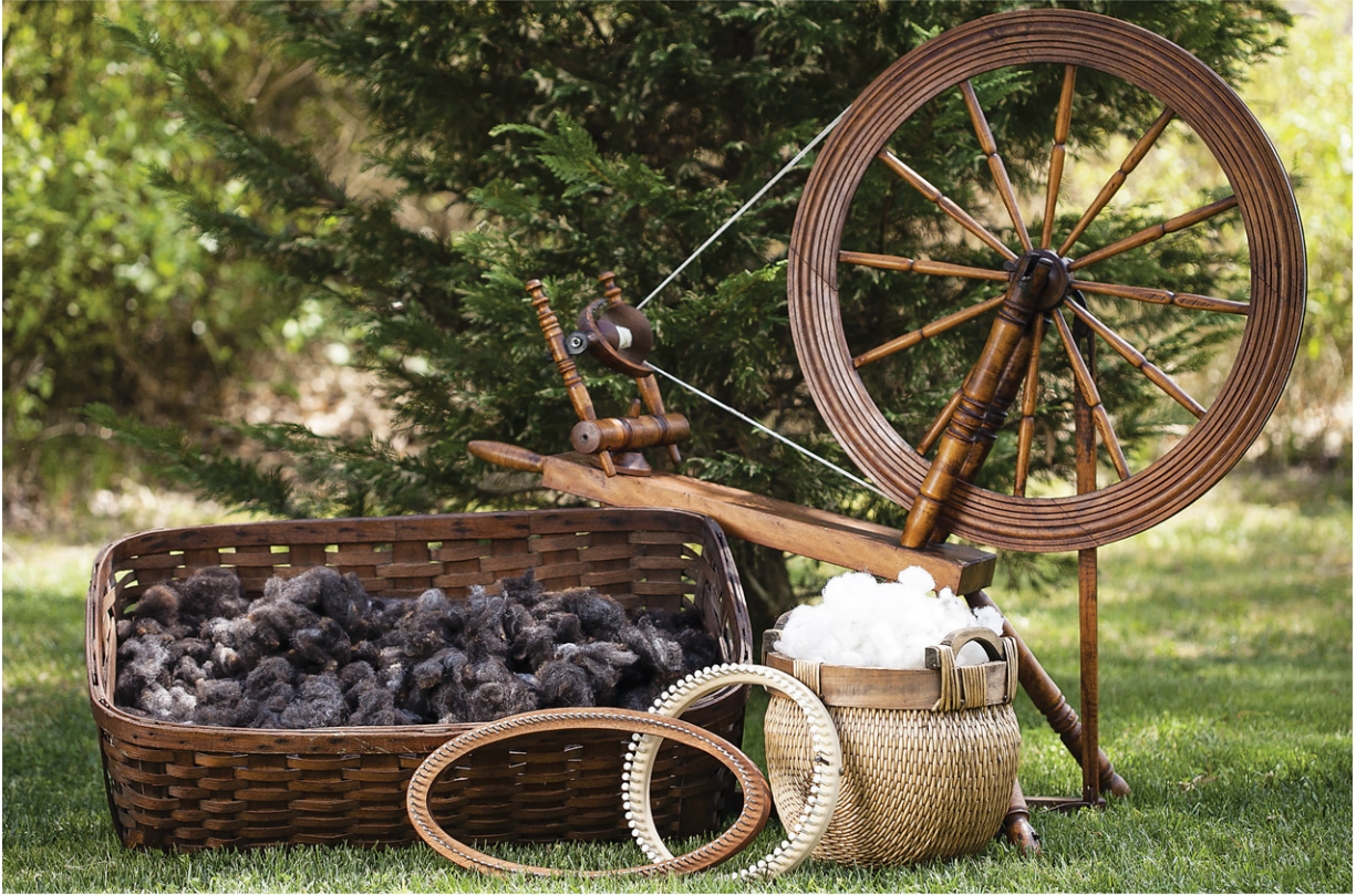
Raw wool before spinning; wool is washed, carded, and then spun by hand or machine into the strands that will become yarn.
