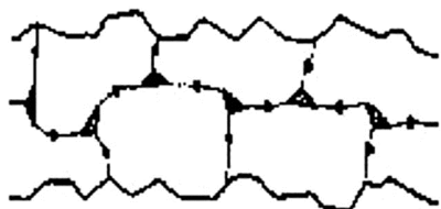
Fig. 183 Polyglucose chains cross-linked with "cellulose reactants"
