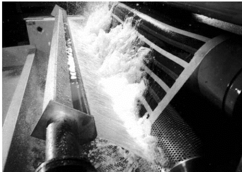
Fig. 21 Water-sheet washing system
