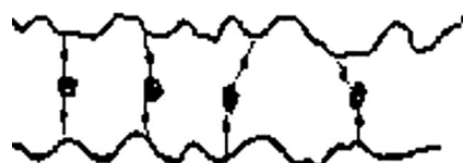
Fig. 184 Polyglucose chains cross-linked with thermosetting resins
