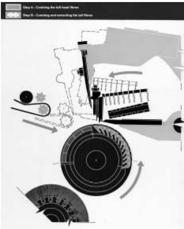
Fig. 182 - Combing machine with double combined motion
