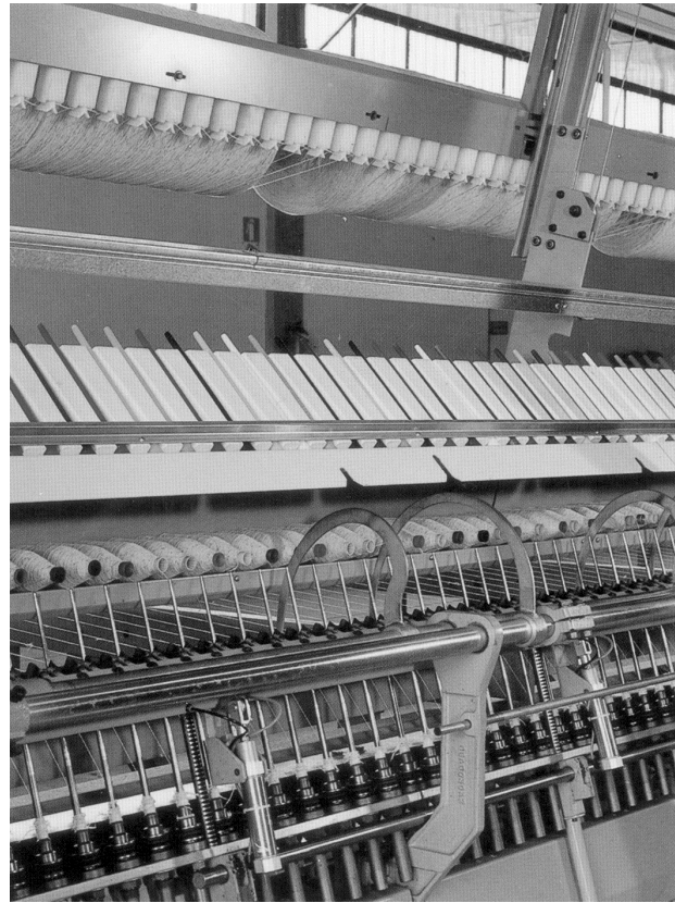
Fig. 100 Tubes orderly positioned on the rack
