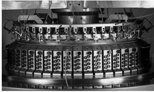
Picture 90 – Cam adjusting system with external screw
