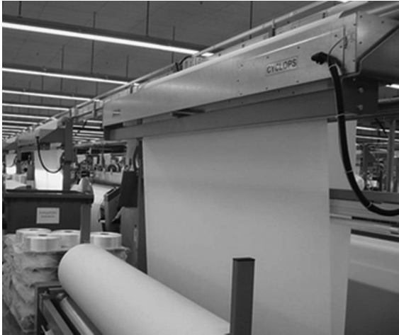
11.7 New Cyclops automatic on loom fabric inspection system.
