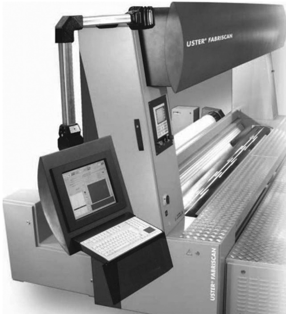
11.4 Uster Fabriscan inspection system.
