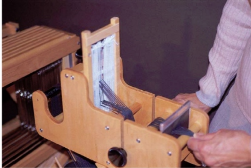
3. Raise the tension box harness. Place holding thread through the shed.
