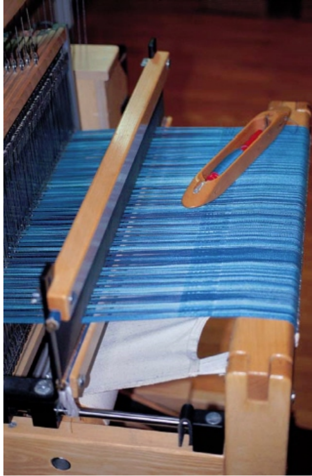
A sliding beater is my favorite, shown on AVL's Studio Dobby Loom.
