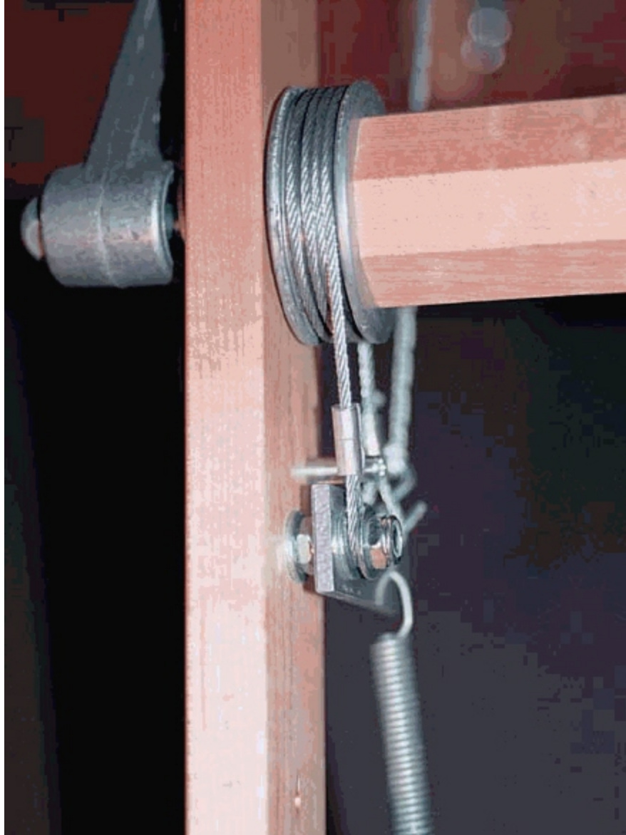
Friction brake on the Schacht Baby wolf loom.
