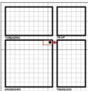
The first two analyzed weft threads are filled in the drawdown area of the draft.
