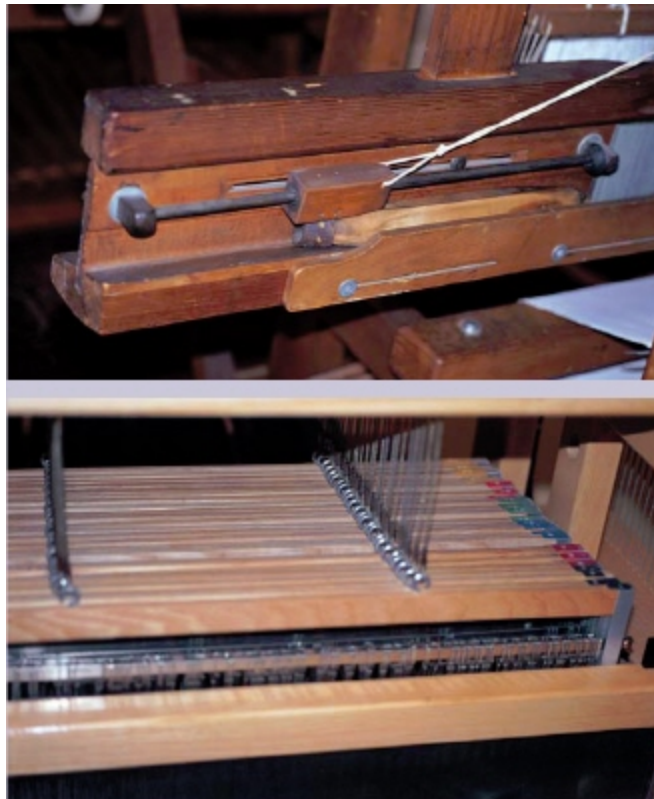
The fly shuttle at a countermarch loom (top): a bank of 24 shafts on an AVL Studio Dobby loom, each four color-coded with label tape (bottom).
