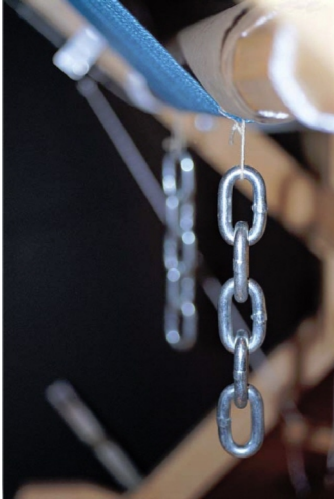
Aluminum chain links tied around selvedge threads.
