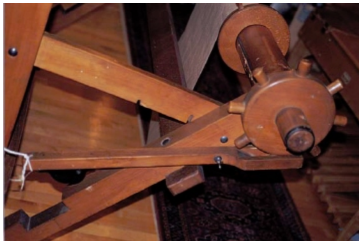
The brake (wheel with spokes) on Anni Alber's counter-march loom.
