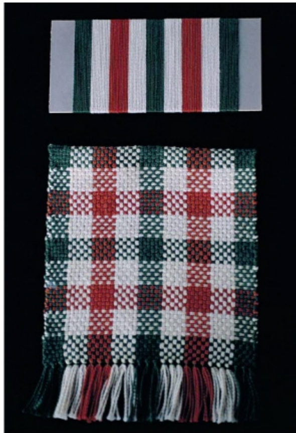
Basket weave sample with color wrapping. The sett for 50/50 basket weave is closer than 50/50 plain weave because in basket weave, each thread interlaces with every other thread.
