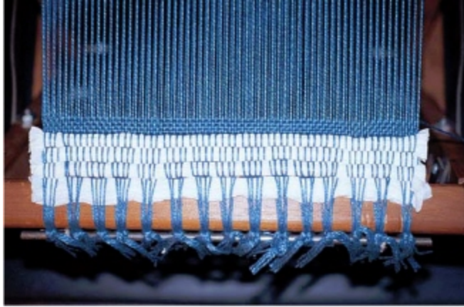
The warp tied on, spread out with bath tissue, and a few picks woven in.
