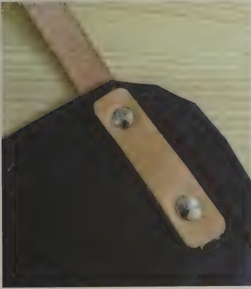
Fig. 1 Rounded corners and the leather rivet piece on the back of the apron.
