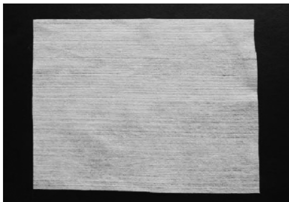
1.13 Hydroentangled non-woven sheet from Biocelsol and PET staple fibres made by Suominen Nonwovens Ltd [183].
