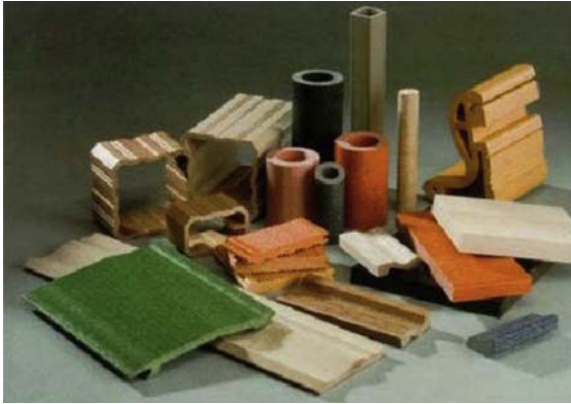
Figure 14.5 Pultruded NFC products (courtesy of M.T. Ton-That et al, The Institute of Textile Science, Ottawa, ON, Canada).
