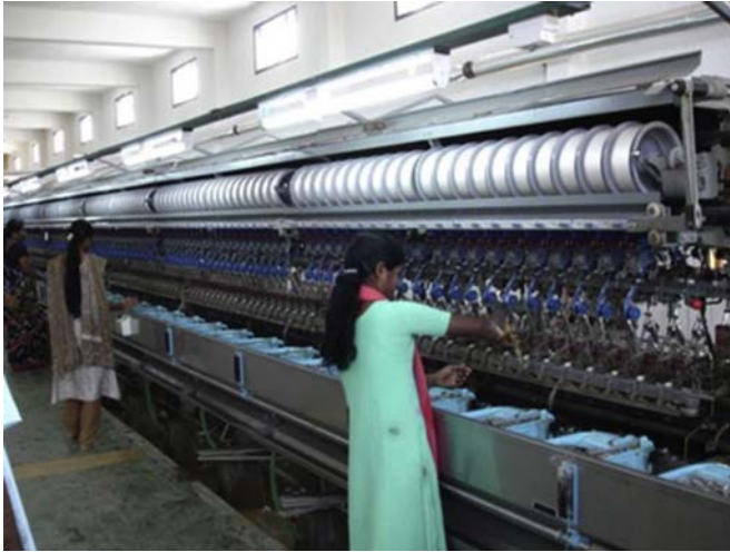
Figure 3.10. Automatic silk reeling machine.
