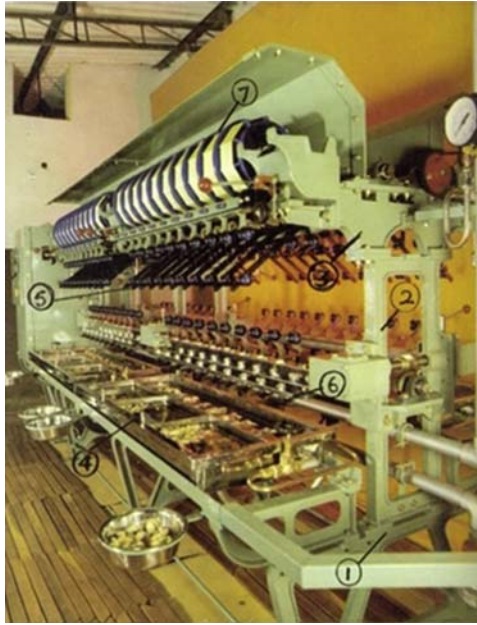
Figure 3.9 Multi-end silk reeling machine.
