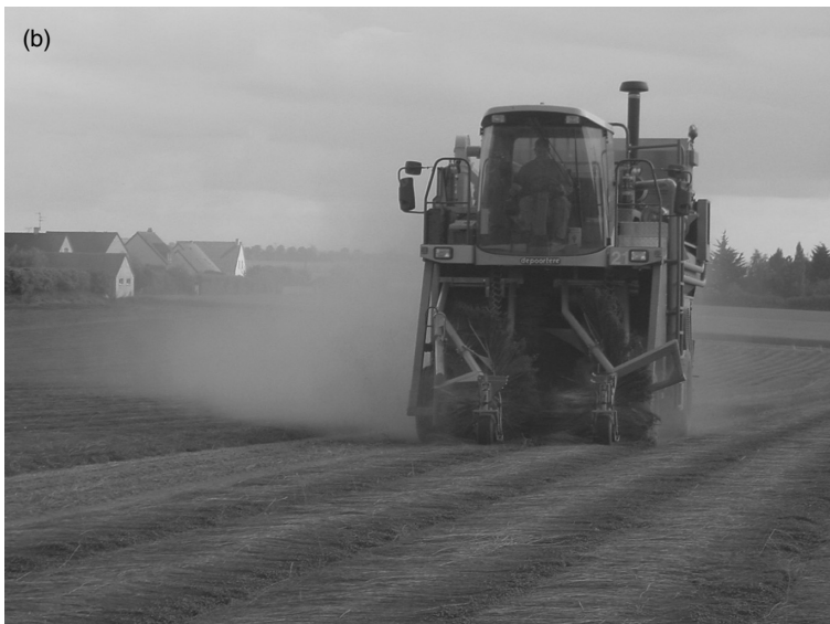
5.1 Photographs of pulling, deseeding and turning machines used by Belgian company Depoortere. (a) Pulling machine, double row with cabin, (b) deseeding machine, double row 1, (c) turning machine, double row 2.
