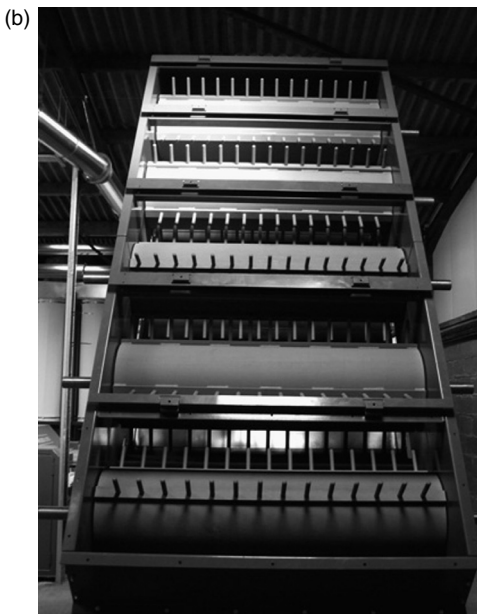
6.6 Step cleaner. Side view (a) and rear view showing rollers and beaters (b).
