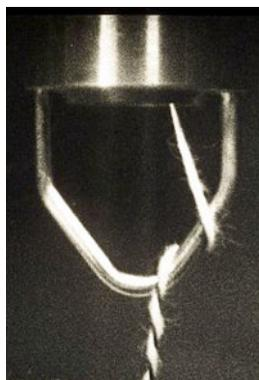
**FIGURE 6.30** Hollow-spindle wrap spinning system.
