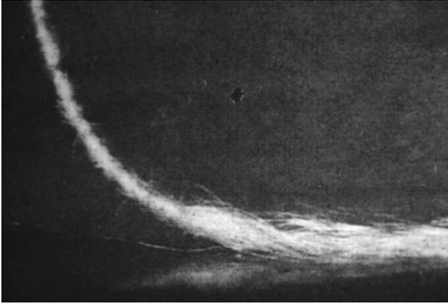
**FIGURE 6.43** Twist insertion with smooth doffing tube navel.
