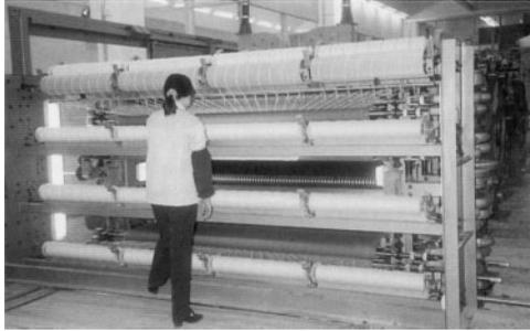
**FIGURE 3.18** Bank of Rub Aprons. (Courtesy of Befama Ltd.)
