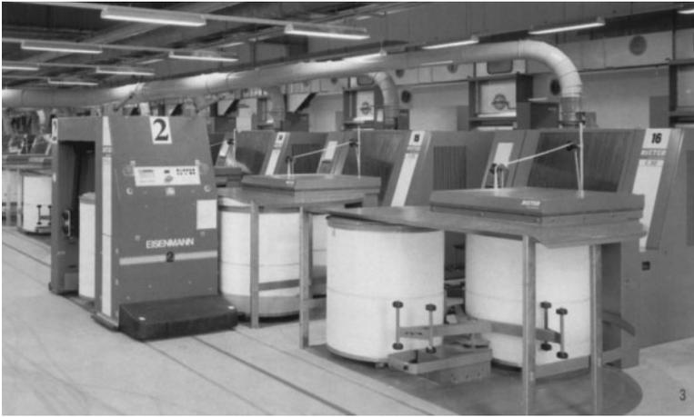
**FIGURE 3.3** Short-staple carding line. (Courtesy of Rieter Machine Works Ltd.)
