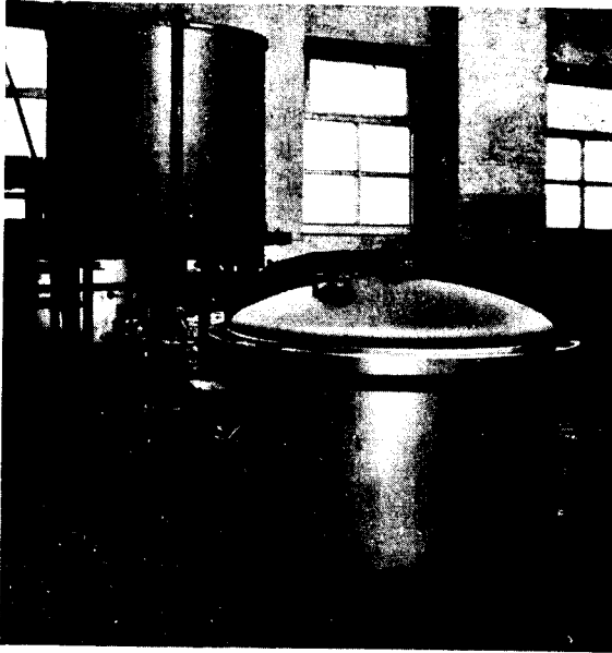
Fig. 13.7(a) High-temperature machine for dyeing tops (Courtesy of Longclose)
