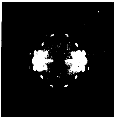
Fig. 2.7 X-ray diagram of Terylene
