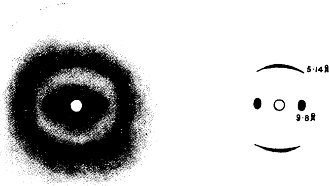
Fig. 5.14 X-ray diagram of \alpha keratin
