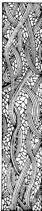
Fig. 2.9—Fibrillar structure in a man-made fibre
