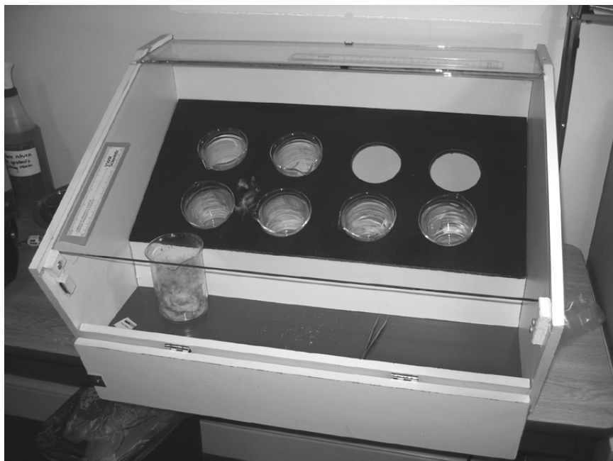
2.8 Separation cabinet (source: Peter Lieber).
