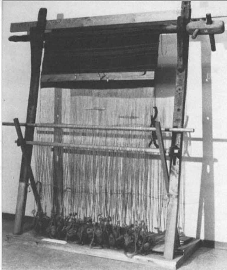
2-9: Icelandic warp-weighted loom, reconstructed and set up before 1914. National Museum of Iceland. Photo: Gísli Gestsson.
