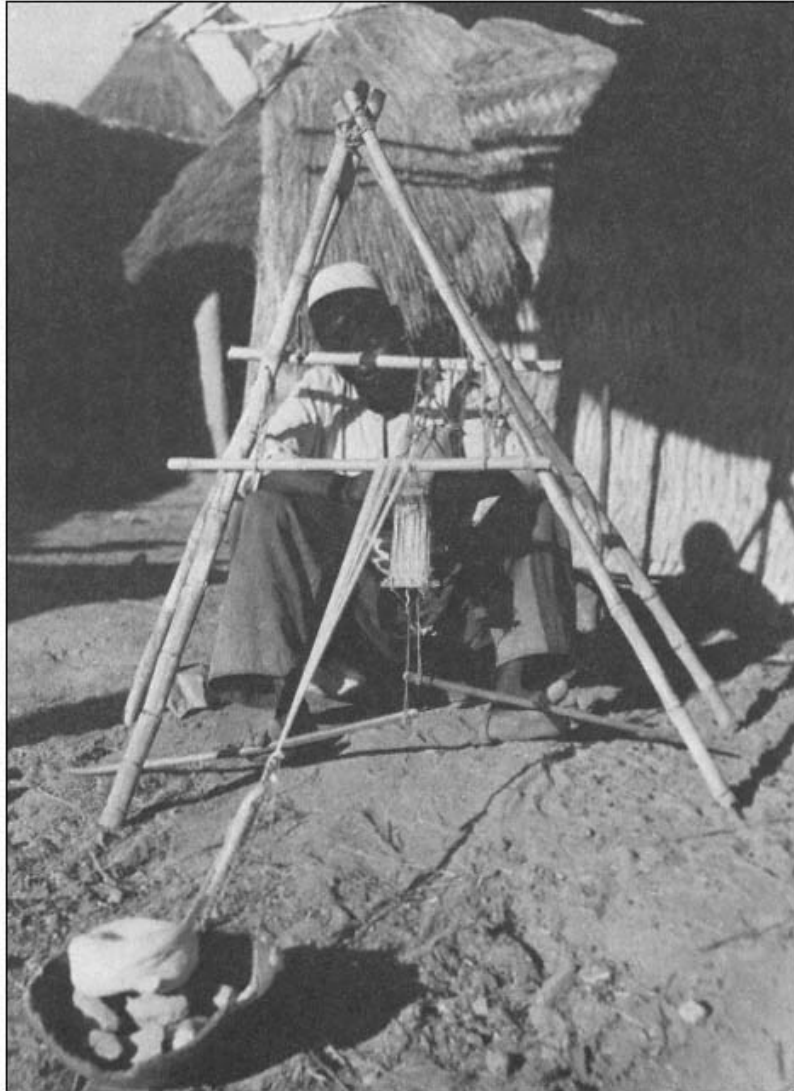
The loom frame consists of a tripod arrangement that contains the shedding apparatus. The cloth beam is fastened to two uprights behind the weaver. In both cases the warp is stretched out and held taut by weights on the ground. Photographs by René Gardi.
