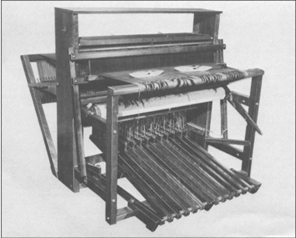
A twelve-harness jack loom ("Nilart") with jacks that raise harnesses from below. Made by Leclerc, L'Islet, Quebec, Canada.
