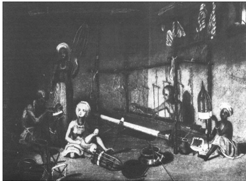
6-8: Indian pit loom with roller beams. From Gilroy, The History of Silk, Cotton, Linen, Wool and Other Fibrous Substan
