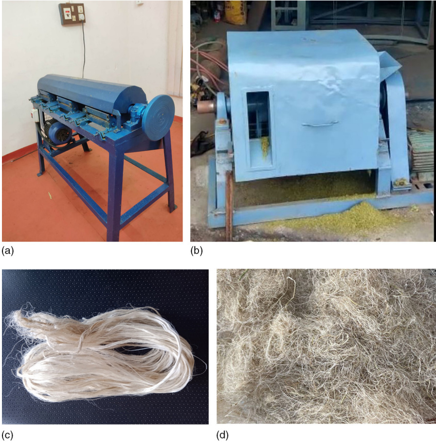
FIGURE 3.1 (a) Fiber decorticator for long fiber extraction, (b) short PALF extraction machine, (c) fibers obtained from long fiber decorticator, (d) fibers obtained from the short fiber extraction machine.
