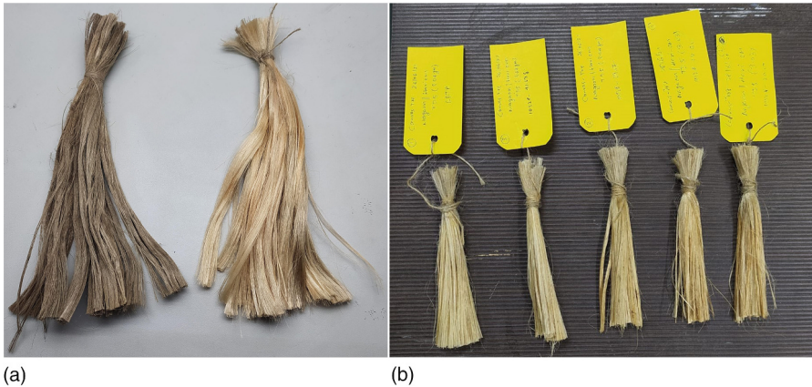
FIGURE 1.12 (a) Untreated jute fiber and EDTA treated “goldenized jute”, (b) Change in jute colour with increase in EDTA.
