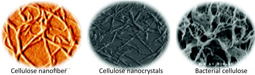
FIGURE 9.2 Morphologies of nanocellulose: CNF, CNC, and BNC. (Permission from Norrahim et al. [14].)
