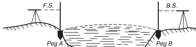
Fig. 6.36. Levelling across a pond.
