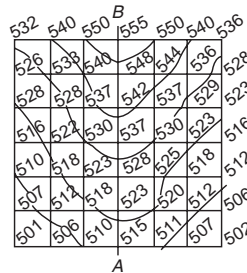
Fig. 7.13. Locating contours by method of cross-section.
