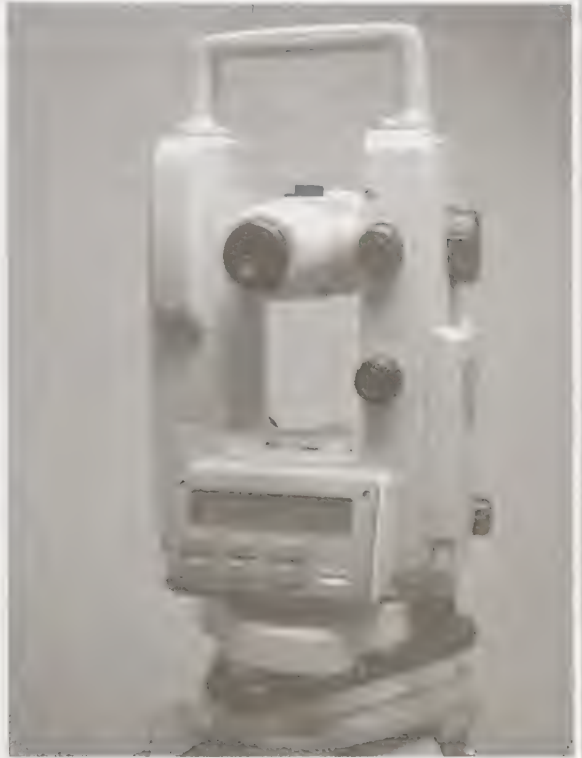
Topcon DT 20. 20" Electronic theodolite
