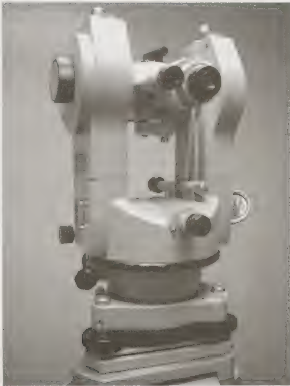
Sokkia TM20E. 5" optical micrometer theodolite
