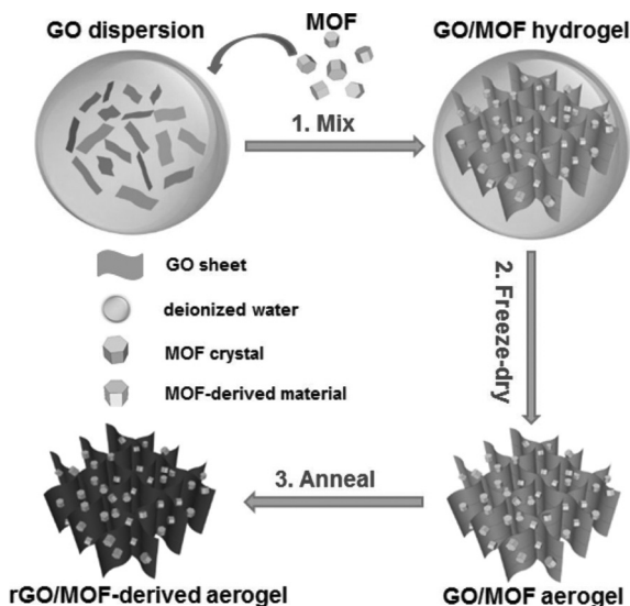
FIGURE 15.8 preparation method of GO/MOF composites for supercapacitor applications. (Reprinted with permission from Xu, M.W. et al., J. Solid State Electrochem. , 11, 372–377, 2007, Copyright 2007 American Chemical Society.)
