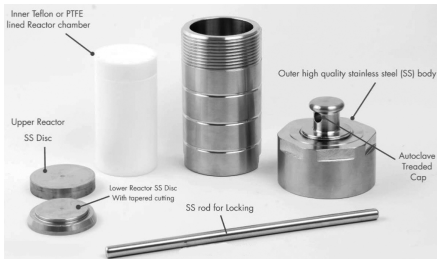
FIGURE 10.18 Generally used reactor (autoclave) during hydrothermal/solvothermal synthesis.
