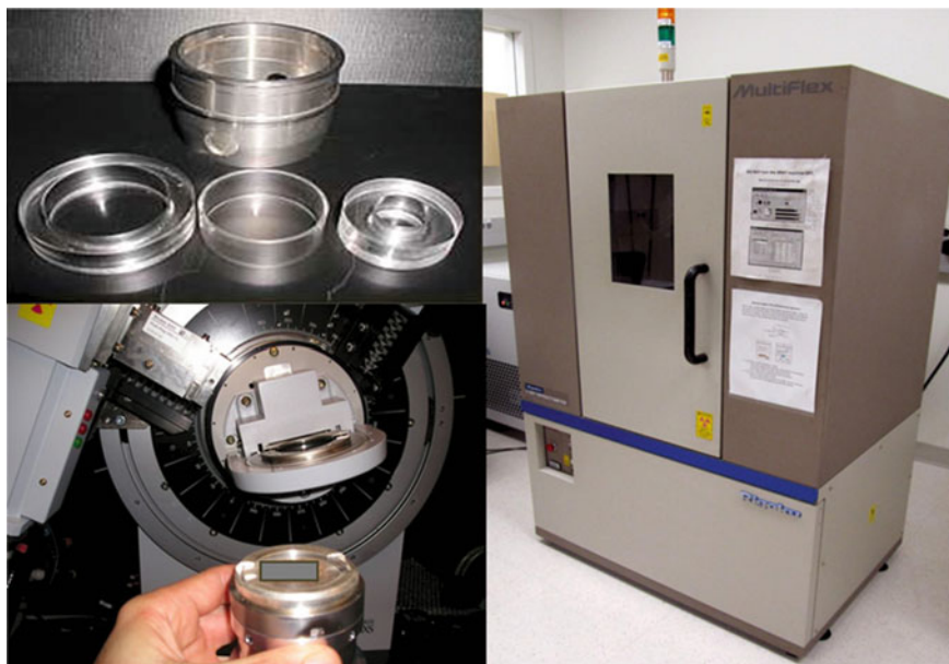
Fig. 4.3 Actual photograph of X-ray diffraction unit (Hanyang University, Korea)
