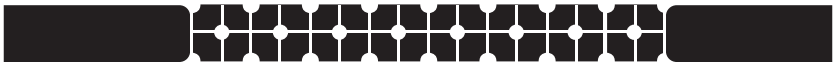
FIGURE 7.24 Grid structure for an array of staggered circular cylinders in a cross-flow with inlet and exit plenums.
