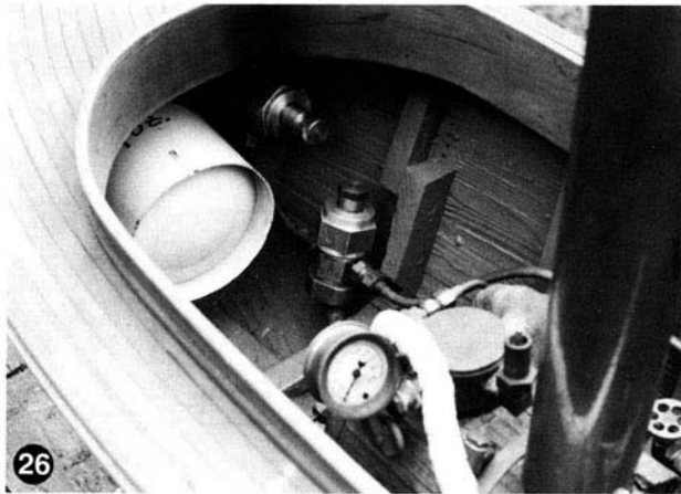
The regulator and attenuator must be easily removable but need not be available for ordinary running.
