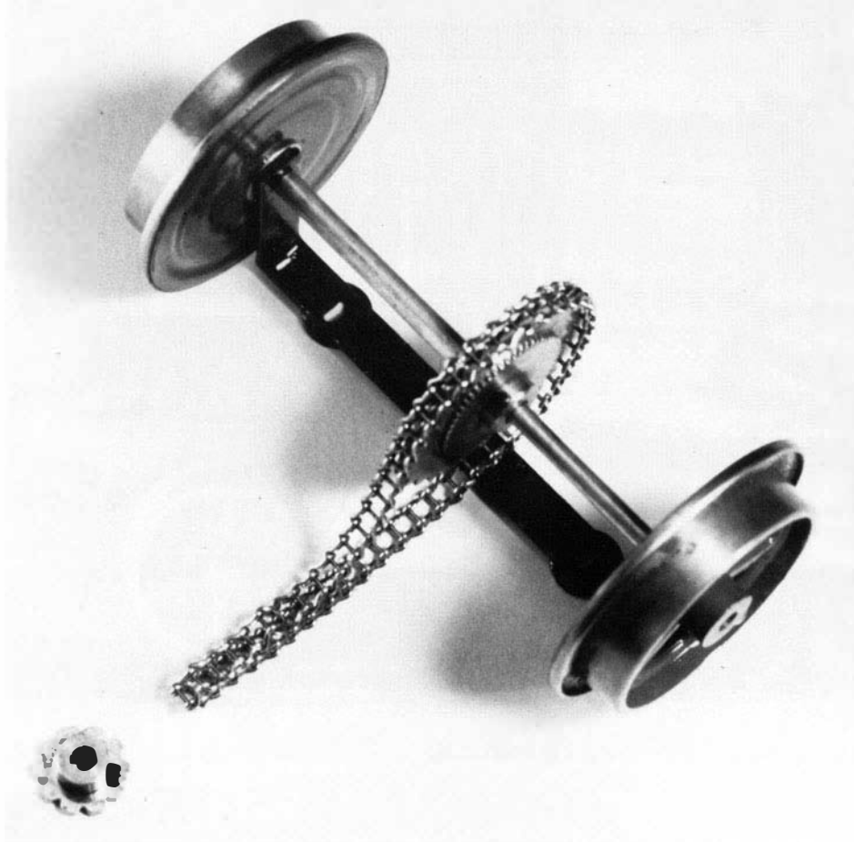
The drive mechanism with the ladder chain and gearing shown.
