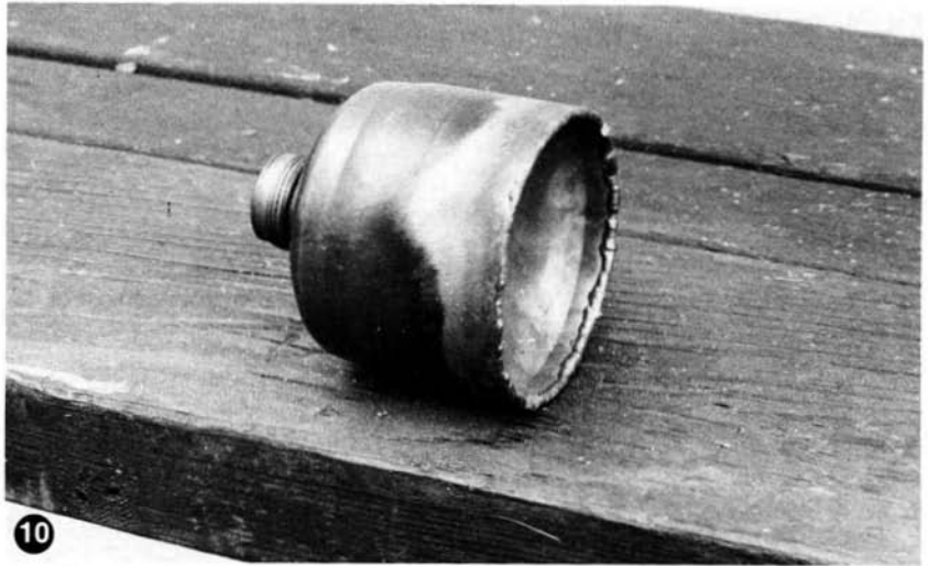
An attempt to make up a very small bottle. It leaked from my bad welding.
