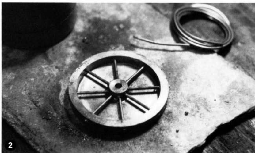
The spoke holes have been drilled through the rim and into the hub, spokes inserted, and soft soldered in.
