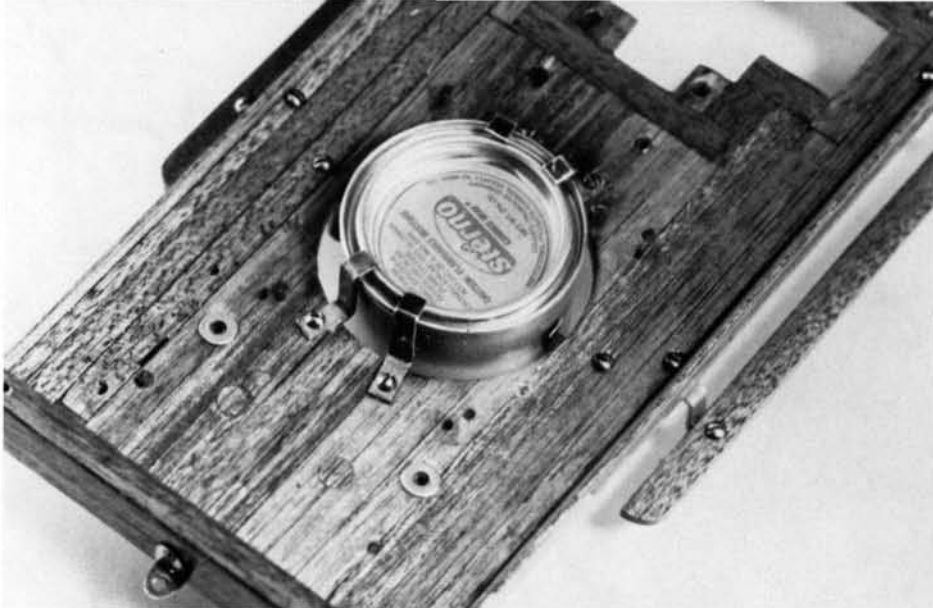
The Sterno can held in place on top with 1/4" brass strips.
