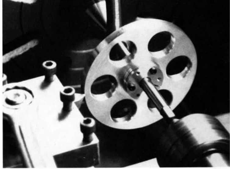
Assemble the bushing and web. Finish turn + .003'' for 3 thou pressed fit into the outer ring.
