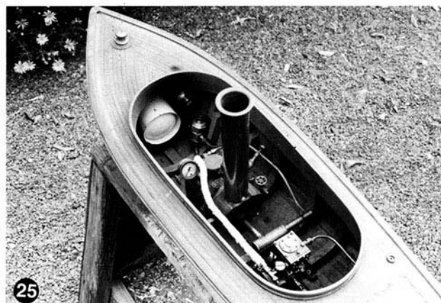
The hardware installed in the boat. The main gas valve is the capstan on the foredeck. Radio gear is under hatch covers.
