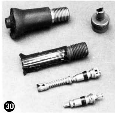
30 Valves that are junked in tire shops and are quite satisfactory for our use. The shorter valve core must be used.
