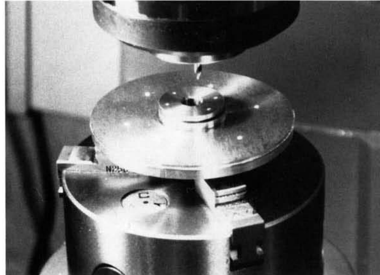
Locate and drill holes with the web and bushing assembled.
