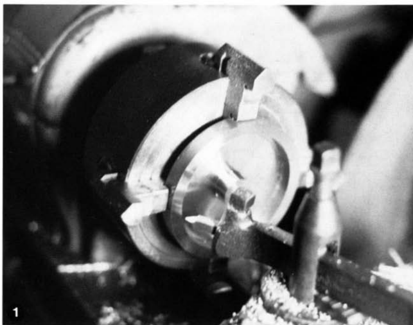
The flywheel disk has been faced, drilled and reamed, and a recess cut to form the rim and hub. A scant \frac{1}{32} " of stock still connects rim and hub.
