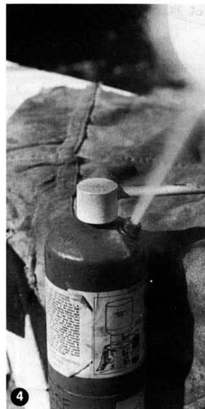
When the bottle is full, a heavy mixture of gas and liquid issues from the vent.
