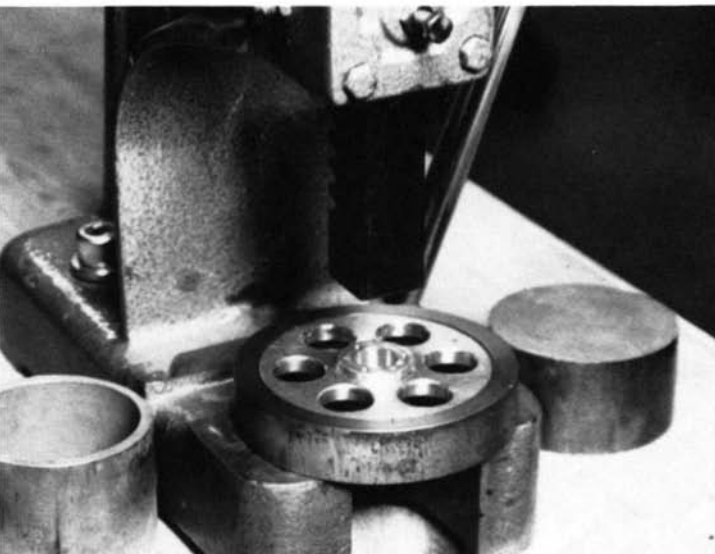
Pushing the cold inner web into the hot outer ring.
