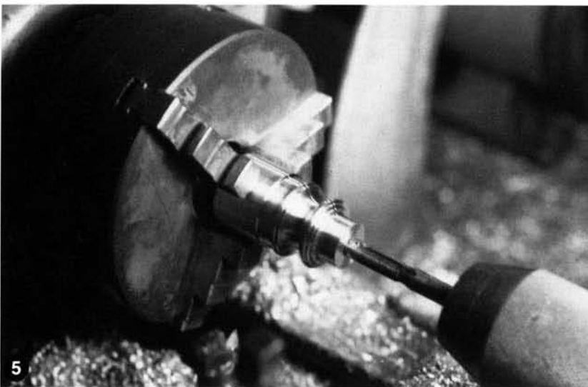
The column base is being tapped 1/4-32. Note the "free" turning to produce a contoured architectural form.
