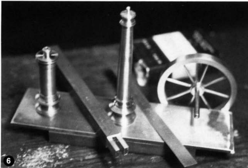
6 Cylinder, Column, Flywheel, and Baseplate. The column top bearing has been roughed out by milling.
