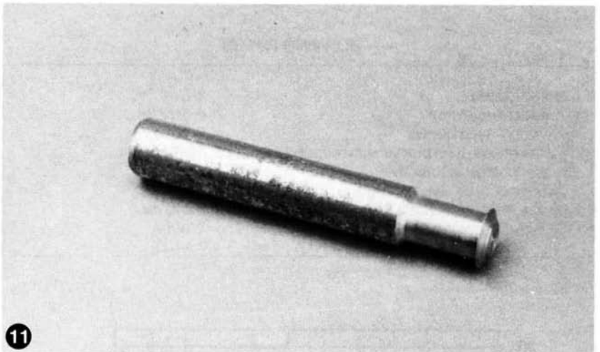
Hook tool used to remove the plastic O-ring retainer from the neck of the bottle.
