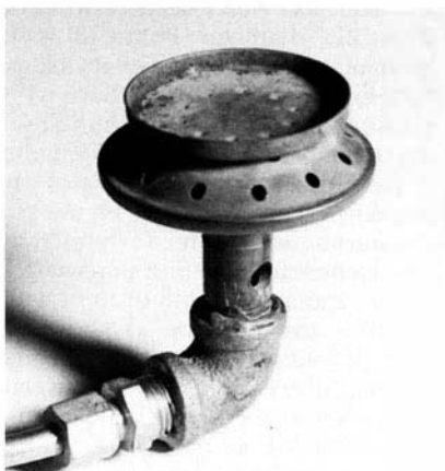
The versatile and "almost indestructible" sheet metal water heater burner as used on many locomotives.
