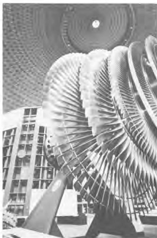
Fig. 2. The blading of a 220 MW LP turbine rotor
