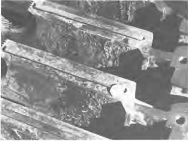
Fig. 4. Heavy chemical deposits on diaphragm
