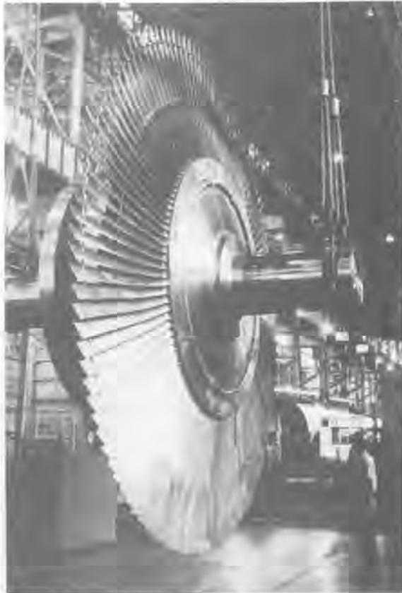
Fig.2 52-inch LSB Test Wheel
