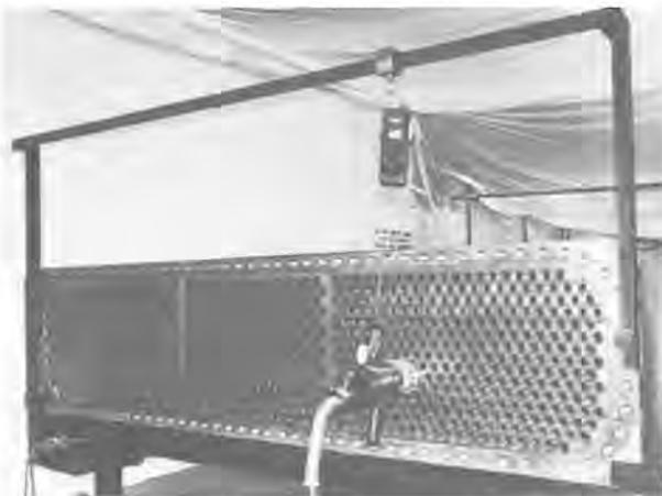
Fig. 5 : Automatic orbital T.I.G. tube to tubeplate welds between Type 439 finned tubes and Inconel weld clad reheater tube bundle header.
