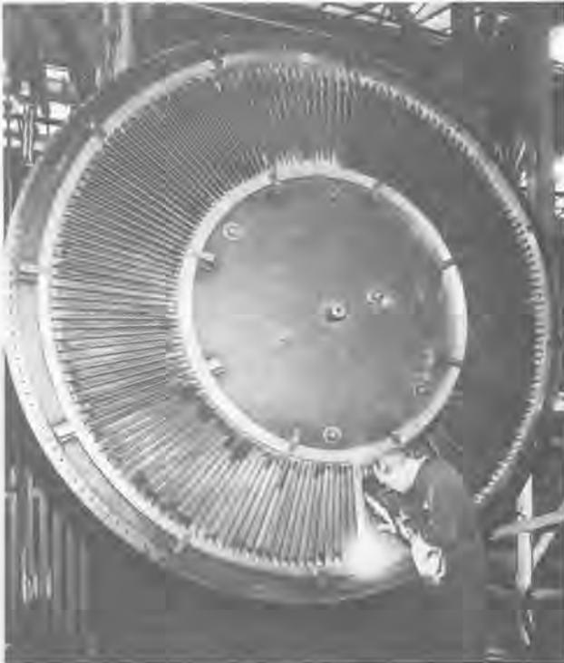
Fig. 2 : Welding of swirler blade ring.
