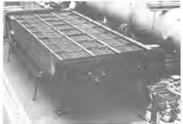
Fig. 6 : Finished reheater tube bundle with Type 439 finned tubes.
