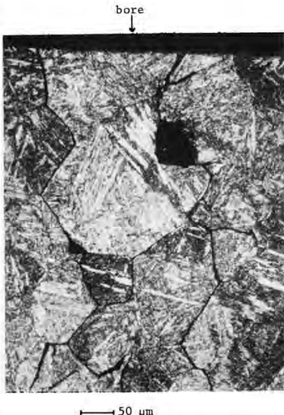
Fig. 5. Appearance of one of the cracks of the bore.
