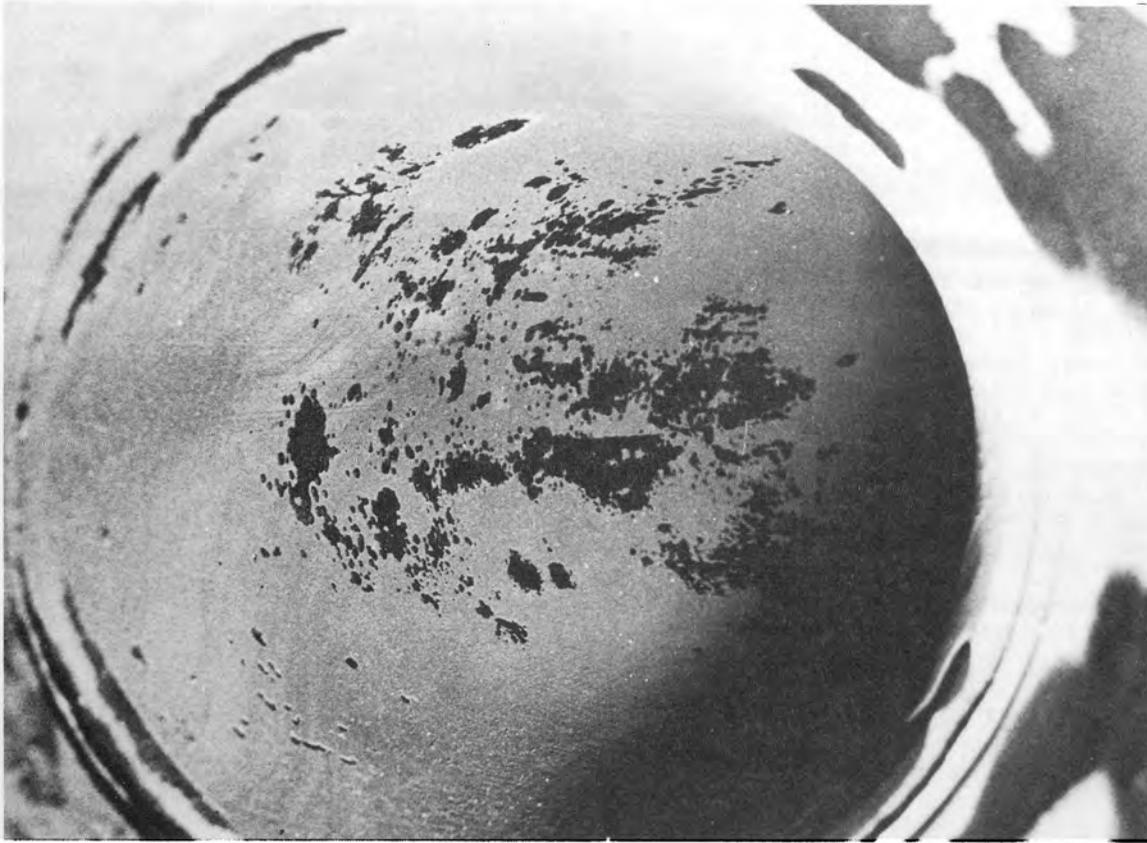
Fig. 3 - Erosion/corrosion of carbon steel bled steam pipe.
