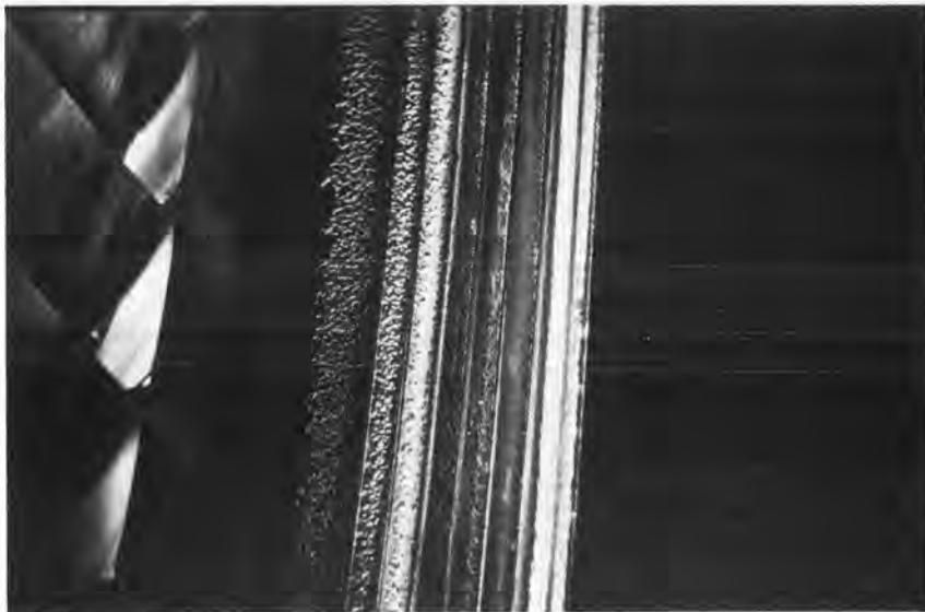
Fig. 3. Drop impact erosion between shroudings in inner casing of LP-part of Biblis turbines
