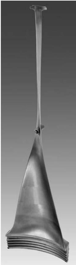
**Figure 5-2. A steel LSB of GE/Toshiba with the length of 1,016/1,220 mm (40/48 in) for the rotation speed of 3,600/3,000 rpm, respectively. Source: A. Mujezinovic<sup>1</sup>**
