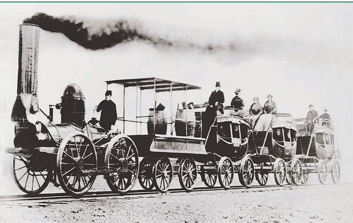
**The first passenger trains were stagecoaches equipped with railroad wheels pulled by a steam locomotive. The coaches' backless wooden seats and low roofs were so uncomfortable that they prompted George M. Pullman to develop his Pullman Sleeper cars, which made it possible for travelers to ride in comfort.**
