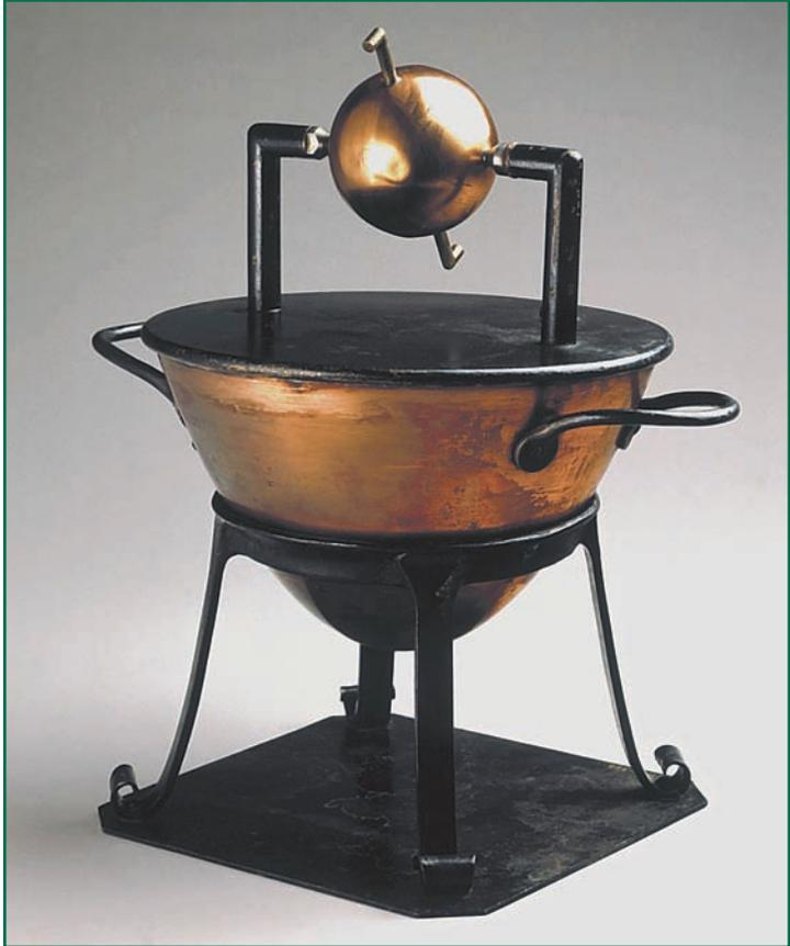
**Hero, a Greek mathematician of the first century, invented this early steam engine. Called an aeolipile, it was a hollow ball into which steam from the sealed cauldron of boiling water rose. The short pipes extending from the ball were bent at a right angle and emitted jets of the highly pressurized steam, causing the ball to rotate.**
