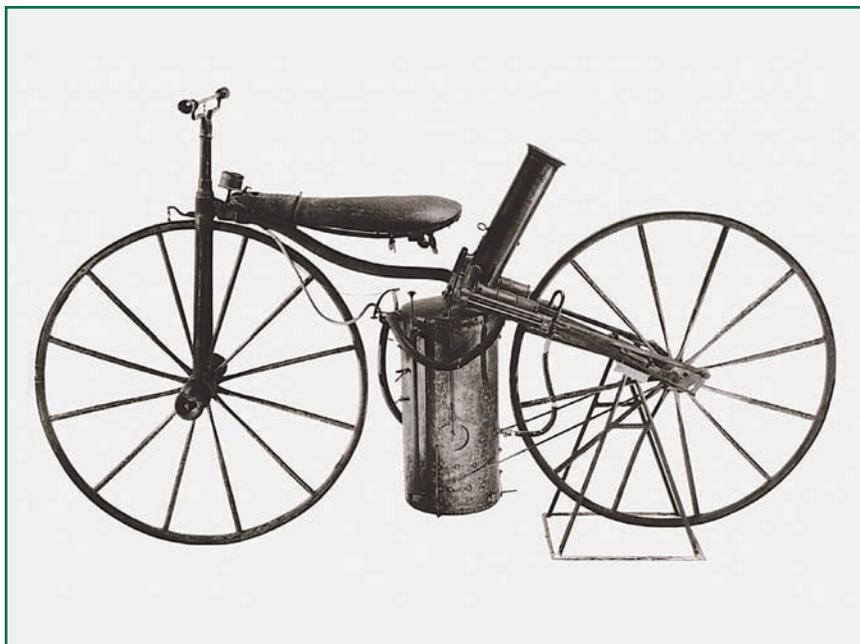
**This first motorized bicycle was steam-powered. Built by S. H. Roper in 1867, the steam engine was positioned underneath a raised seat. A precursor to the motorcycles driven today, the steam-powered bicycle could reach speeds of up to 19 miles per hour.**
