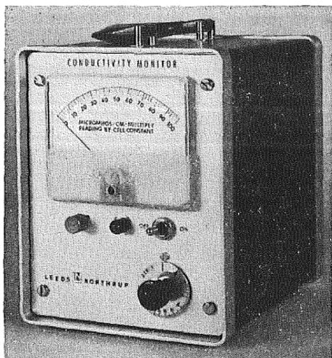
FIG. 3-3. Transistorized portable conductivity monitor that operates on 107 to 127 volts, 60 cycles, AC, is employed for a variety of solution conductivity measurements including condensate, demineralized water. (Courtesy of Leeds & Northrup Company.)
