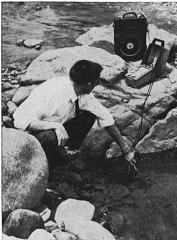
FIG. 3-8. Portable pH meters have many uses. This one is being employed on stream survey work. (Courtesy of The Bristol Company.)
