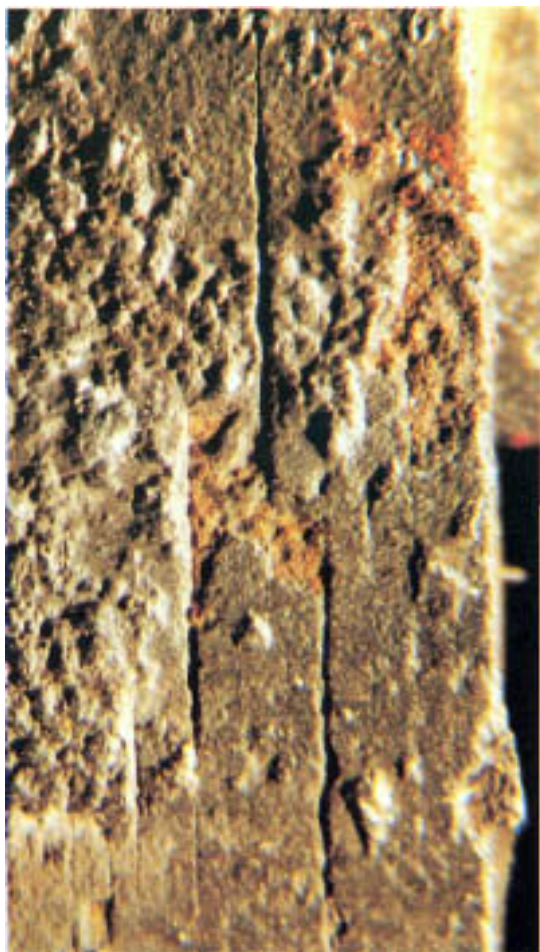
Figure 15.11 Secondary corrosion-fatigue cracks on external surface. (Magnification: 6.5 \times .)
