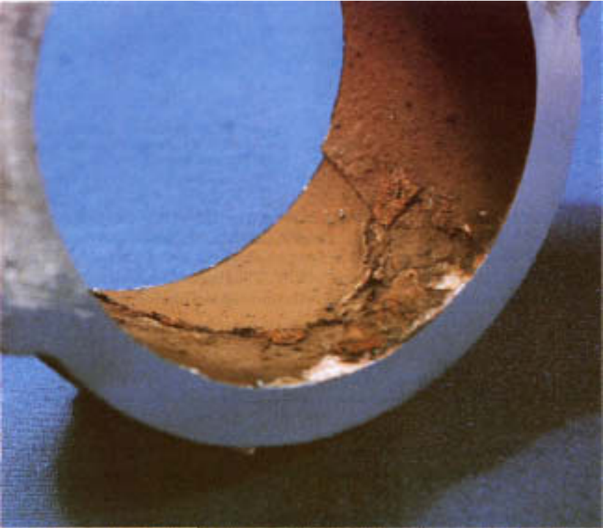
Figure 20.11 Internal surface of tube showing oval-shaped replacement window welded into place.
