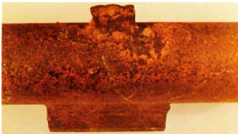
Figure 9.6 High-temperature corrosion at the base of an attachment (top of photograph) on a stainless steel reheater tube. (Courtesy of Electric Power Research Institute.)
