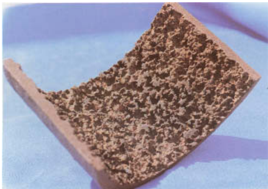
Figure 7.4 Jaggedness associated with severe acid corrosion. (Courtesy of Electric Power Research Institute.)
