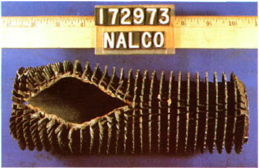
Figure 3.7 Large, wide-open rupture in a superheater tube of a waste-heat boiler. The tube experienced long-term overheating followed by a brief episode of short-term overheating when nearby tubes ruptured.
