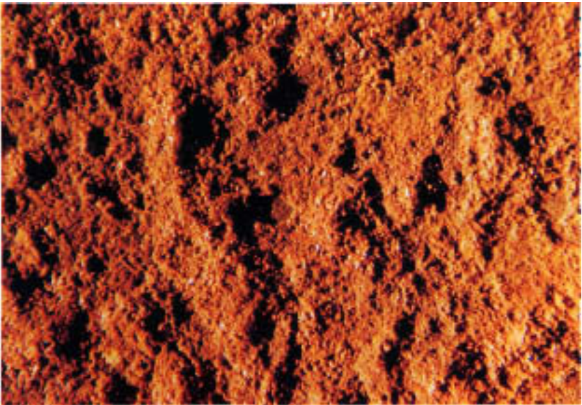
Figure 12.3 Pockmarked contour of economizer tube exposed to condensed sulfuric acid. (Magnification: 7.5 X.)
