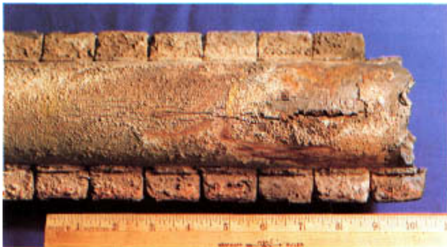
Figure 2.12 Longitudinal fissures along hot side. Note the through-fissure at the bulge apex.
