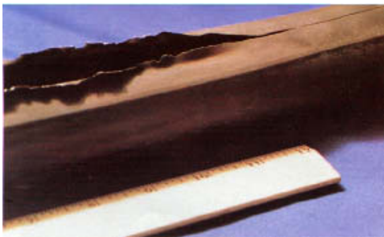
Figure 17.2 Tube rupture caused by a misdirected soot blower. Rupture edges are thin and ragged because of tearing of the wasted steel in the eroded zone. The tube surface is light gray and shiny as a result of erosion of the normally present fire-side oxides and deposits.
