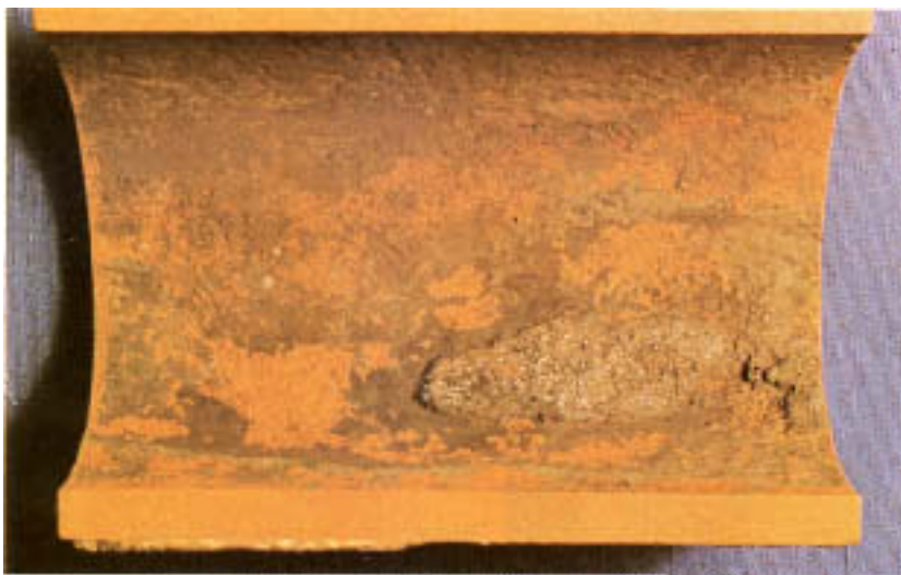
Figure 1.16 Patch of sparkling magnetite crystals associated with caustic corrosion site. Such crystals are often found near sites of acid and caustic corrosion.
