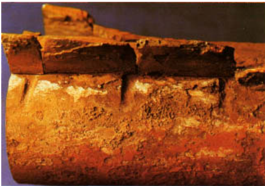
Figure 17.8 Deep grooves cut into the hot side of a waterwall tube. Grooving was caused by channeling of furnace gases containing entrained fly ash.
