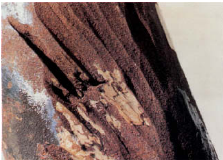
Figure 17.6 Grooving on pendant U-bend superheater leg caused by steam leaking through a corrosion-fatigue crack at the U-bend. Grooves were rusted after removal from boiler.
