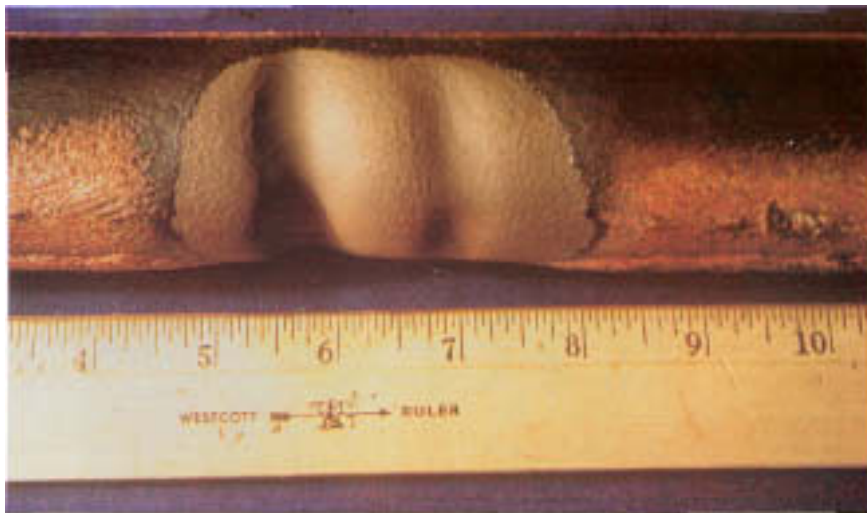
Figure 17.5 Utility superheater tube cut by steam leaking from an adjacent tube that failed at a manufacturing defect. Note the smoothly undulating surface and removal of red and black oxides and deposits in the wasted area.
