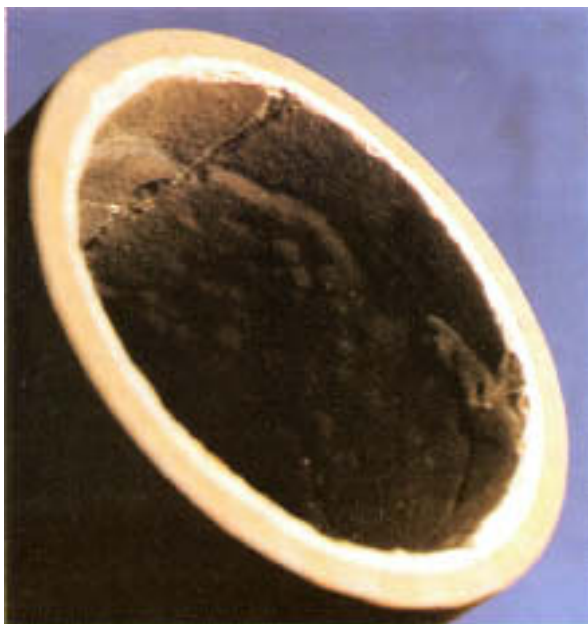
Figure 1.17 Calcium carbonate deposit (see Fig. 1.10).
