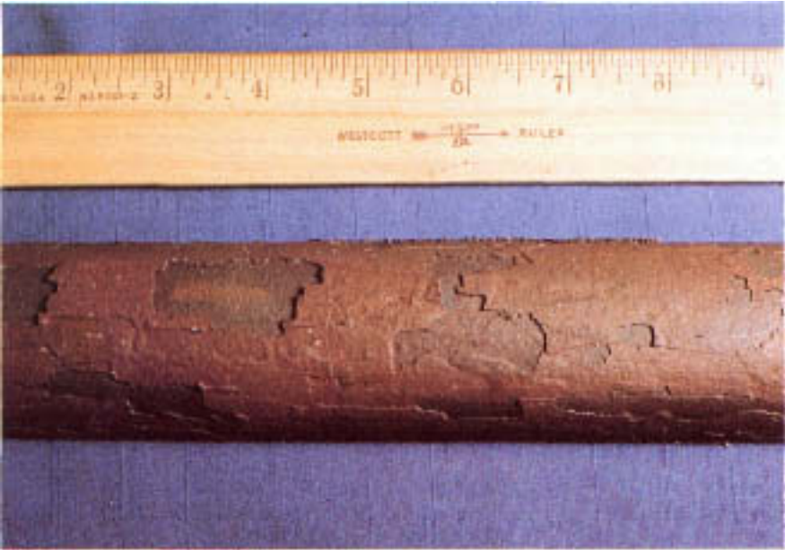
Figure 2.11 Severe thermal oxidation and spalling of magnetite on external surface. The laminated nature of the scale indicates multiple episodes of spalling and oxide reformation.
