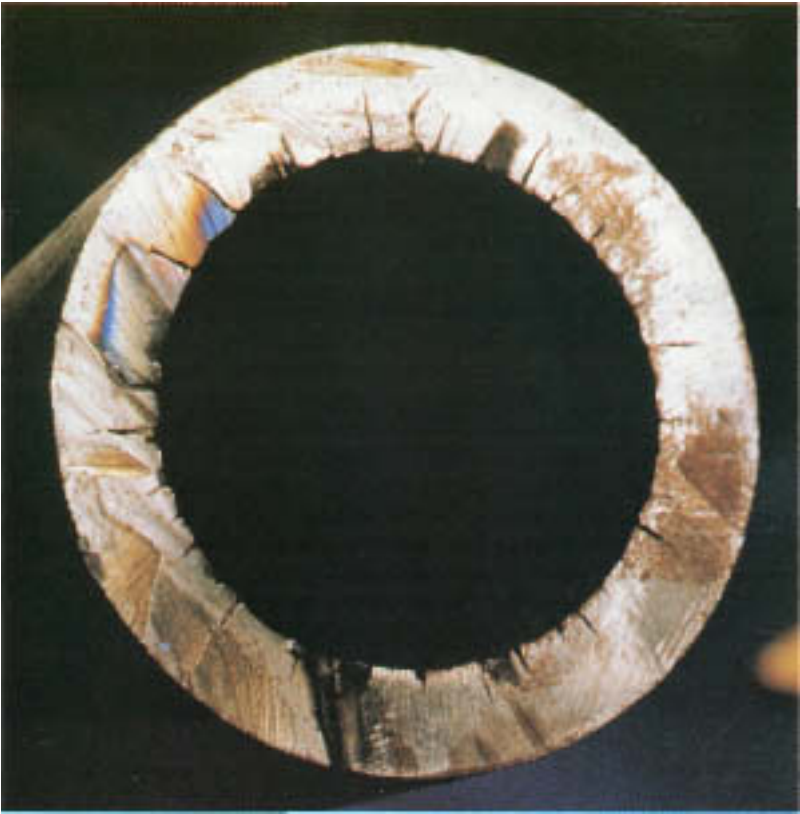
Figure 15.7 Cross section through cracks.
