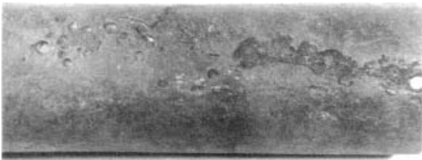
Figure 9.5 Oil-ash corrosion on stainless steel reheater tube. (Courtesy of John Wiley and Sons, Metallurgical Failures in Fossil Fired Boilers , by David N. French, New York, 1983.)
