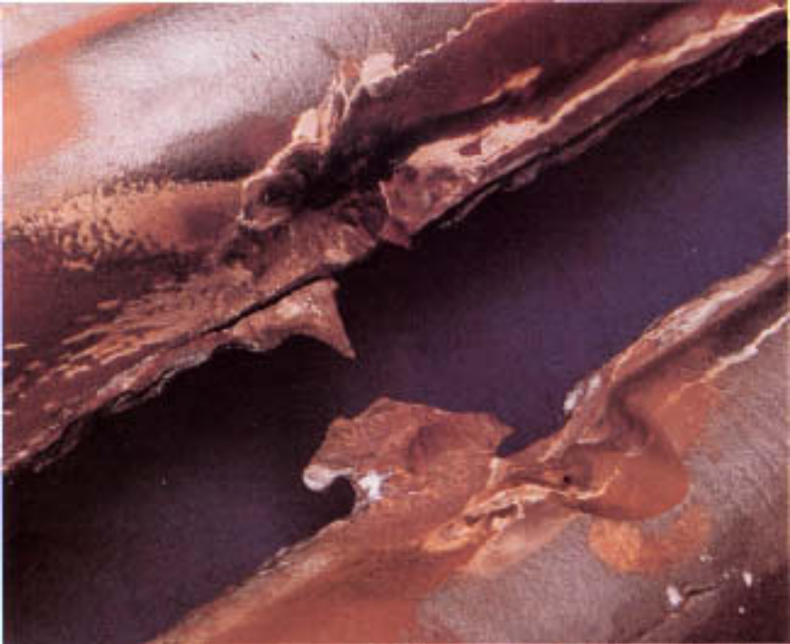
Figure 17.20 Steam cutting of utility convection tubes. The original failure occurred at a welded support bracket and was due to corrosion fatigue. The adjacent tube was breached by escaping steam from the original failure.
