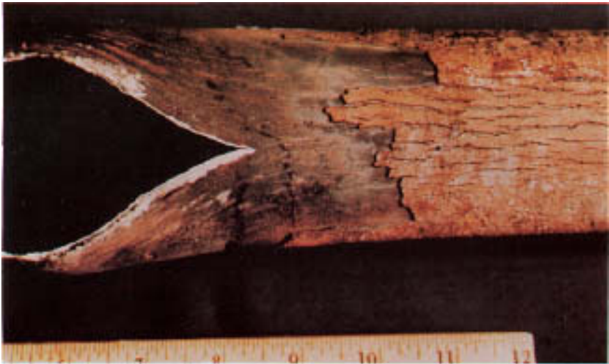
Figure 2.5 Thermally deteriorated metal on failed wall tube of a utility boiler. Note the spalled and cracked oxide resembling tree bark caused by expansion of tube during bulging and thermally induced stresses.
