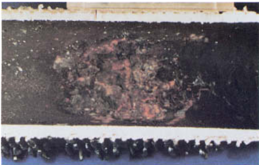
Figure 6.8 Gouging along internal surface opposite fins.
