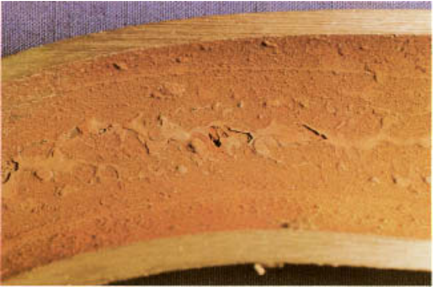
Figure 1.5 Fragmented hematite layer on an internal surface of an economizer. Most oxide was formed in place, but some was moved as fragments and chips.
