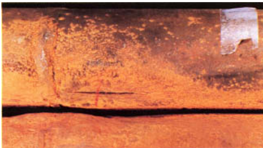
Figure 19.2 Seam defect (top tube). External metal loss on the bottom tube is the result of erosion from mixed steam and water escaping through the rupture.
