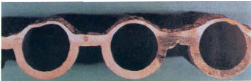
Figure 11.2 Severe fire-side metal loss on waterwall tubes. (Courtesy of Electric Power Research Institute.)
