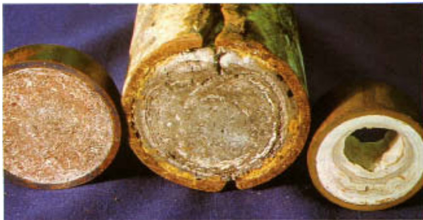
Figure 1.10 Tube sections virtually plugged with deposits. The tube on the right is from a low-pressure boiler and is fouled with almost pure calcium carbonate. The center tube contains silicates, phosphates, and other compounds; fouling occurred on standby service. The section on the left is reddened by almost 20% elemental copper. Such heavy deposition can occur only when internal pressures are low. Otherwise rupture would occur.
