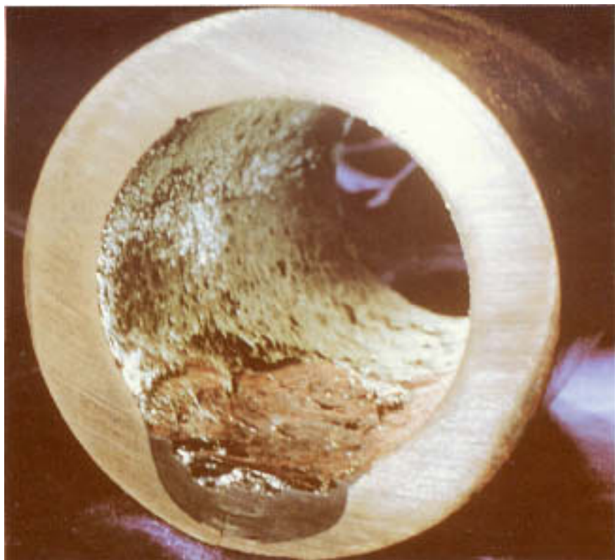
Figure 4.3 Deep caustic gouging beneath insulating internal deposits. (Courtesy of National Association of Corrosion Engineers.)
