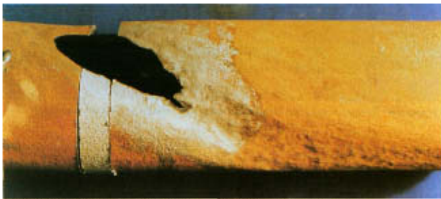
Figure 13.7 Grooving and perforation of a slanted tube resulting from corrosive water dripping from above.
