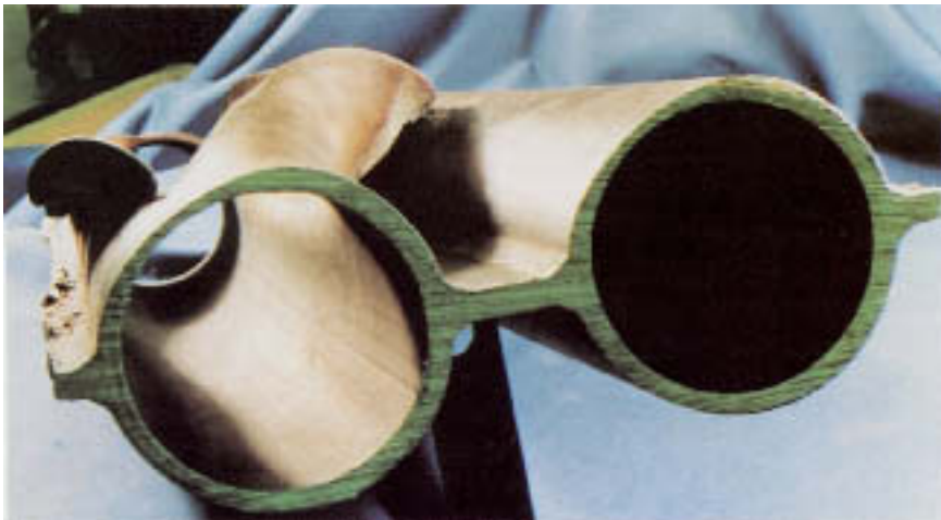
Figure 17.16 Ruptured division-wall tube from fluidized-bed boiler. Attack was caused by sand abrasion in the bed.
