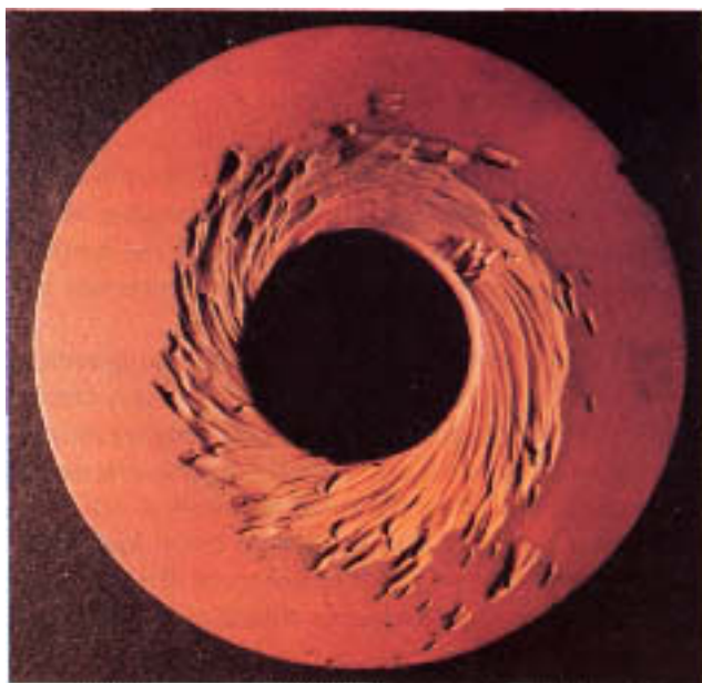
Figure 17.9 Feedwater-pump spacer eroded by turbulent high-speed water. Flow patterns are obvious.
