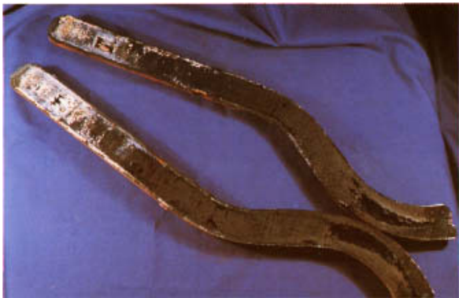
Figure 1.21 Longitudinally split stub end from a superheater outlet. The tube is plugged with deposits. The white material is sodium hydroxide and sodium carbonate concentrated at the bottom of the stub end. The black material is mostly magnetite.
