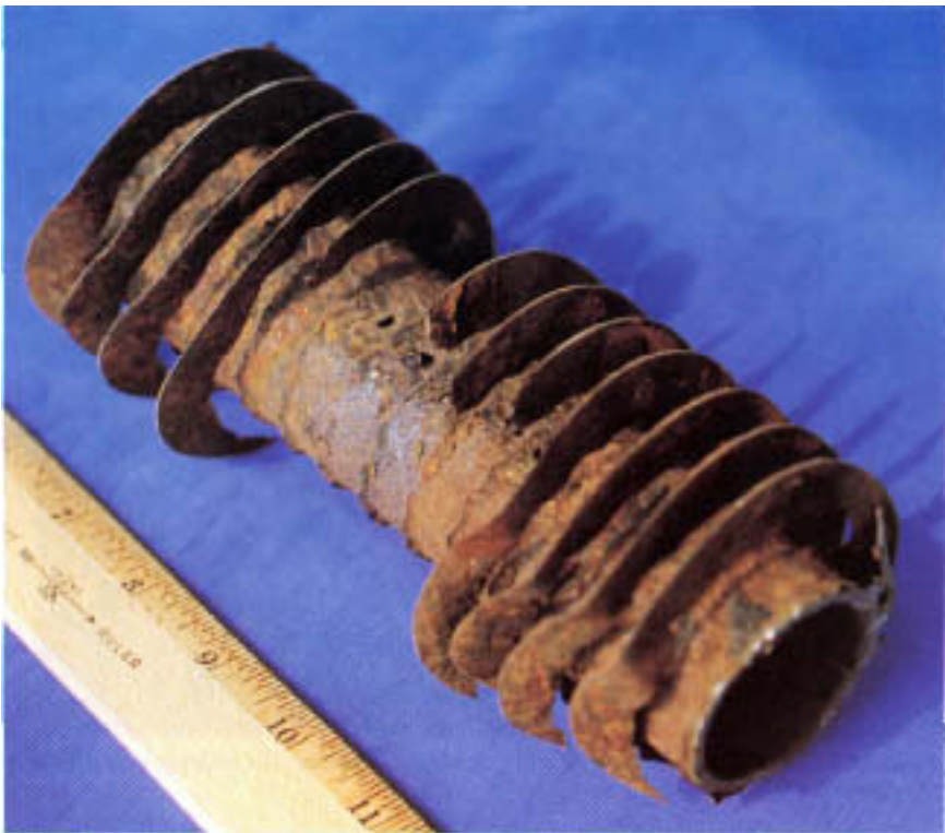
Figure 12.4 Corrosion and perforations of finned economizer tube resulting from exposure to condensed sulfuric acid. Note detachment of fins from tube wall.
