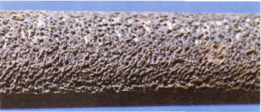
Figure 17.13 Erosion on mild steel turbine drain line. Surface is festooned with small, conical projections pointing toward the direction of impingement.
