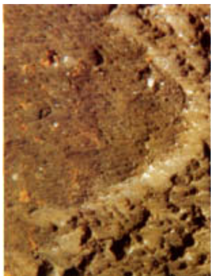
Figure 17.18 Erosion patterns at edge of wasted area. As in Fig. 17.17. Note flow patterns. (Magnification: 7.5X.)
