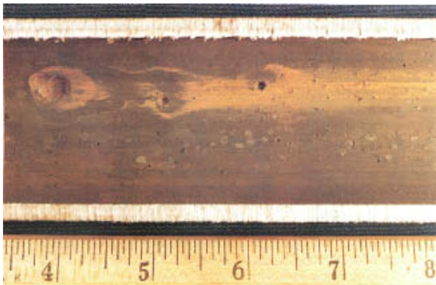
Figure 8.1 Oxygen pits in section of superheater tube. (Courtesy of Electric Power Research Institute.)
