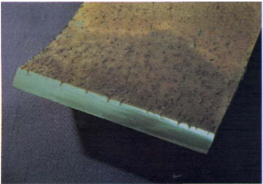
Figure 15.4 Transverse cracks originating on the internal surface.
