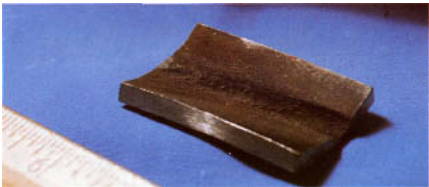
Figure 4.13 Grooved window section cut from inner bend.
