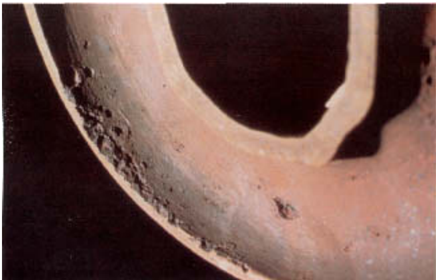
Figure 8.3 Oxygen pits along bottom of superheater pendant. (Courtesy of National Association of Corrosion Engineers.)
