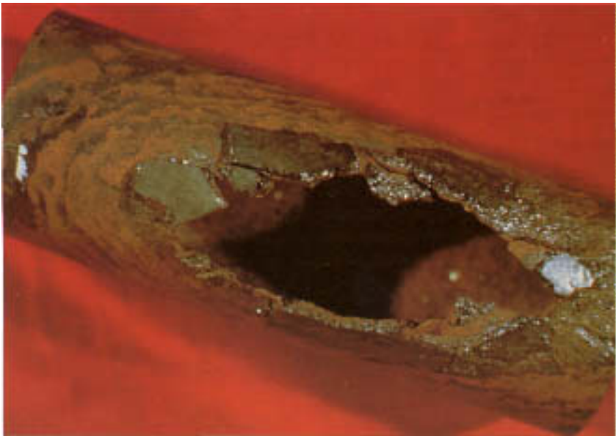
Figure 2.6 Through-wall oxidation of a tube from a low-pressure boiler. Brittle black magnetite patches still adhere to the rupture mouth. Elsewhere the oxide has spalled. Such through-wall oxidation is most common in low-pressure boilers, where internal pressures are not sufficient to cause premature failure.
