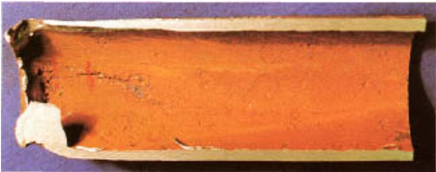
Figure 7.5 Longitudinal fissures near rolled end.
