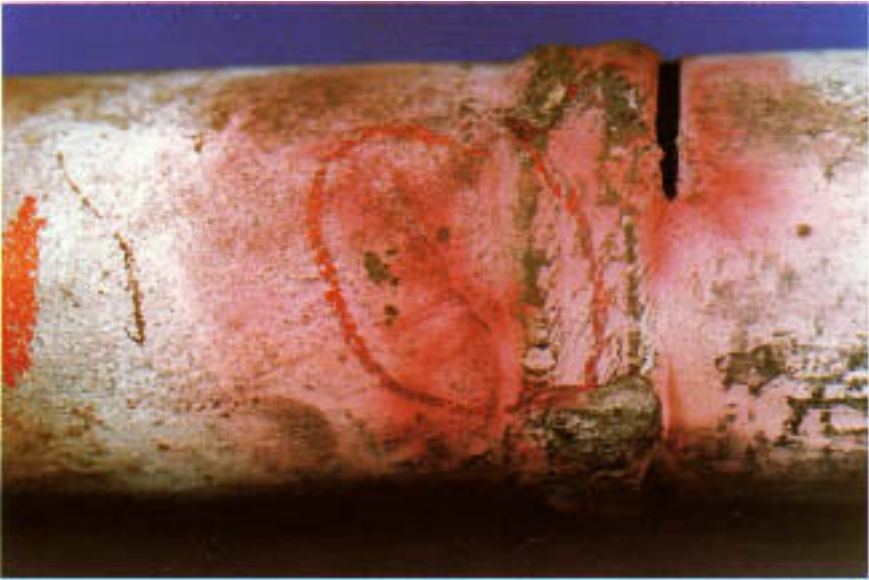
Figure 16.5 Appearance of stress-corrosion crack on the external surface. Crack is located within the red circle.
