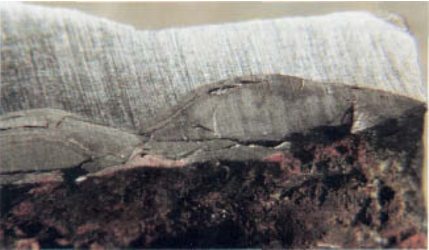
Figure 6.2 Deep gouge on internal surface. (Magnification: 7.5X.)
