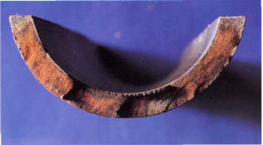
Figure 15.10 Brittle fracture face resulting from corrosion fatigue.
