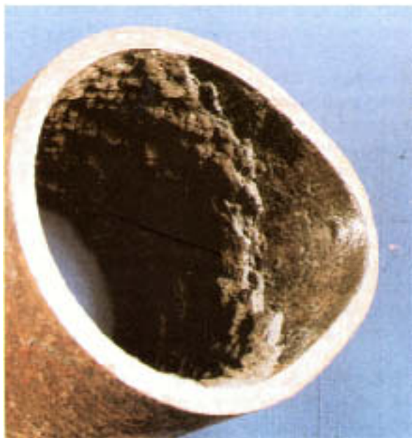
Figure 1.18 Analcite formed by carryover of alum from clarifiers. Note how the deposit has spalled from the bulge.
