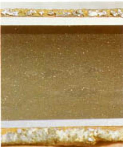
Figure 1.15 Sparkling black magnetite crystals on internal surface of a wall tube. Crystals are formed by precipitation on surfaces, or are transported from preboiler areas.
