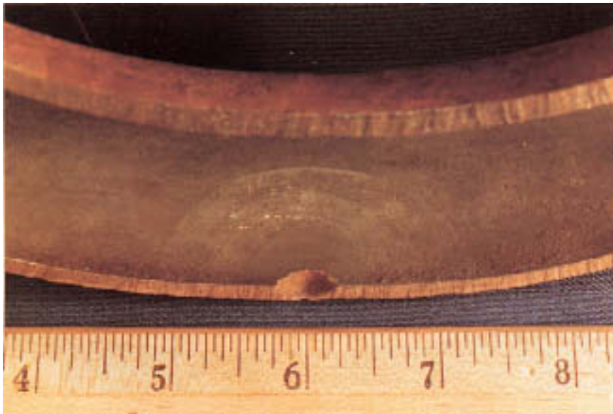
Figure 8.4 Elliptical water rings surrounding oxygen pit in a U-bend. (Courtesy of Electric Power Research Institute.)
