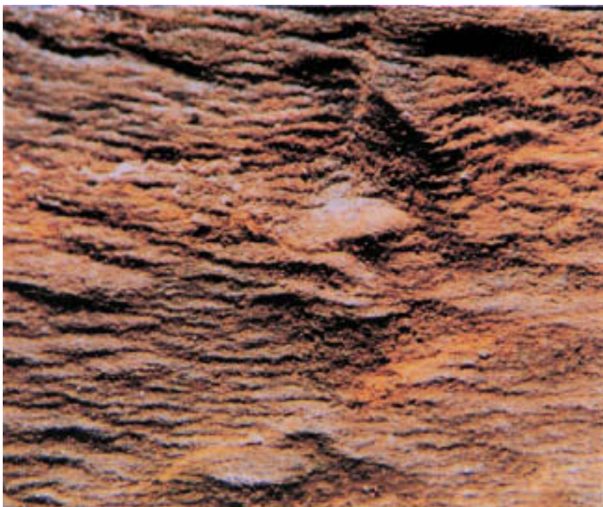
Figure 17.4 Finely spaced, wavelike, parallel undulations on eroded fire-side external surface of superheater tube. The striations resemble waves viewed from the air and are aligned perpendicularly to the direction of steam impingement. (Compare with Fig. 17.3.)
