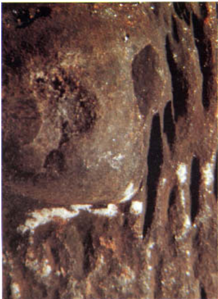
Figure 15.9 Transverse fissures near stud (center). (Magnification: 6.5X.)
