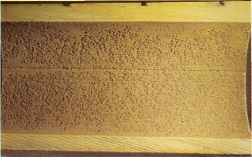
Figure 7.1 Acid corrosion on the internal surface of a wall tube. (Courtesy of Electric Power Research Institute.)
