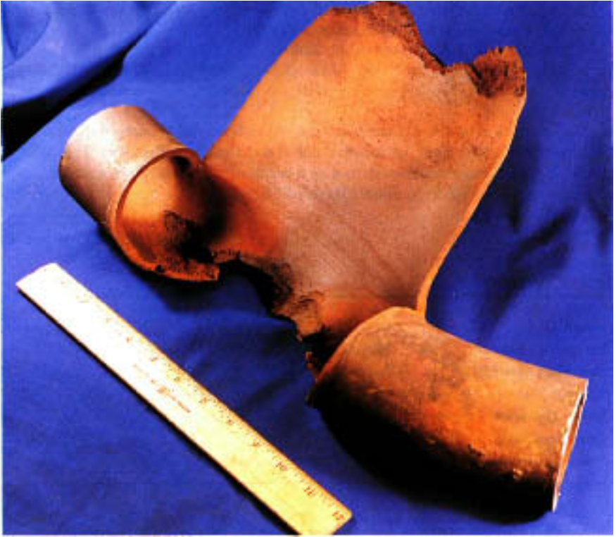
Figure 6.3 Rupture associated with low-pH gouging.
