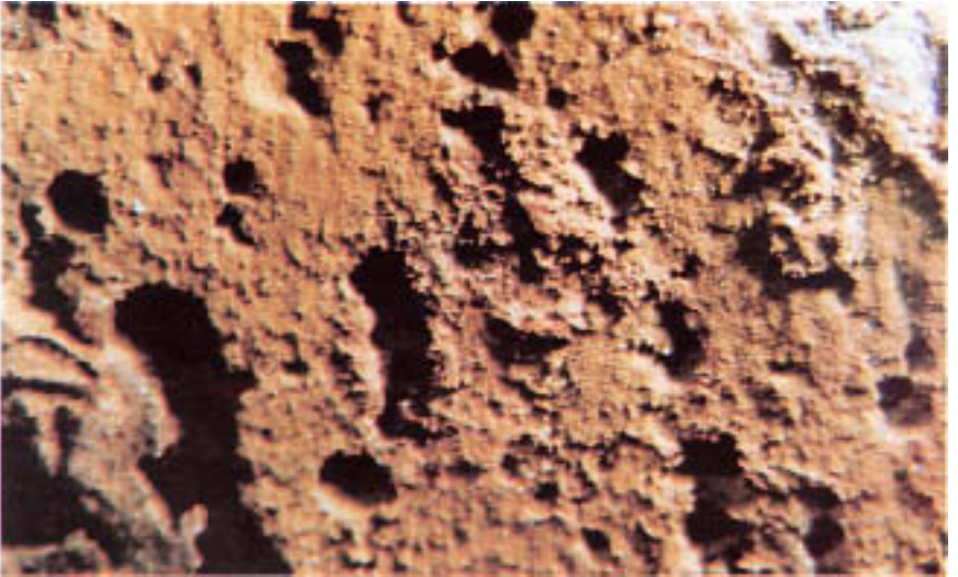
Figure 7.10 Acid corrosion along internal surface. (Magnification: 7.5X.)
