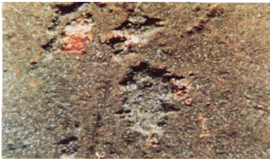
Figure 7.11 Metal loss from strong acid. (Magnification: 7.5X.)
