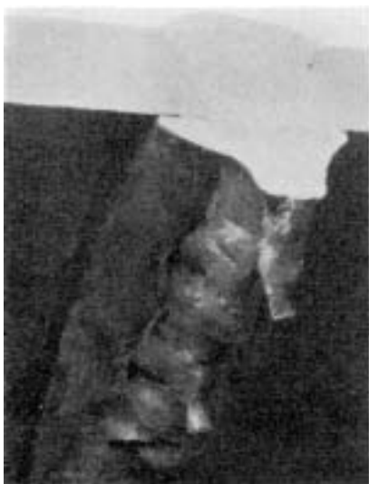
Figure 20.3 Burnthrough resulting in icicles on the underside of a butt weld. ( Reprinted with permission from Helmut Thielsch, Defects and Failures in Pressure Vessels and Piping, New York, Van Nostrand Reinhold, 1965. )
