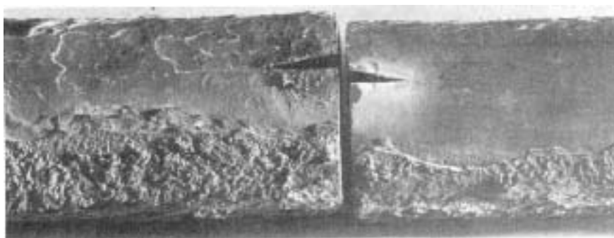
Figure 10.1 Superheater tube (ASME SA-213, grade T22) that ruptured due to thinning by coal-ash corrosion. (Reprinted with permission of American Society for Metals Handbook, vol. 10, 8th ed., Metals Park, Ohio, 1975, p. 537.)
