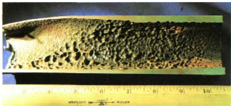
Figure 5.4 Chelant corrosion on internal surface of inlet end.
