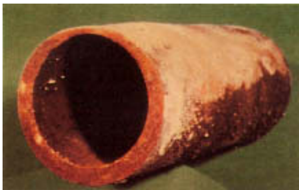
Figure 9.4 Wall thinning from oil-ash corrosion. Corrosion rates of 30 mil/y (0.76 mm/y) have been observed. (Courtesy of Electric Power Research Institute.)
