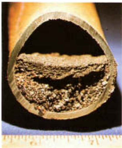
Figure 1.19 Anthracite and resin beads beneath a stratified iron oxide layer.
