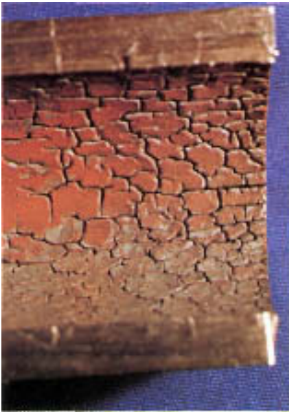
Figure 15.6 Thermal-fatigue cracks on internal surface.
