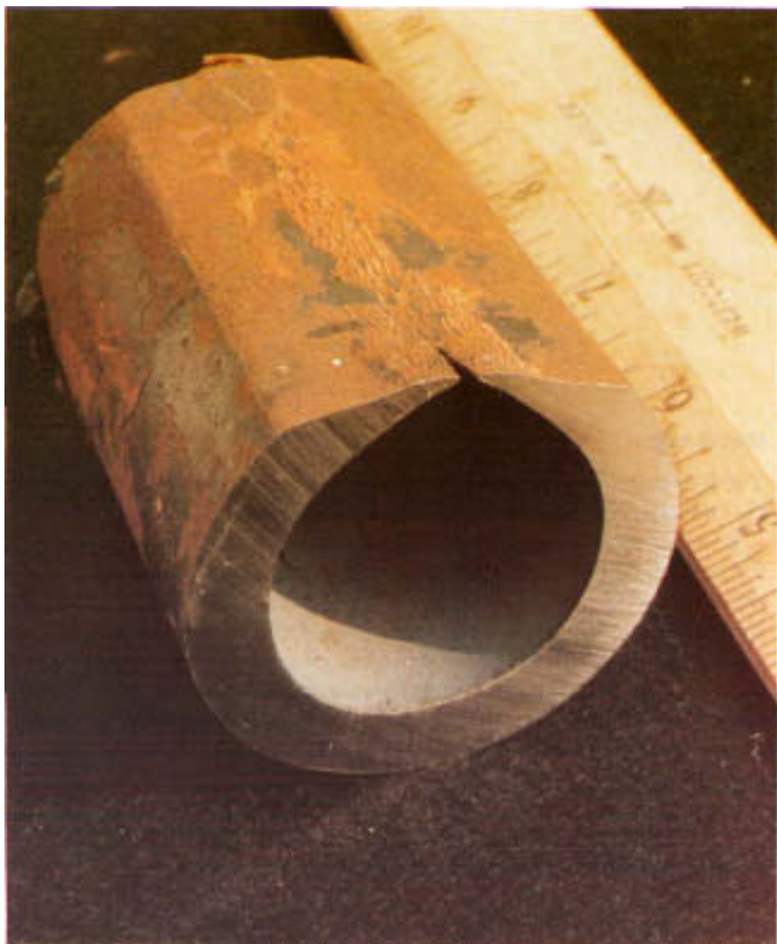
Figure 17.1 Superheater section thinned by soot-blower erosion. Note the flattened surface. The tube bulged and ruptured on the thinned side. Also, note how the eroded surface color is not dissimilar to unattacked regions, indicating intermittent attack.
