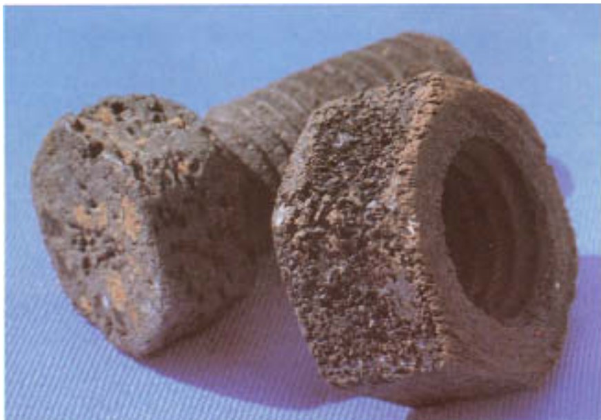
Figure 7.3 Acid corrosion of attachment hardware.
