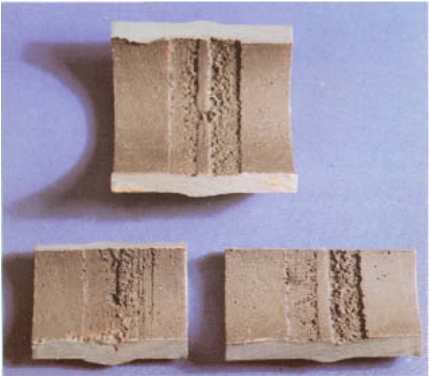
Figure 7.2 Acid corrosion at weld.
