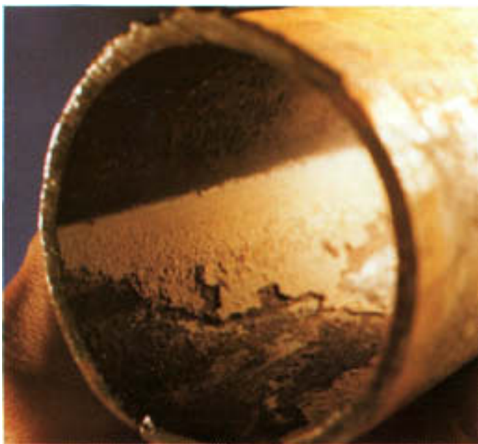
Figure 1.22 Deposit layer on the internal surface of the hot side of a crossover tube. Some deposit spalled off at a shallow bulge. Note the sharp boundaries indicating the terminus of steam blanketing.
