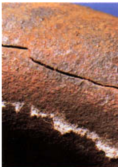
Figure 16.4 Longitudinal crack along the side of a 90° bend in an economizer tube. A similar crack is located along the opposite side.
