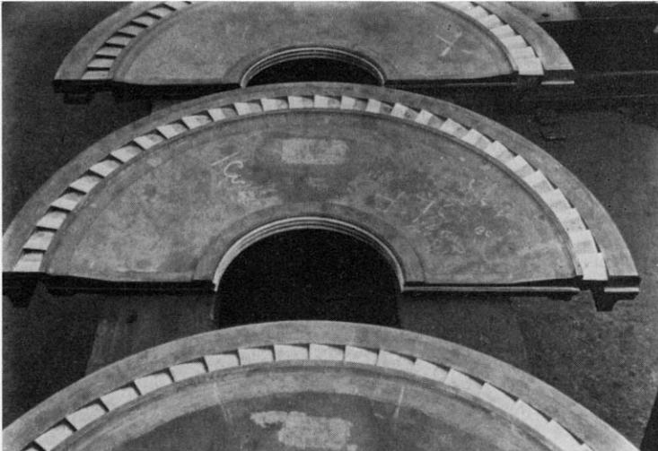
Figure 3.30 Typical half diaphragms, showing cast-in nozzle division plates, and diaphragm gland fins
