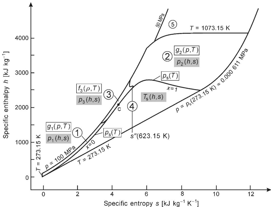
**Fig. 2.13** Assignment of the backward equations  $p(h,s)$  to the single-phase regions 1 to 3 and  $T_s(h,s)$  to that part of the two-phase region 4 with  $s \geq s''$  (623.15 K). For this overview, it is not shown how regions 2 and 3 will be divided into subregions.
