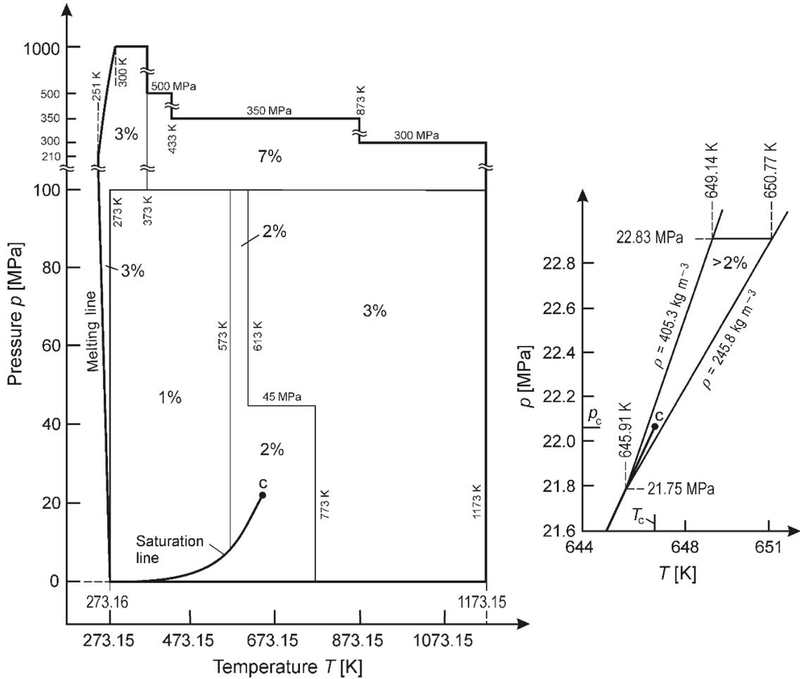
**Fig. 3.2** Percentage uncertainties in viscosity estimated for the viscosity equation, Eq. (3.1). In the near-critical region, shown in the enlarged diagram on the right, the uncertainty of Eq. (3.1) is greater than 2%. The positions of the lines separating the uncertainty regions are approximate.
