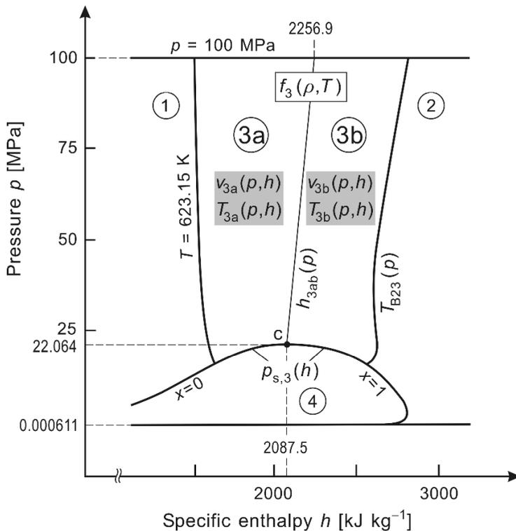
**Fig. 2.8** Division of region 3 into subregions 3a and 3b, and the assignment of the backward equations  $v(p,h)$  and  $T(p,h)$  to these subregions. The  $p$  and  $h$  values at the corner points of region 3 are given in Fig. 2.5.
