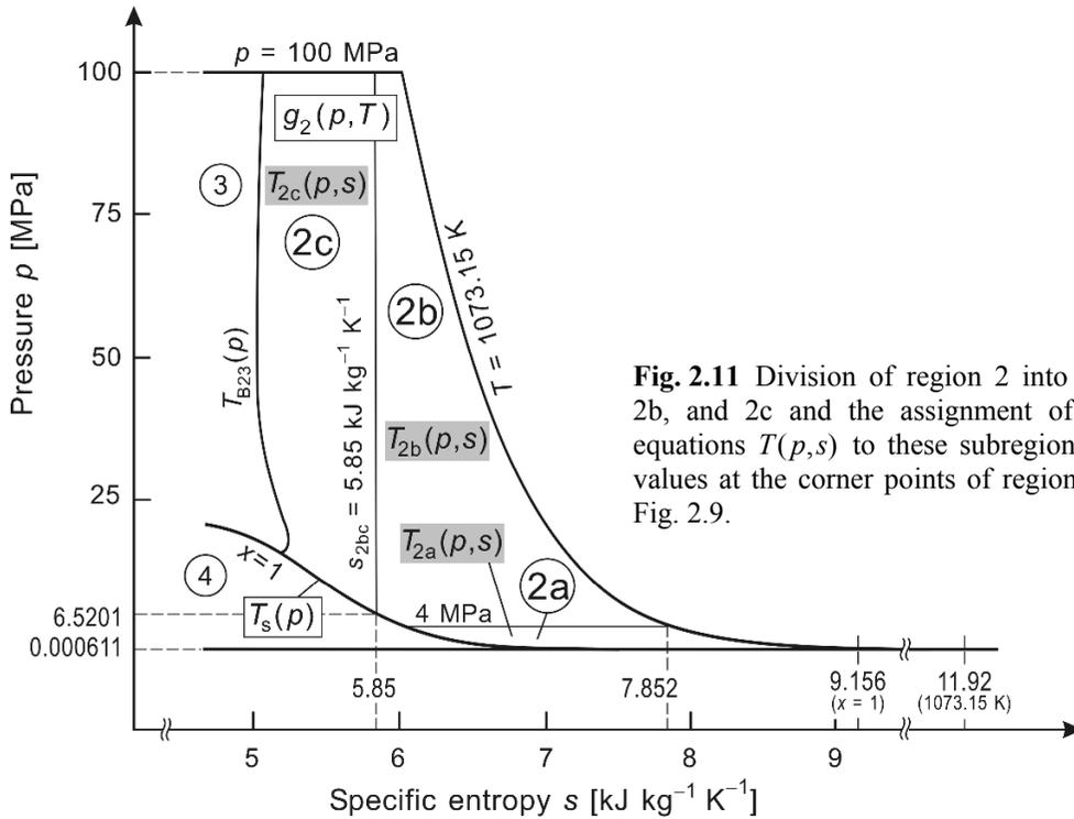
**Fig. 2.11** Division of region 2 into subregions 2a, 2b, and 2c and the assignment of the backward equations  $T(p,s)$  to these subregions. The  $p$  and  $s$  values at the corner points of region 2 are given in Fig. 2.9.
