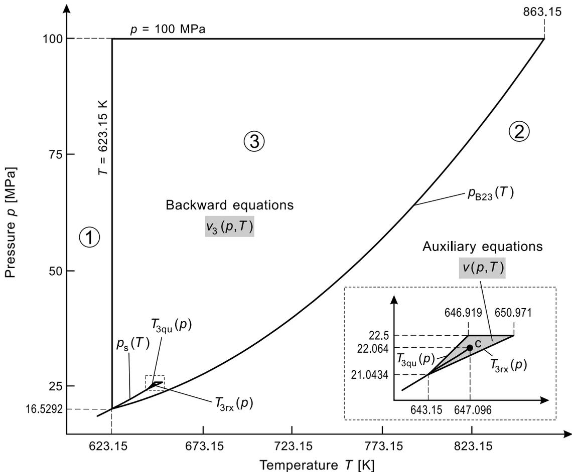
**Fig. 2.23** Range of validity of the backward equations  $v_3(p, T)$  covering all of region 3 except for the near-critical region. The near-critical region is enlarged and marked in grey in the lower right part of the figure, where this region is covered by the auxiliary equations  $v(p, T)$ . This near-critical region includes a temperature range from 643.15 K to 650.971 K at pressures from 21.0434 MPa to 22.5 MPa. Figure 2.26 shows this small region in more detail.
