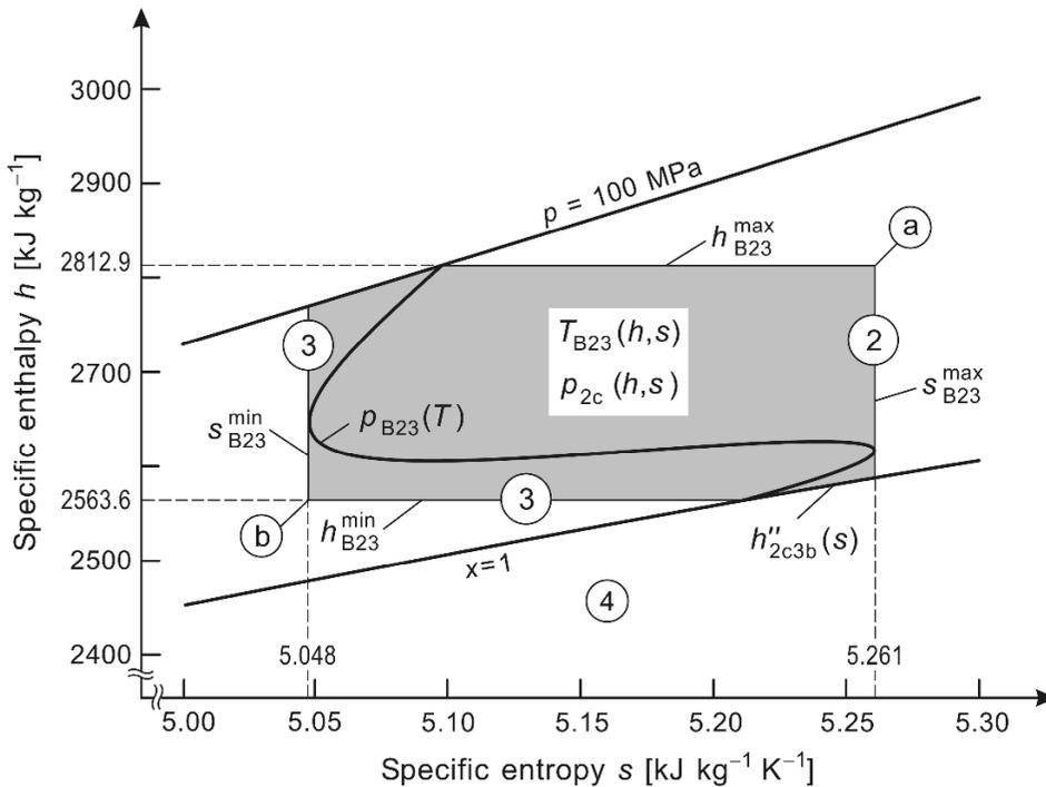
**Fig. 2.16** Plot of the equation  $p_{B23}(T)$ , Eq. (2.1), and the range of validity (grey area) of the equation  $T_{B23}(h, s)$ , Eq. (2.45), in an  $h$ - $s$  diagram. To be exact, region 2 means subregion 2c and region 3 means subregion 3b. The corner points a and b are needed to show their place in Fig. 2.17.
