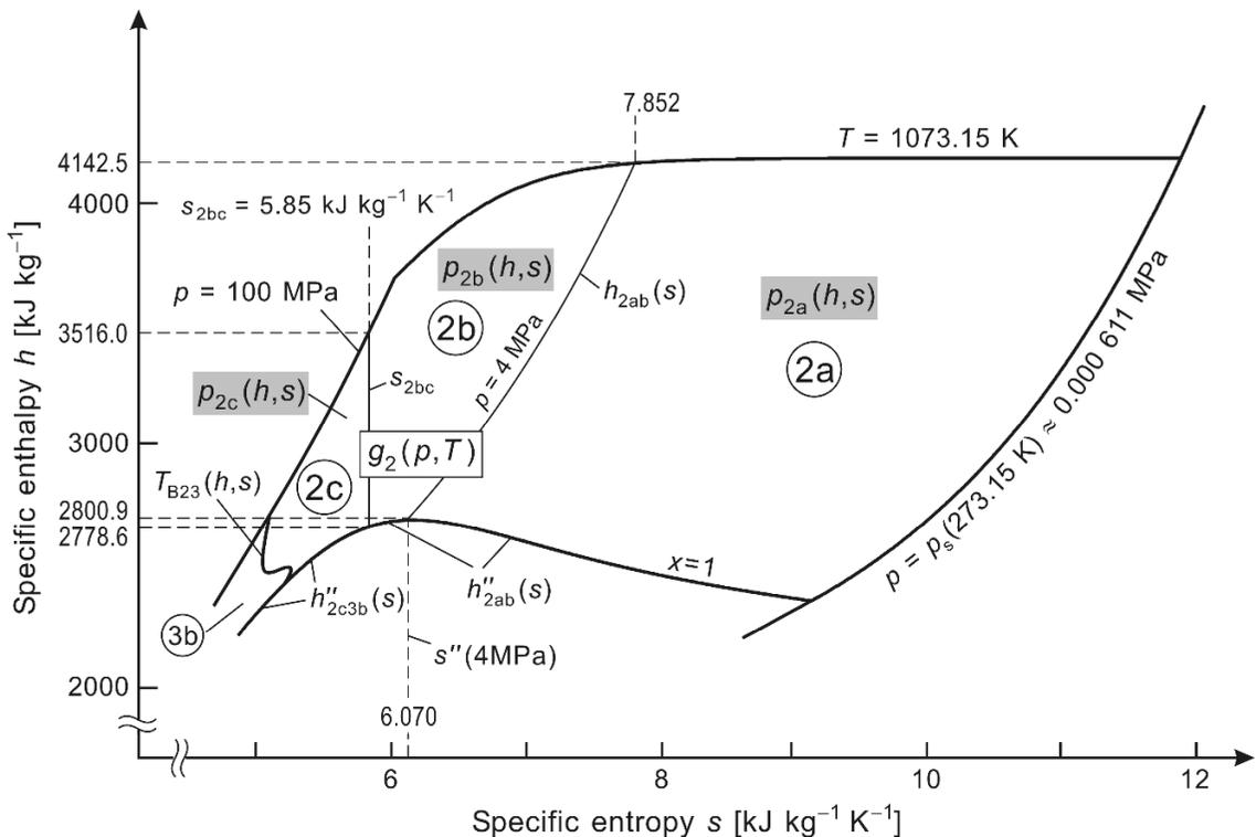
**Fig. 2.19** Division of region 2 into subregions 2a, 2b, and 2c and the assignment of the backward equations  $p(h,s)$  to these subregions. The  $h$  and  $s$  values at the corner points of region 2 are given in Fig. 2.14.
