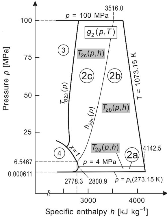
**Fig. 2.7** Division of region 2 into subregions 2a, 2b, and 2c and the assignment of the backward equations  $T(p, h)$  to these subregions. The  $p$  and  $h$  values at the corner points of region 2 are given in Fig. 2.5.
