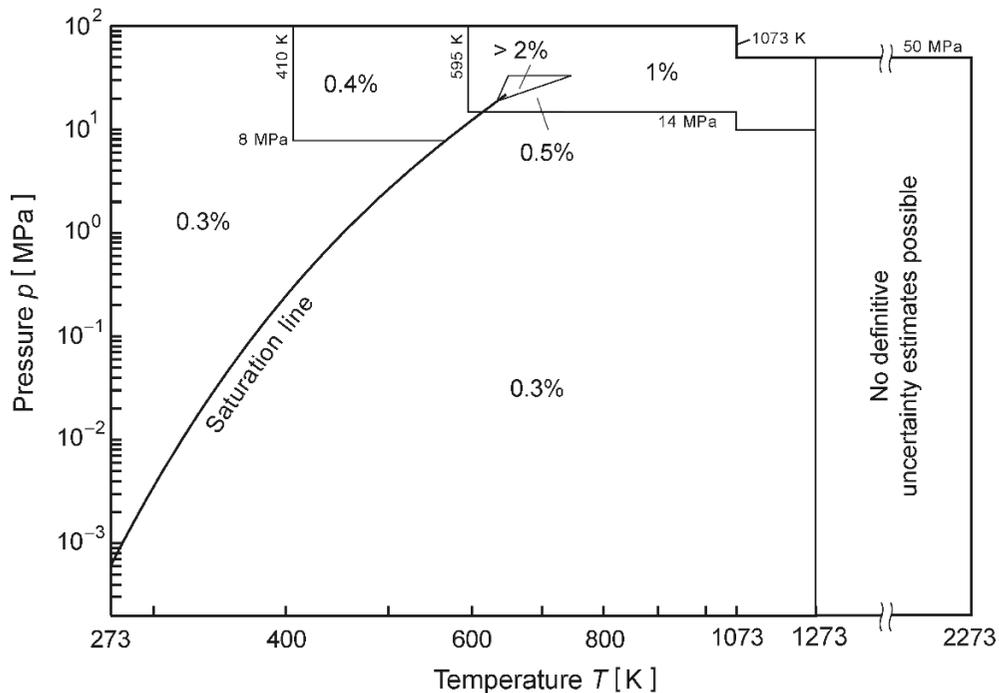
**Fig. 2.29** Percentage uncertainties in speed of sound estimated for the basic equations for regions 1 to 3 and 5 of IAPWS-IF97. The definition of the triangle showing the enlarged critical region is given in Fig. 2.27. The positions of the lines separating the uncertainty regions are approximate.
