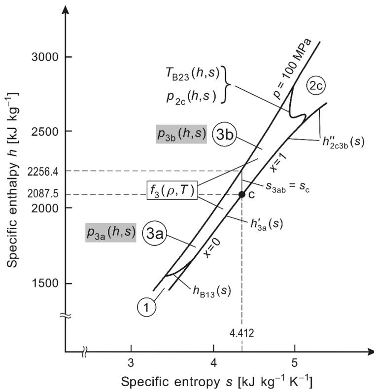
**Fig. 2.20** Division of region 3 into subregions 3a and 3b, and the assignment of backward equations  $p_{3a}(h, s)$  and  $p_{3b}(h, s)$  to these subregions. The  $h$  and  $s$  values at the corner points of region 3 are given in Fig. 2.14.
