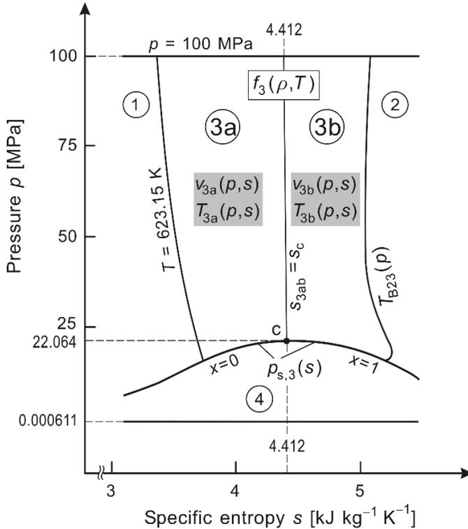
**Fig. 2.12** Division of region 3 into subregions 3a and 3b, and the assignment of backward equations  $v(p,s)$  and  $T(p,s)$  to these subregions. The  $p$  and  $s$  values at the corner points of region 3 are given in Fig. 2.9.
