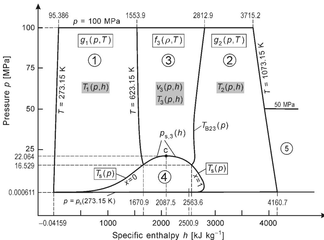
**Fig. 2.5** Regions and region boundaries of IAPWS-IF97 for the variables ( $p,h$ ). Assignment of the backward equations  $T(p,h)$  and  $v(p,h)$  to these regions (without showing how regions 2 and 3 will be divided into subregions). The  $p$  and  $h$  values given at the corner points of the region boundaries are rounded values.
