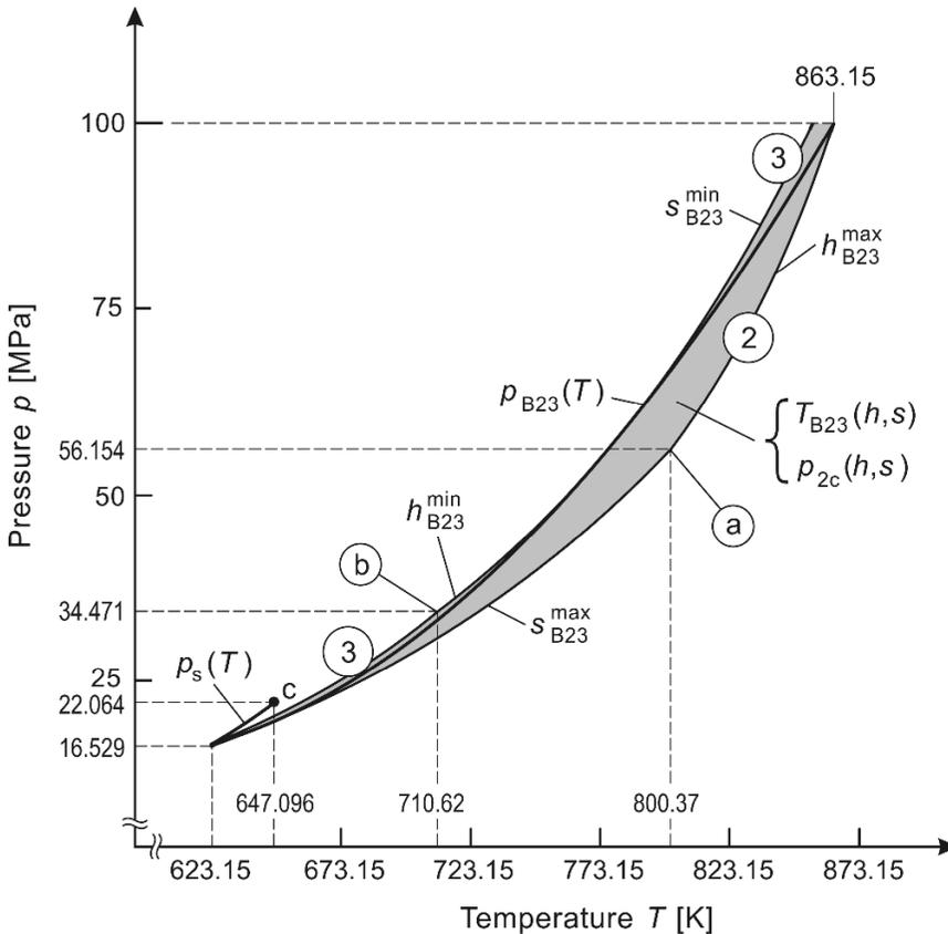
**Fig. 2.17** Illustration of the B23-equation  $p_{B23}(T)$ , Eq. (2.1), and the range of validity of the boundary equation  $T_{B23}(h, s)$ , Eq. (2.45), in a  $p$ - $T$  diagram. To be exact, region 2 means subregion 2c and region 3 means subregion 3b.
