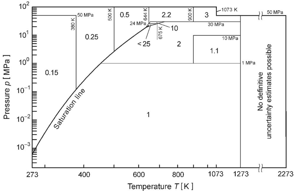
**Fig. 2.31** Absolute uncertainties  $\Delta h$  in  $\text{kJ kg}^{-1}$  in specific enthalpy  $h$  estimated for the basic equations for regions 1 to 3 and 5 of IAPWS-IF97. The definition of the triangle showing the enlarged critical region is given in Fig. 2.27. The positions of the lines separating the uncertainty regions are approximate.
