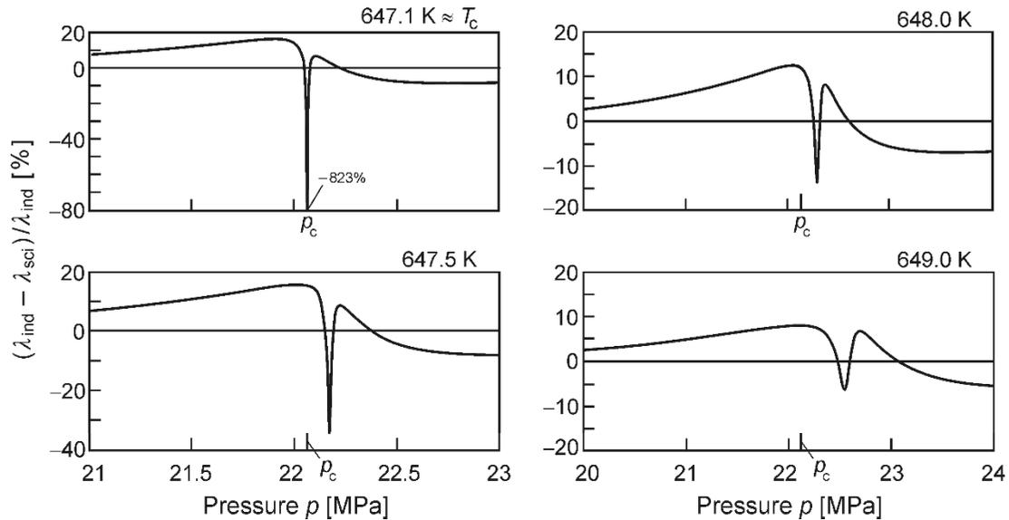
**Fig. 3.5** Percentage differences between values for the thermal conductivity  $\lambda$  in the critical region calculated from the equation for industrial use, Eq. (3.4), and values determined from the equation for scientific use [35].
