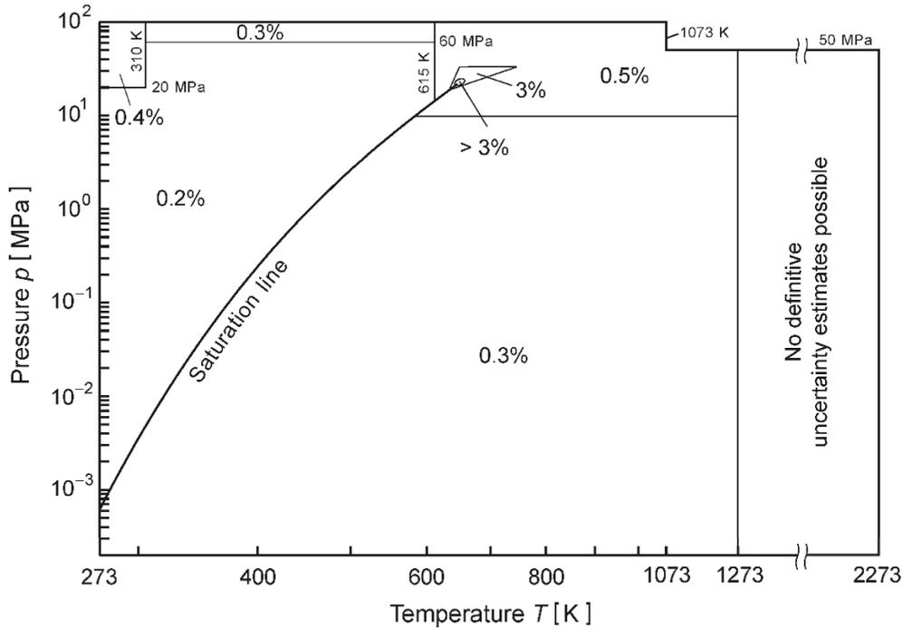
**Fig. 2.28** Percentage uncertainties in specific isobaric heat capacity estimated for the basic equations for regions 1 to 3 and 5 of IAPWS-IF97. The definition of the triangle showing the enlarged critical region is given in Fig. 2.27. The positions of the lines separating the uncertainty regions are approximate.
