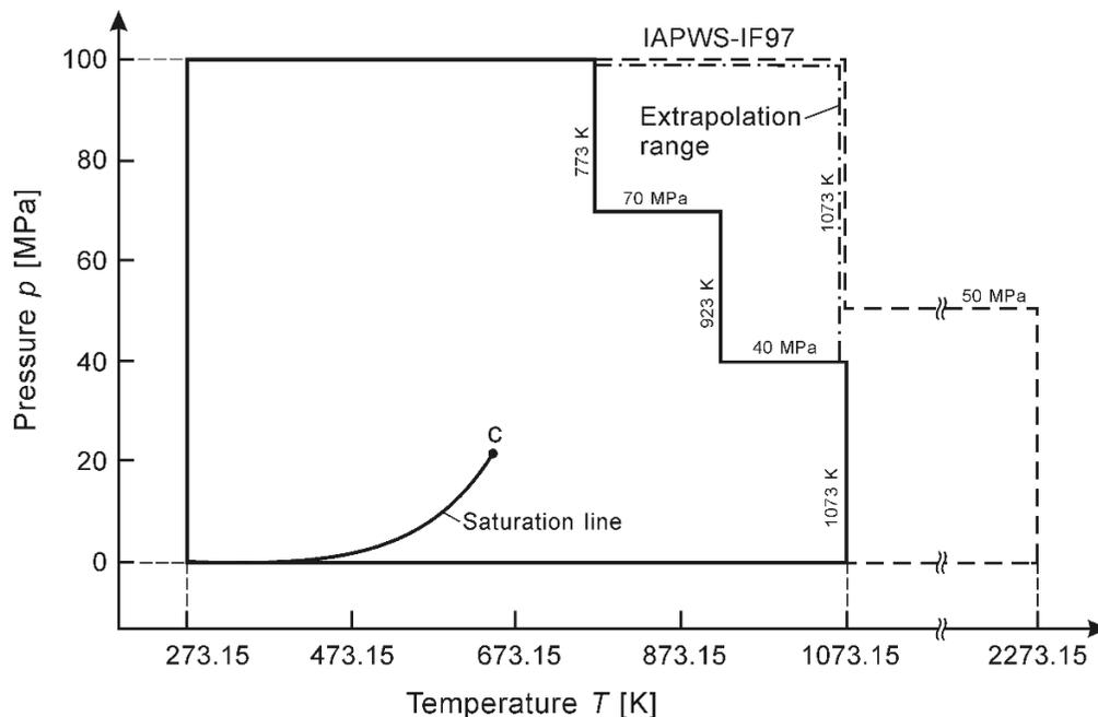
**Fig. 3.3** Range of validity of the thermal-conductivity equation for industrial use, Eq. (3.4). The greater validity range of IAPWS-IF97 shown by the dashed lines is plotted for comparison. The extrapolation range of Eq. 3.4 is illustrated by the dashed-dotted line, see next page.
