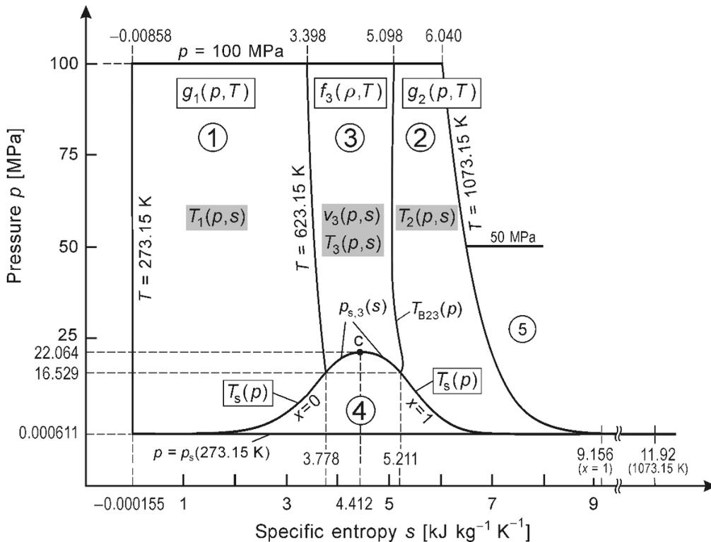
**Fig. 2.9** Regions and region boundaries of IAPWS-IF97 for the variables ( $p,s$ ). Assignment of the backward equations  $T(p,s)$  and  $v(p,s)$  to these regions, (without showing how regions 2 and 3 will be divided into subregions). The  $p$  and  $s$  values at the corner points of the region boundaries are rounded values.
