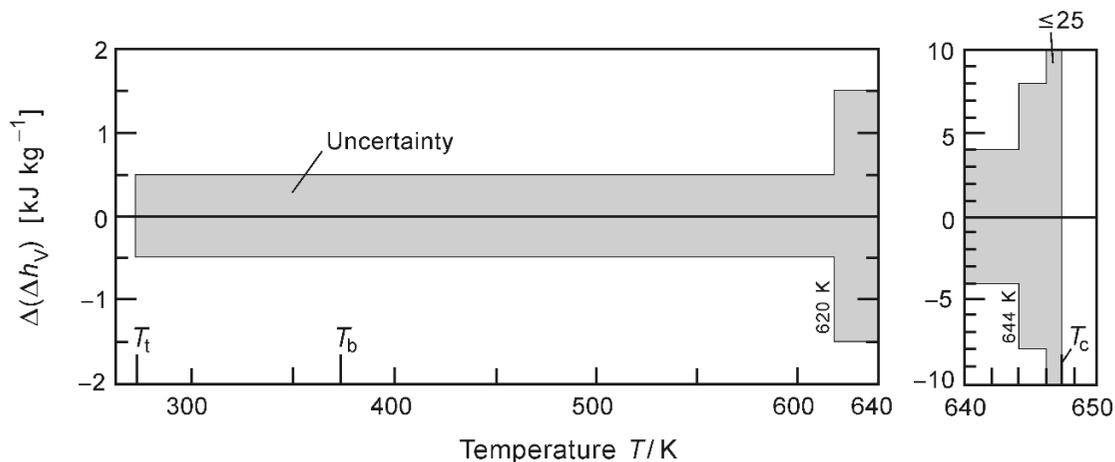
**Fig. 2.34** Absolute uncertainties  $\Delta(\Delta h_v)$  in enthalpy of vaporization  $\Delta h_v$  estimated for the basic equations for regions 1 to 3 and 5 of IAPWS-IF97. These uncertainty values only correspond to temperatures  $273.15 \text{ K} \leq T \leq 647 \text{ K}$  ( $T_c = 647.096 \text{ K}$  according to Eq. (1.4)).
