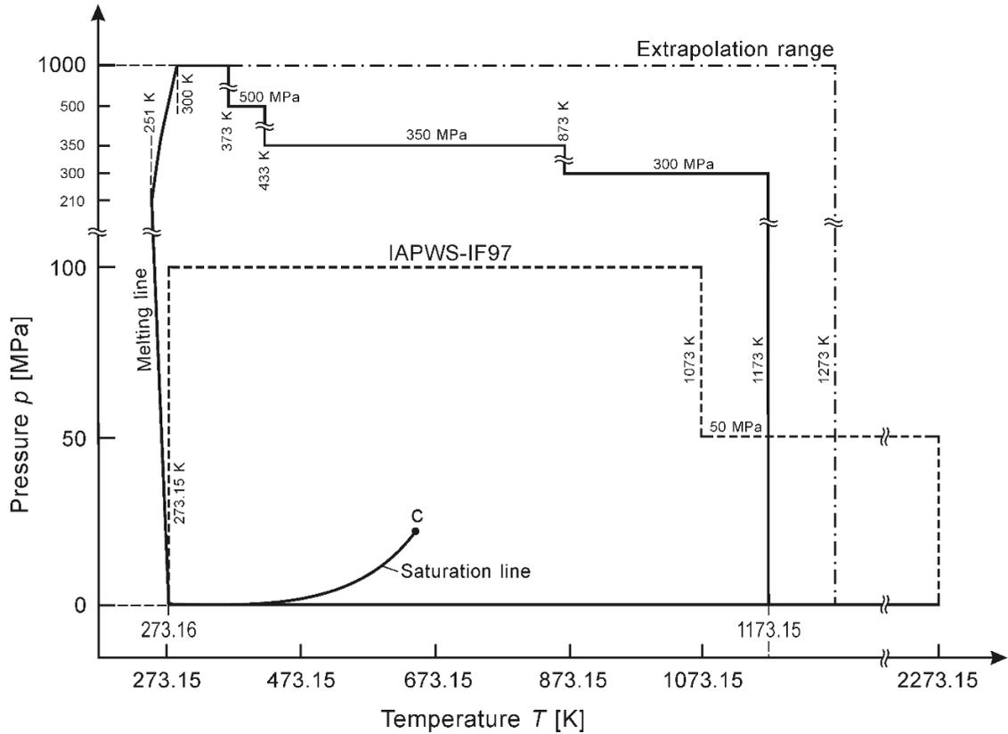
**Fig. 3.1** Range of validity of the viscosity equation for industrial applications, Eq. (3.1); its extrapolation range is given by dashed-dotted lines. The validity range of IAPWS-IF97 shown by dashed lines is plotted for comparison.
