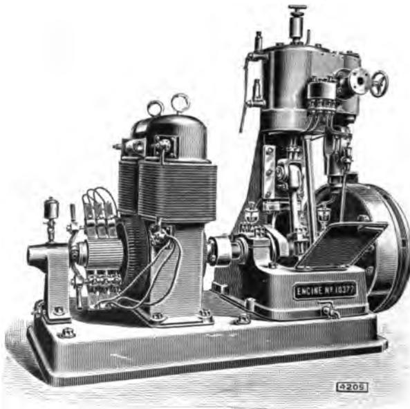
FIG. 32.—RANSOMES' SINGLE CYLINDER "OPEN" TYPE ENGINE (COUPLED DIRECT TO DYNAMO), FITTED WITH AUTOMATIC EXPANSION SHAFT GOVERNOR.
