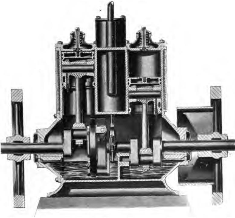
FIG. 63.—"SENTINEL" CLASS "C" SIMPLE ENGINE—LONGITUDINAL SECTION THROUGH CRANK SHAFT.
