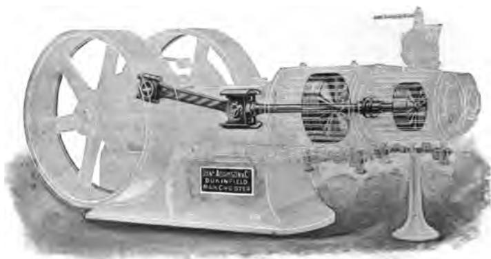
FIG. 93.—"IDEAL" ENGINE—VIEW SHOWING WATER PACKING, PISTONS, SLIPPER AND CONNECTING ROD.
