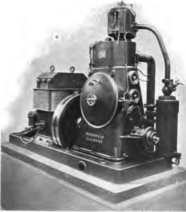
FIG. 153.—THE " SISSON " COMPOUND ENGINE, SHOWN DIRECTLY CONNECTED TO A " CLARKE-CHAPMAN " DYNAMO.
