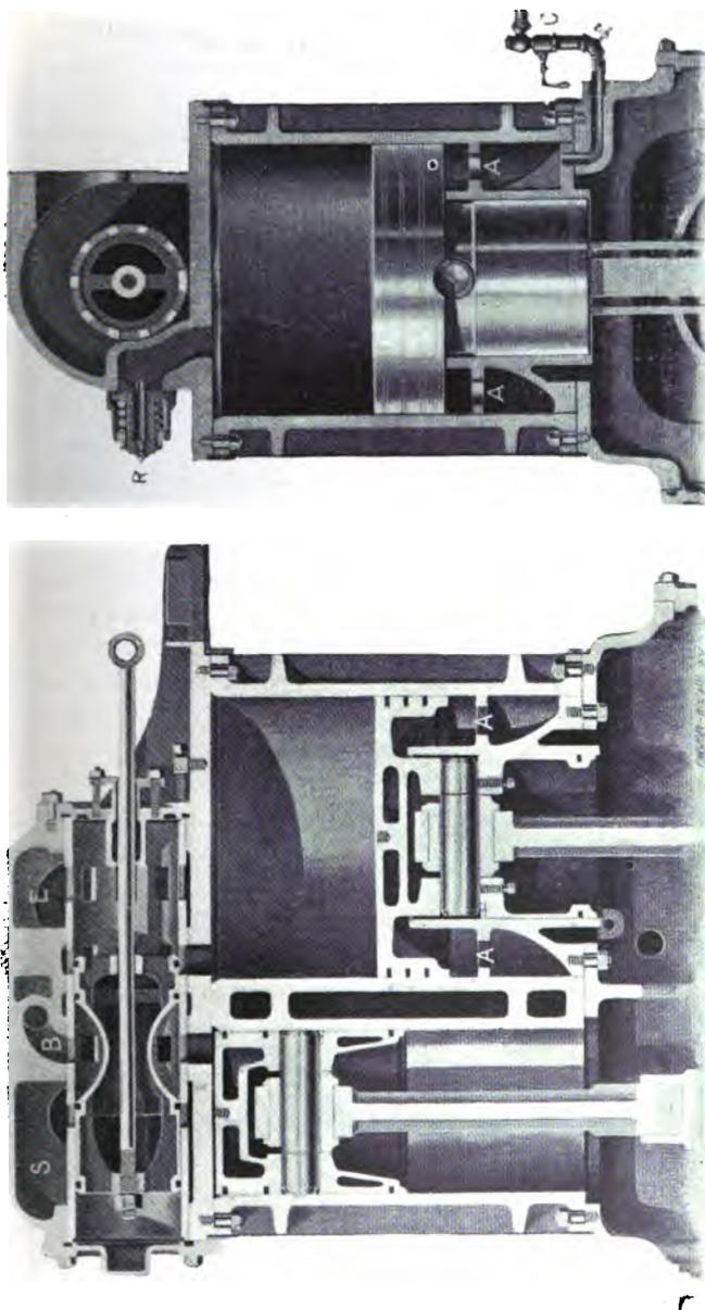
FIG. 83.—DETAIL OF CYLINDERS, PISTONS, STEAM CHEST AND VALVES.
