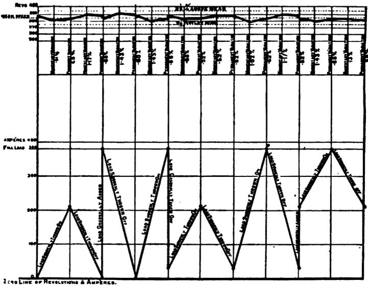
FIG. 8.—"BELLISS" PATENT SELF-LUBRICATING ELECTRIC TRACTION SET, FITTED WITH THROTTLE VALVE GOVERNOR DIAGRAM SHOWING GRAPHICALLY THE RESULTS OF SWITCHING ON AND OFF VARIOUS LOADS. IT WILL BE SEEN THAT WHEN THE LOAD IS SUDDENLY THROWN OFF OR ON, THE VARIATION OF SPEED FROM THE MEAN DOES NOT EXCEED 3 TO 4 PER CENT. PERMANENT, AND 2 PER CENT. MOMENTARY.
