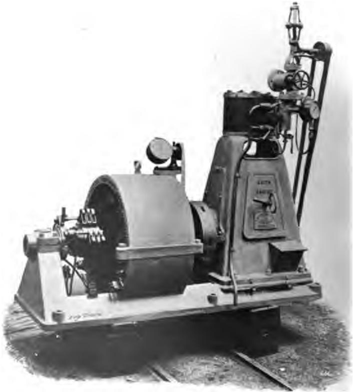
FIG. 18.—SINGLE CYLINDER "ERITH" ENGINE, COUPLED TO FOUR-POLE DYNAMO.
