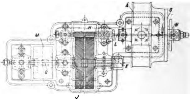
FIGS. 114 AND 115.—SECTIONAL VIEWS OF A 20 P.H.P. "DE LAVAL" MOTOR TURBINE.
