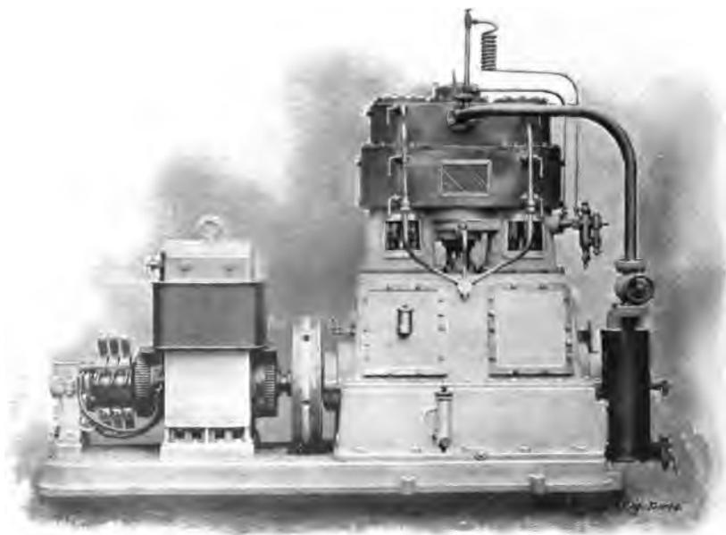
FIG. 60.—THE "RESTLER" ENGINE, COUPLED TO DYNAMO.
