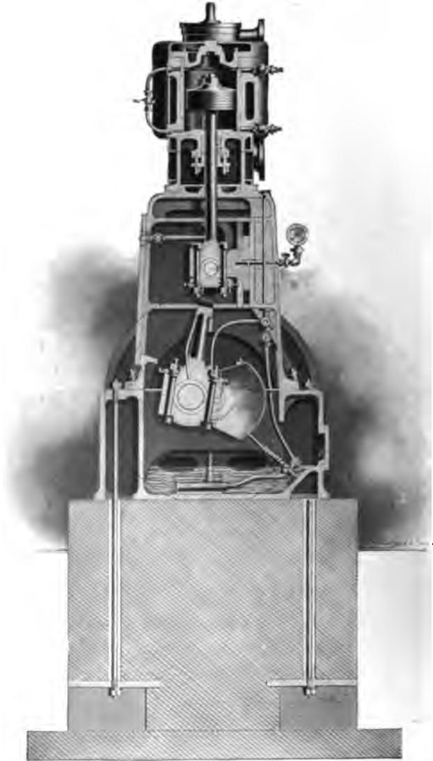
FIG 11.—SECTIONAL END VIEW OF "B.L." QUICK SPEED ENGINE.
