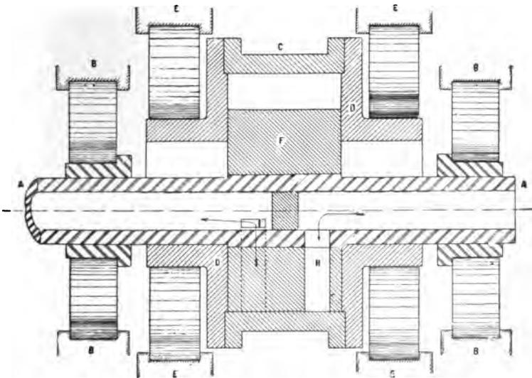
FIG. 133.—FRONT SECTIONAL VIEW OF THE “HULT” ROTARY ENGINE.
