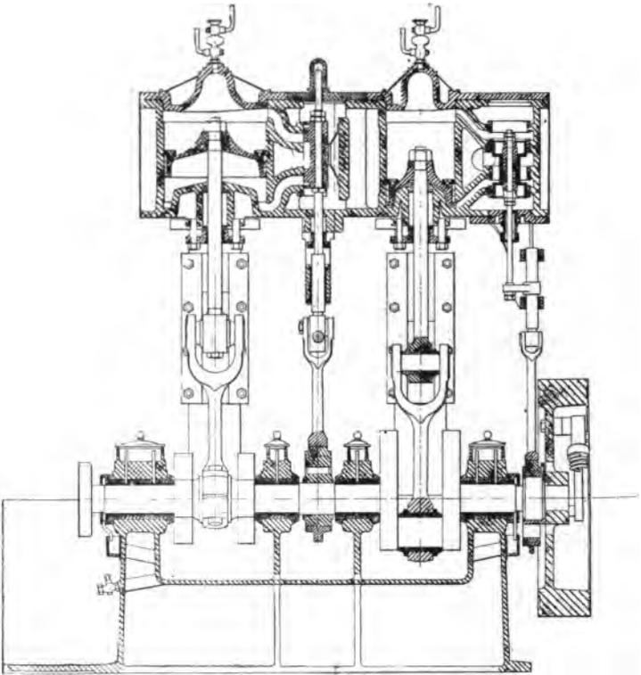
FIG. 125.—SECTIONAL VIEW OF THUNE'S DOUBLE-ACTING COMPOUND ENGINE.
