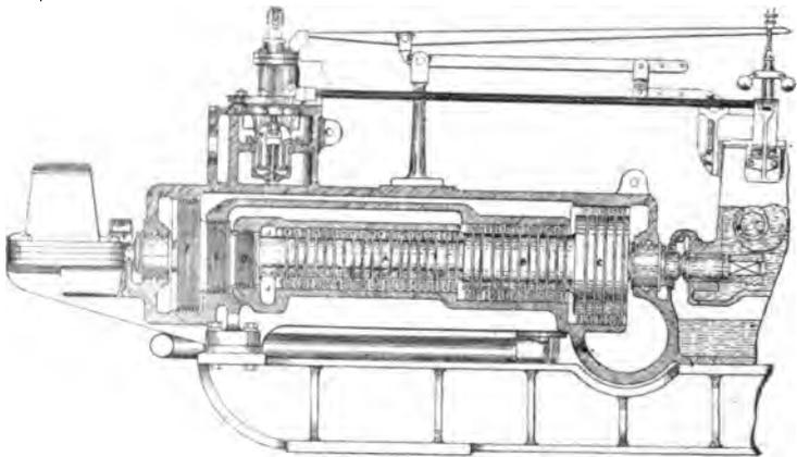
FIG. 109.—SECTIONAL VIEW OF PARSONS' STEAM TURBINE.
