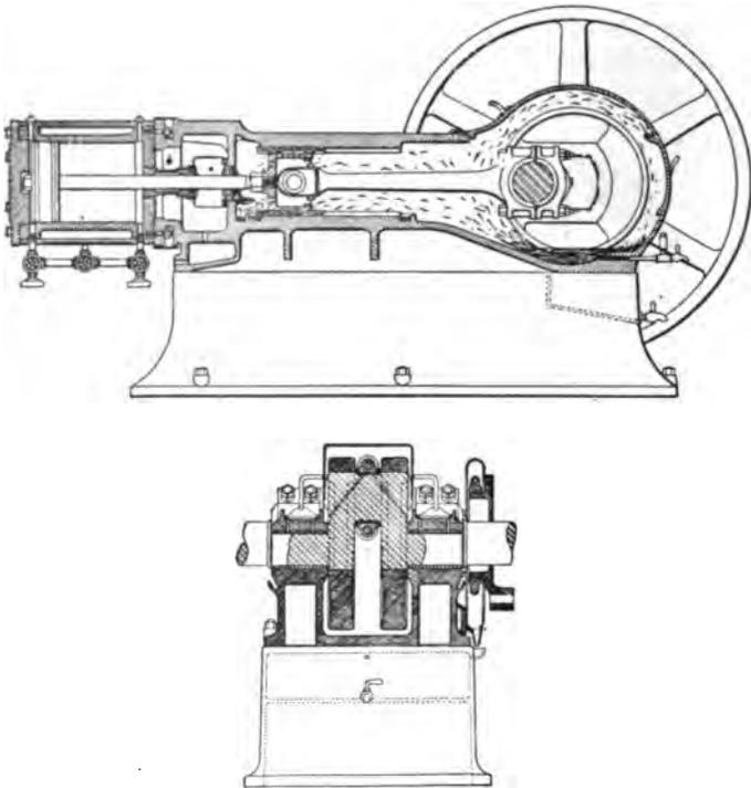
FIGS. 95 AND 96.—SECTIONAL VIEWS OF THE HARRISBURG "IDEAL" SIMPLE ENGINE.
