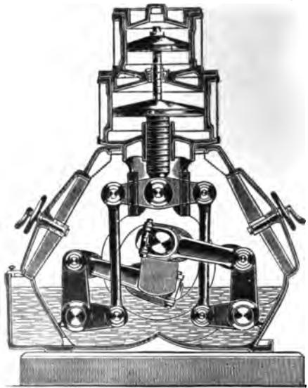
FIG. 123.—SECTIONAL VIEW OF MERTZ'S SINGLE-ACTING ENGINE.
