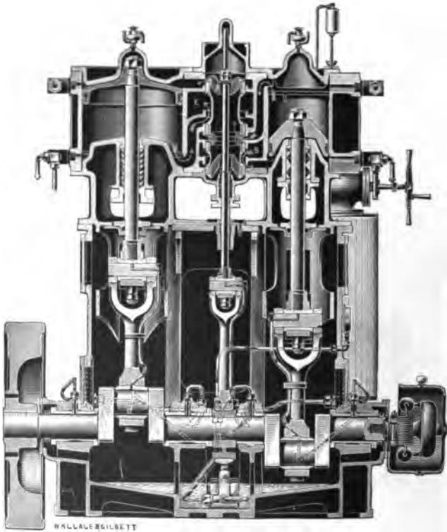
FIG. 6.—"BELLISS" ENGINE. SECTIONAL ELEVATION.
