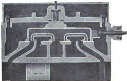
FIG. 101.—"RUSSELL" ENGINE—PART SECTIONAL PLAN THROUGH CYLINDER AND STEAM CHEST.
