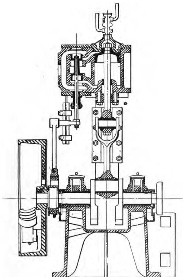
FIG. 126.—SECTIONAL VIEW OF THUNE'S DOUBLE ACTING SINGLE CYLINDER ENGINE.
