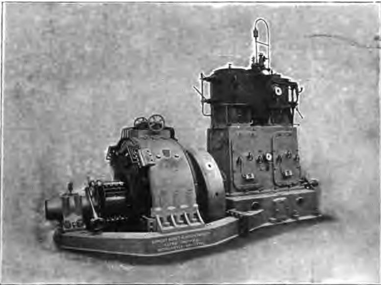
FIG. 29.—ERNEST SCOTT AND MOUNTAIN'S COMPOUND CENTRAL VALVE ENGINE, WITH DYNAMO COMBINED.
