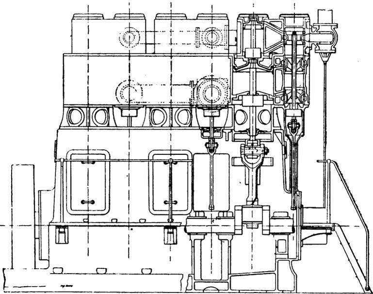
FIG. 15.—PART SECTIONAL ELEVATION OF THREE-CRANK "CLAYTON" ENGINE.
