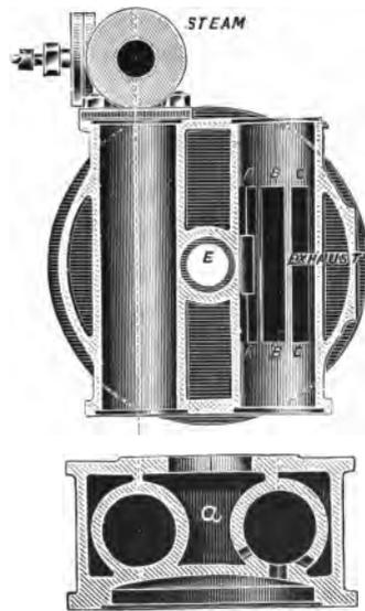
FIG. 48.—VALVE CHEST OF "UNIVERSAL" ENGINE.
