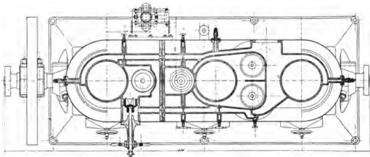
FIG. 119.—SECTIONAL PLAN OF MERTZ'S ENGINE.
