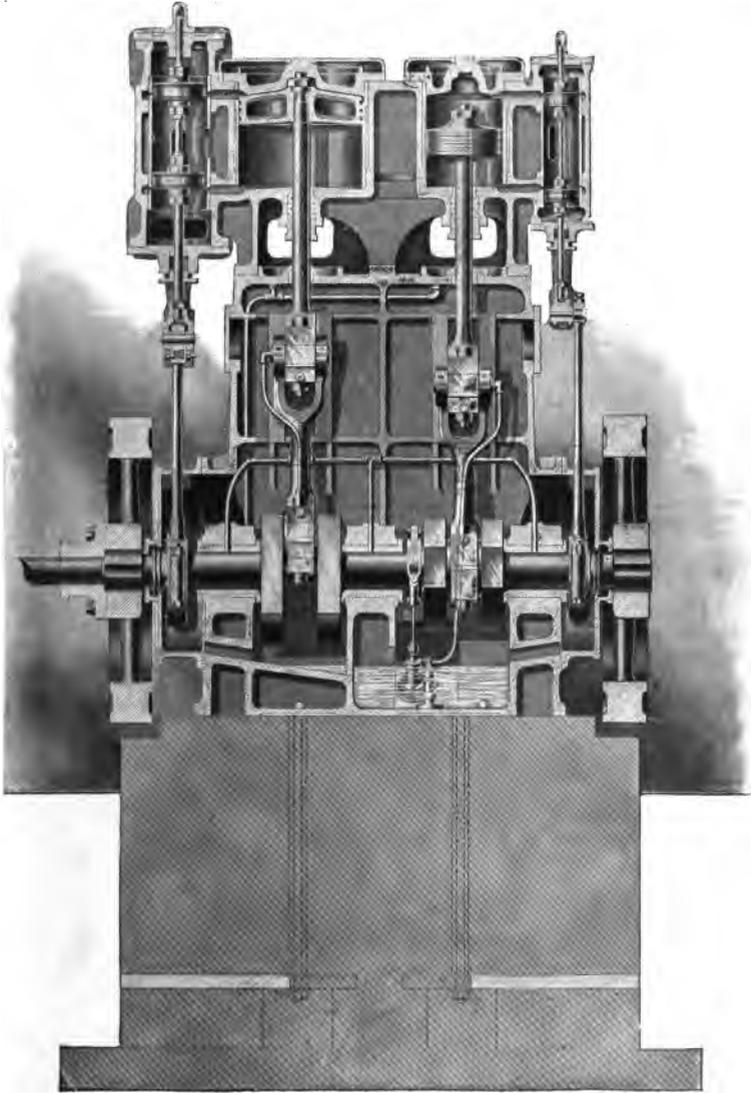
FIG. 10.—SECTIONAL VIEW OF "B.I." QUICK SPEED ENGINE.
