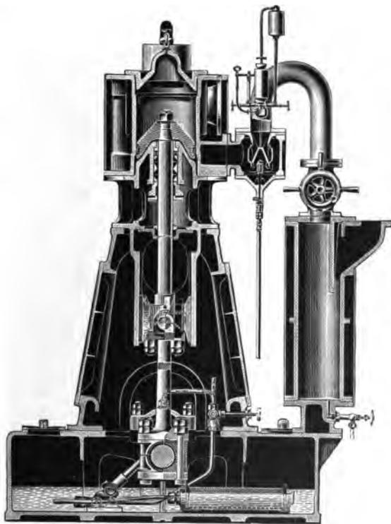
FIG. 7.—"BELLISS" ENGINE. SECTIONAL END ELEVATION.
