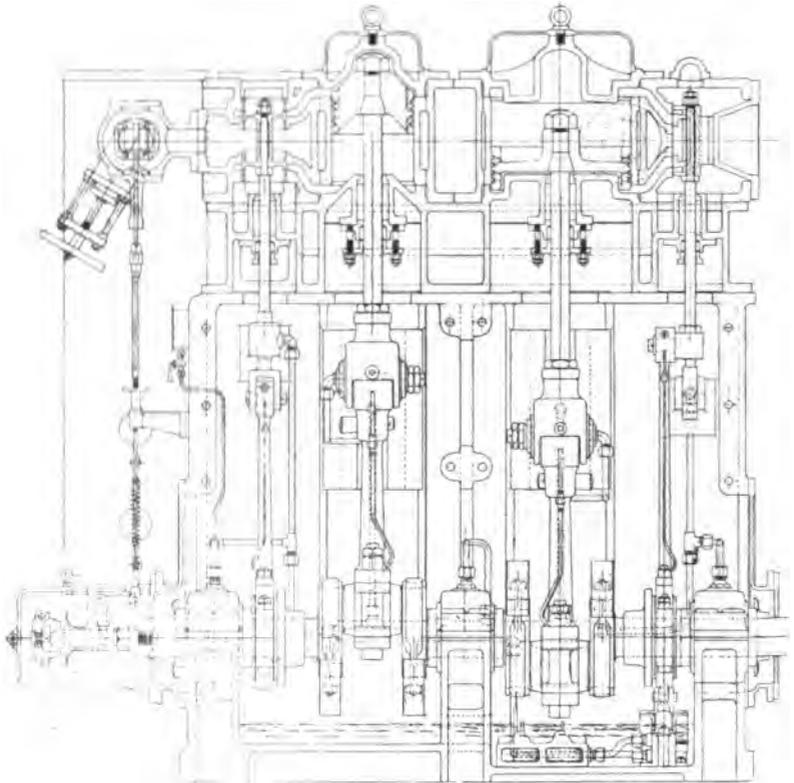
FIG. 146.—SECTIONAL VIEW OF MESSRS. ROBEY & CO.'S COMPOUND ENCLOSED, FORCED LUBRICATION ENGINE.
