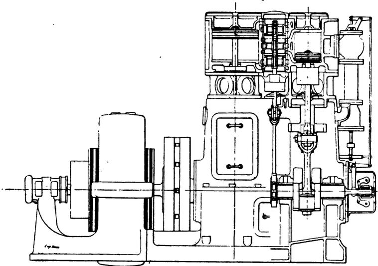
FIG. 14.—PART SECTIONAL ELEVATION OF COMPOUND "CLAYTON" ENGINE.
