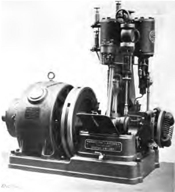
FIG. 155.—OPEN TYPE HIGH SPEED ENGINE, BY MESSRS. RANSOMES, SIMS AND JEFFERIES, LIMITED, SHOWN COUPLED TO DYNAMO.
