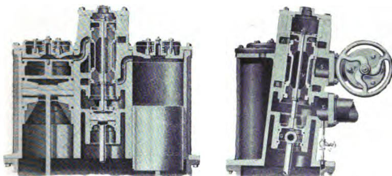
FIG. 81.—DETAIL, SHOWING CYLINDERS, PISTONS, STEAM CHEST AND VALVE.
