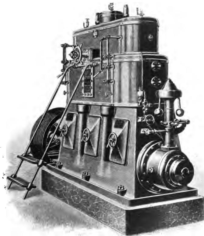
FIG. 121.—MERTZ'S COMPOUND ENGINE.
