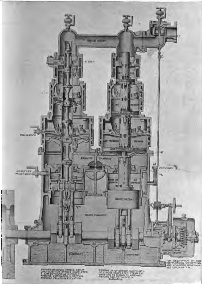
FIG. 4.—SECTIONAL VIEW OF THE "WILLANS" STANDARD PATTERN ENGINE.
