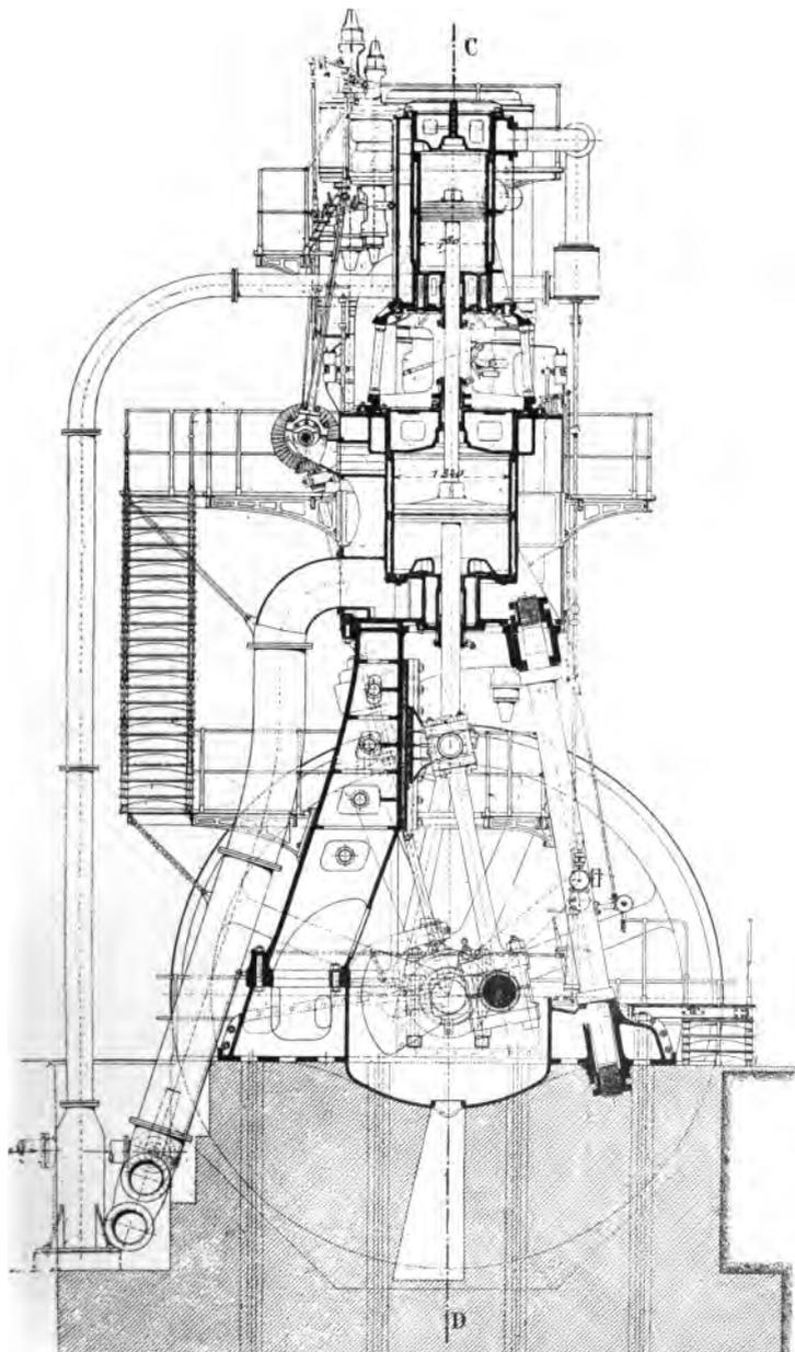
FIG. 129.—END SECTIONAL VIEW OF TRIPLE-EXPANSION FOUR-CYLINDER “ BORSIG ” ENGINE, DEVELOPING 2,500 H.P.
