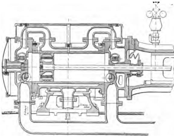
FIG. 127.—SECTION OF "FARCOT" ENGINE CYLINDER.
