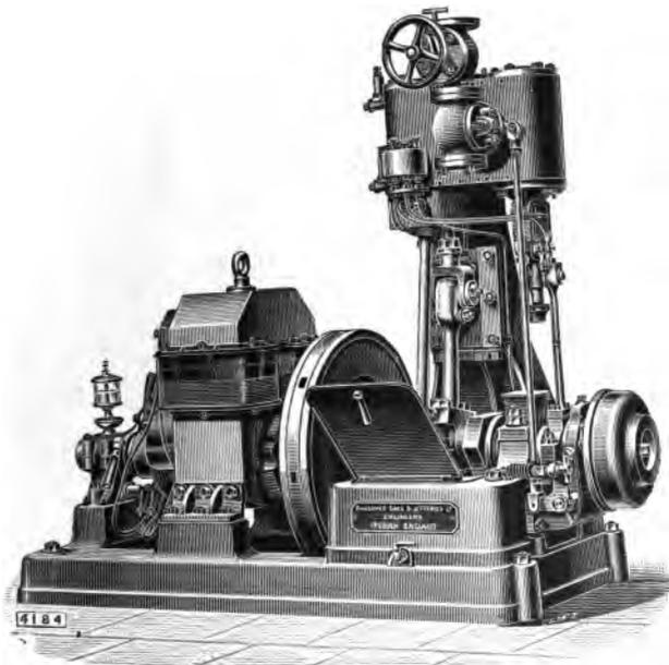
FIG. 33.—RANSOMES' ENGINE (COUPLED TO DYNAMO), FITTED WITH CRANK SHAFT THROTTLE VALVE GOVERNOR.
