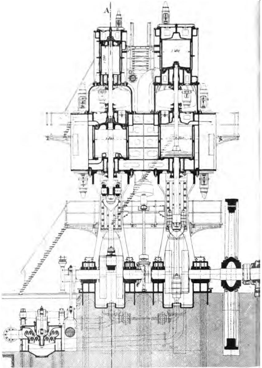
FIG. 128.—FRONT SECTIONAL VIEW OF 2,500 H.P. "BORSIG" ENGINE.
