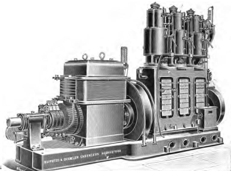
FIG. 69.—THE "CHANDLER" COMPOUND ENGINE.
