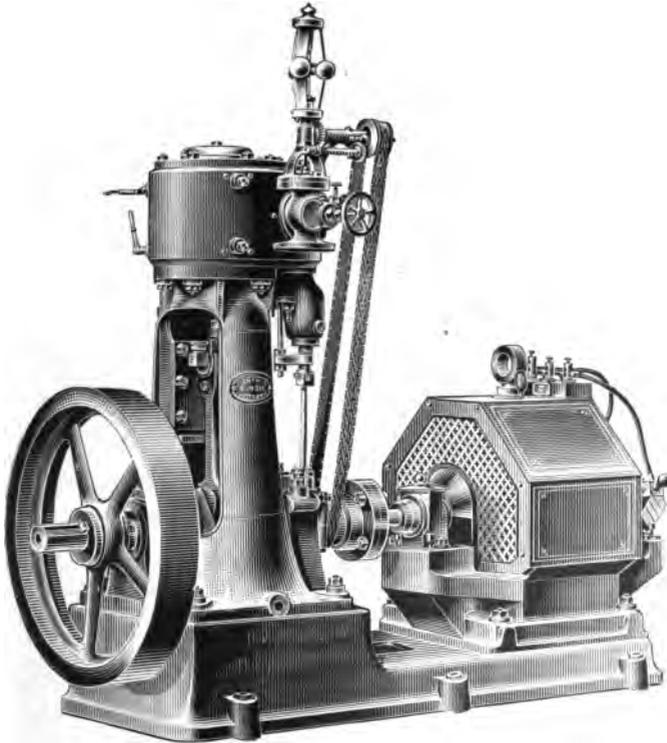
FIG. 72.—“DONKIN & CLENCH” ENGINE COUPLED TO DYNAMO.
