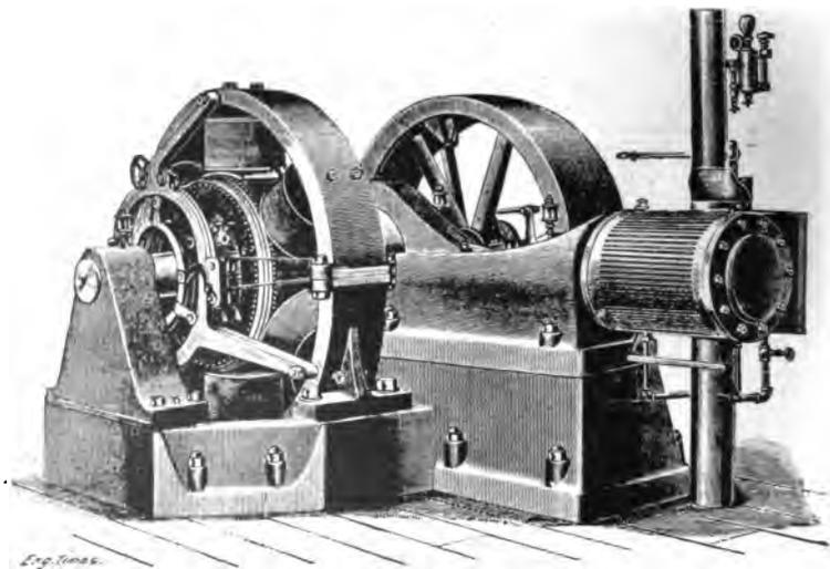
FIG. 106.—THE "ROBB ARMSTRONG" DIRECT CONNECTED ENGINE AND DYNAMO.
