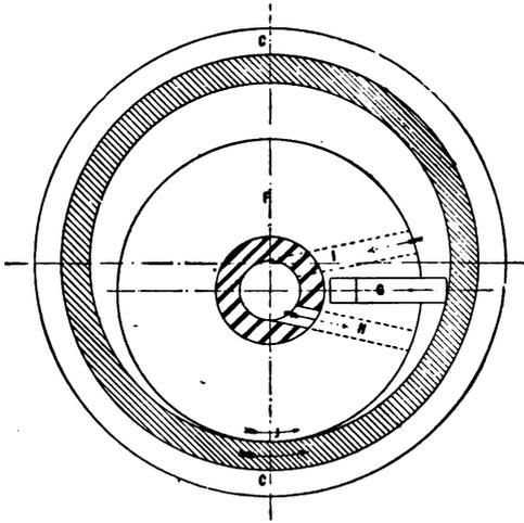
FIG. 132.—END SECTIONAL VIEW, “HULT” ROTARY ENGINE.
