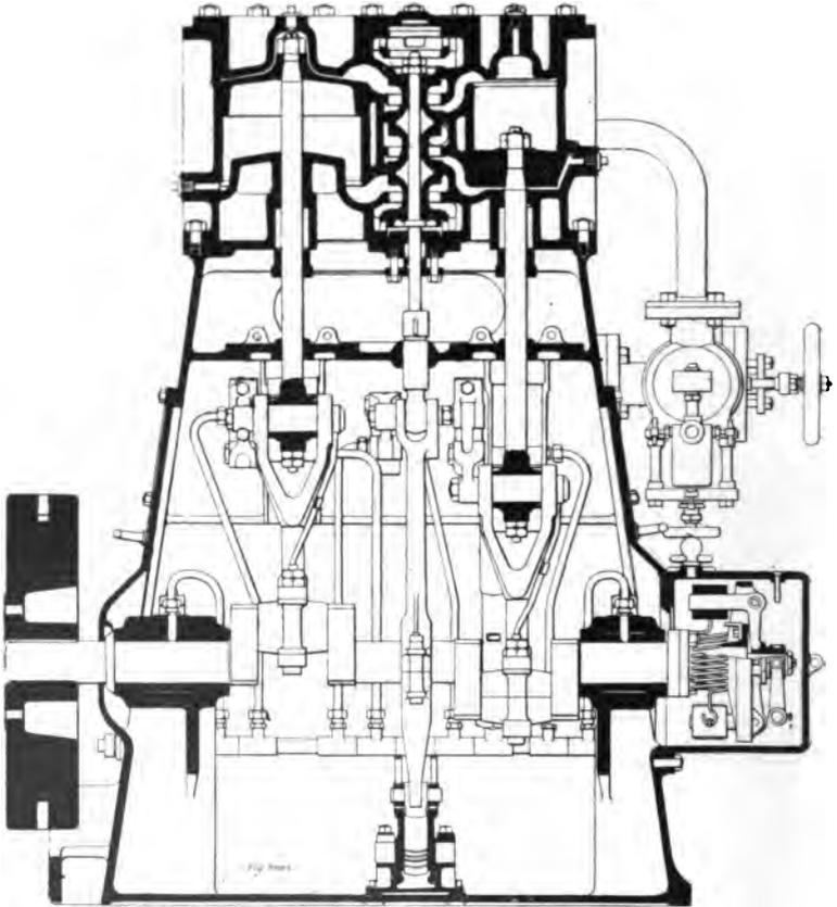
FIG. 20.—SECTIONAL ELEVATION OF "ERITH" COMPOUND ENGINE.
