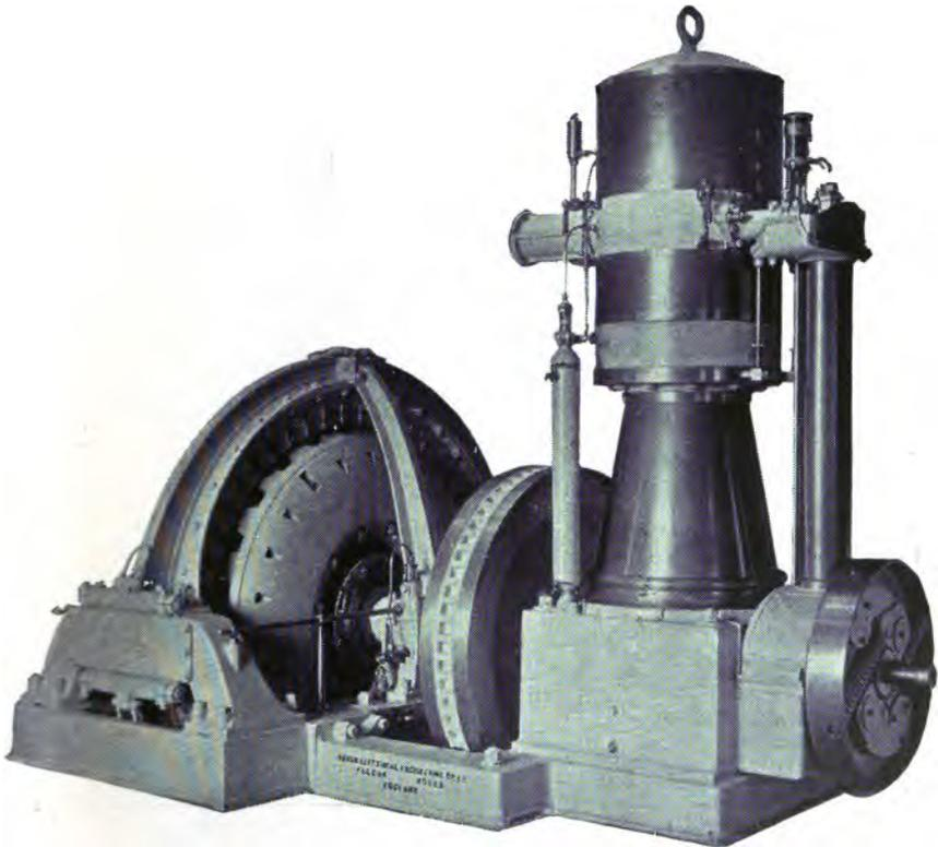
FIG. 45.—THE "UNIVERSAL" ENGINE COUPLED TO DYNAMO.
