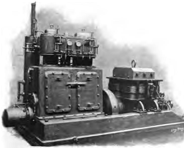
FIG. 24.—"ROBEY" COMPOUND ENGINE OF THE VALVE CLASS, SHOWN WITH DYNAMO.
