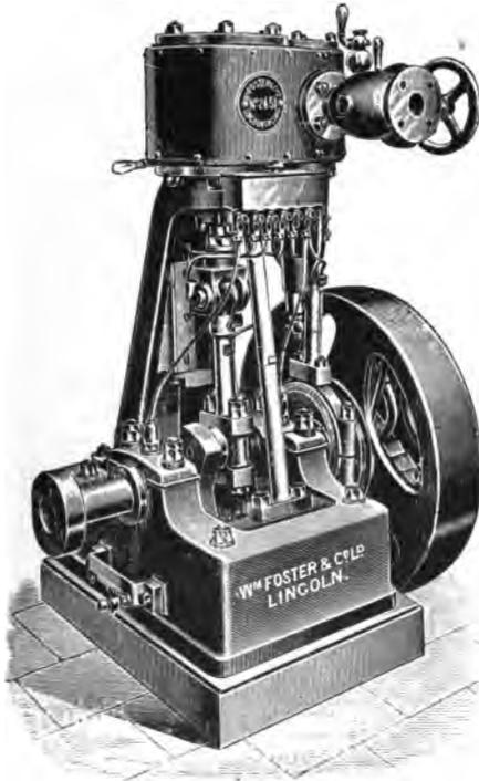
FIG. 156.—OPEN TYPE ENGINE, BY MESSRS. WM. FOSTER & CO., LIMITED, LINCOLN.
