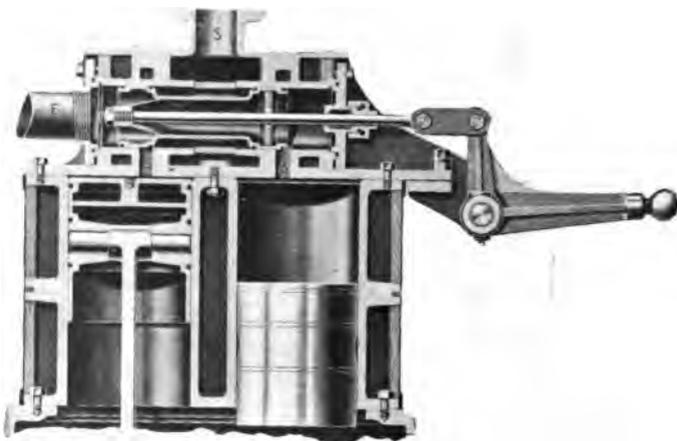
FIG. 89.—DETAIL SHOWING STEAM CHEST, CYLINDERS, VALVE AND PISTONS OF WESTINGHOUSE "JUNIOR."
