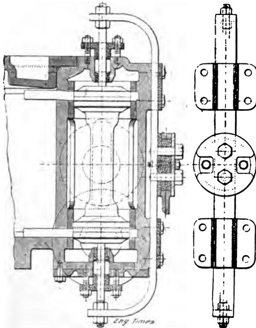
FIG. 57.—“ROBINSON AND AUDEN” ENGINE VALVE DRIVE.
