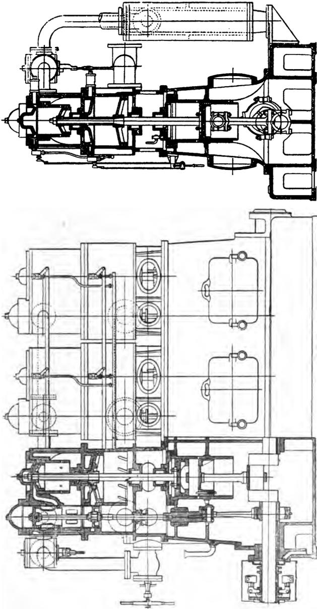
FIG. 138.—FRONT AND END SECTIONAL VIEWS OF MESSRS. ALLEY AND MACLELLAN'S 300 H.P. ENGINE.
