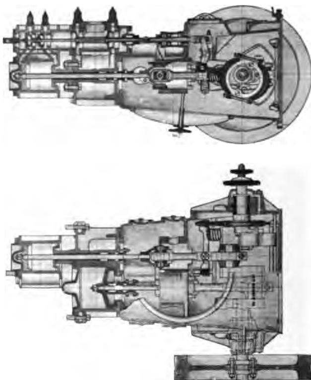
FIG. 154.—SECTIONAL VIEWS OF MESSRS. W. SISSON & CO.'S HIGH SPEED ENGINE.
