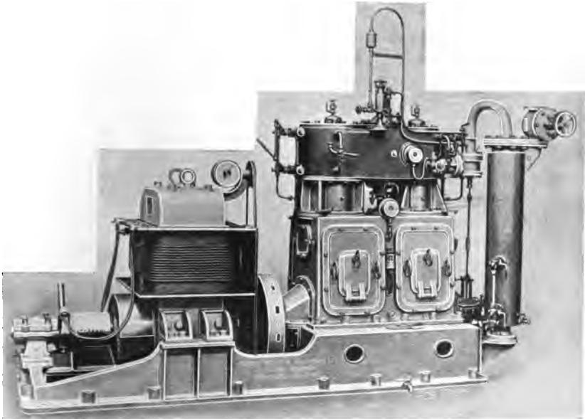
FIG. 31.—ERNEST SCOTT AND MOUNTAIN'S CENTRAL VALVE ENGINE, COUPLED TO A "TYNE" DYNAMO.
