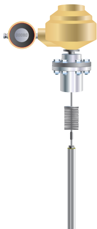
Figure 2.7.1 Illustration showing a spring displacer
