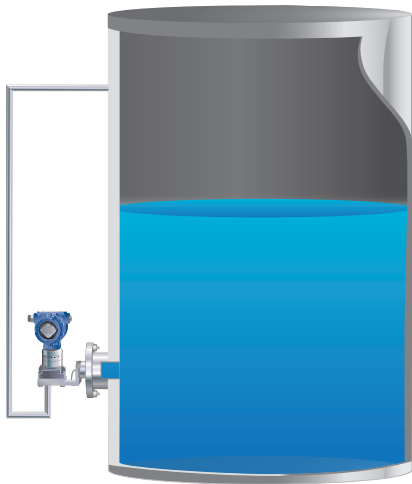
Figure 7.1.1: Illustration of a wet leg installation
