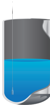
Figure 7.6.1: 9710 cable suspended mounting configuration
