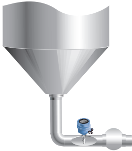
Figure 9.1.4: Pump protection or empty pipe detection
