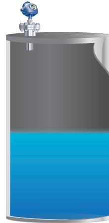
Figure 4.19.1: Water and boric acid storage with a non-contacting radar
