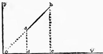
As before,  $H = S + W$ ; and  $S = w K_v (T_2 - T_1)$ ; where  $w$  is the weight of the air;  $T_2$  the final absolute temperature; and  $T_1$  the initial absolute temperature.
