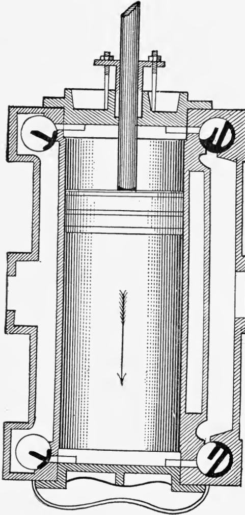
Fig. 19. Section of Cylinder of Corliss Engine.
