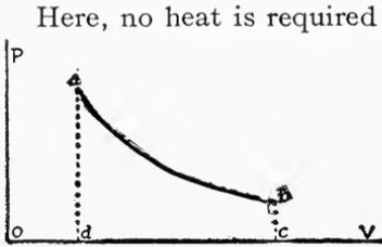
Here, no heat is required to change the temperature of the air; all is used in doing external work.
