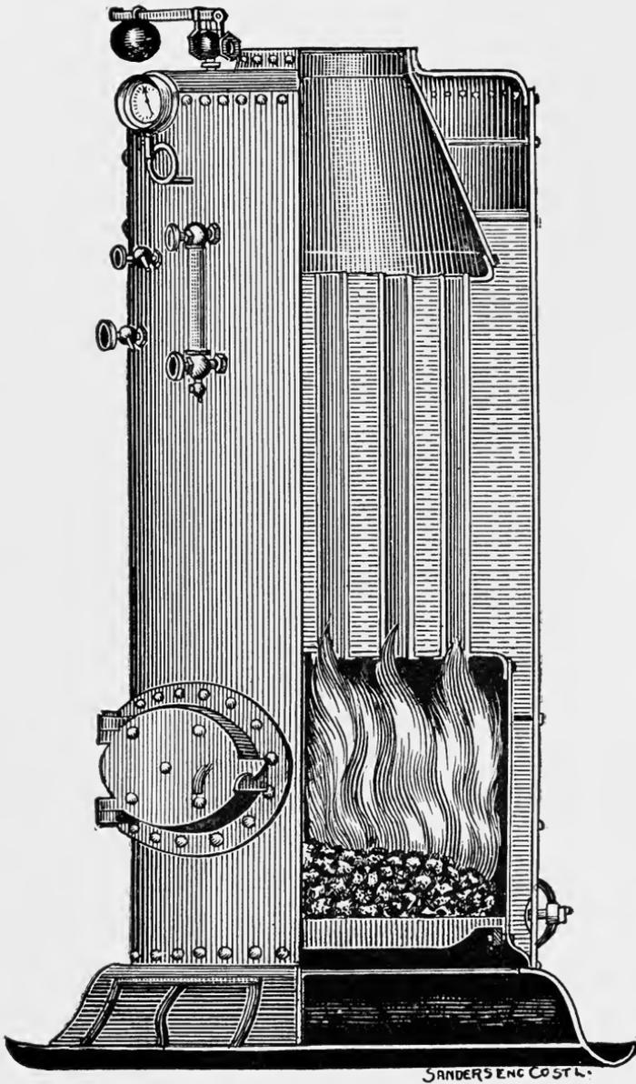
Fig. 86. Vertical Boiler.
