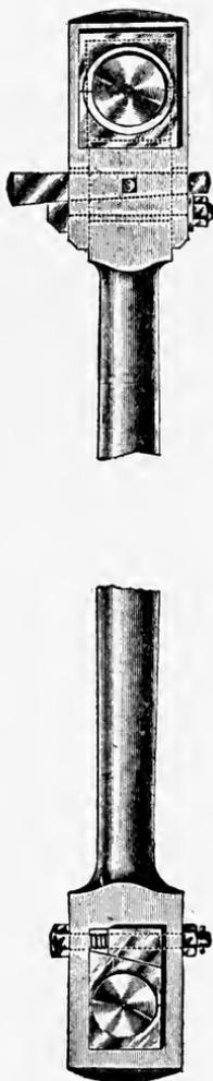
Fig. 25. Connecting Rod, Bates Corliss Engine.
