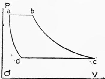
The work diagram is shown in the figure. Let the co-ordinates of  $a$  be  $V_1, P_1, T_1$ ; of  $b$  be  $V_2, P_1, T_2$ ; of  $c$  be  $V_3, P_2, T_2$ ; and of  $d$  be  $V_4, P_2, T_1$ .
