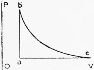
During the change from  $a$  to  $b$  the air is heated at constant volume, no work is done, and the heat put in during this change is  $K_v (T_2 - T_1)$ . During the change from  $b$  to  $c$  no heat is either given to, or emitted by, the air. During the change from  $c$  to  $a$  the
