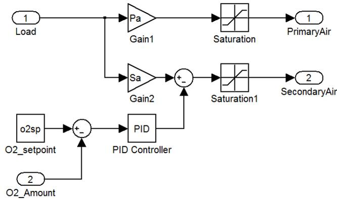
Figure 5.5: Block diagram of the air control system.
