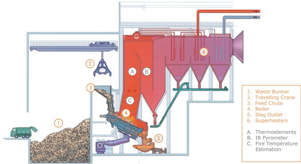
Figure 4.2: Illustration of Boiler 4 at Sysav (Sysav, 2010a)
