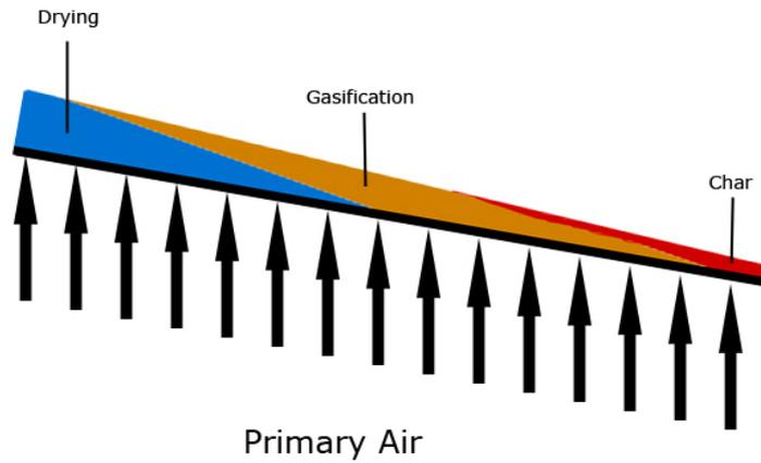
Figure 3.2: Combustion bed.
