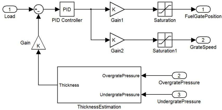
Figure 5.6: Block diagram of the fuel control system.
