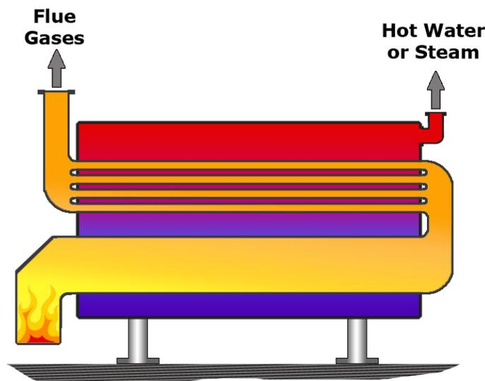
Figure 2.1: A two-pass firetube boiler.
