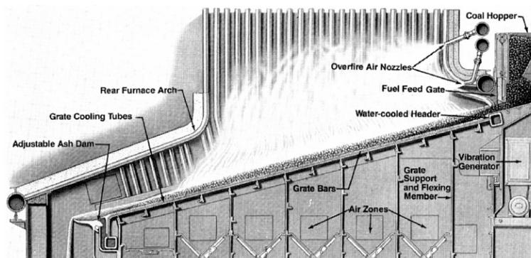
Figure 2.5: Cross-section of an overfeed massfeed stoker (Oland, 2002).
