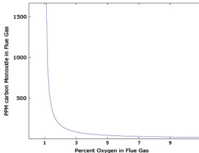
Figure 3.3: Hypothetical CO-O<sub>2</sub> characteristic curve.
