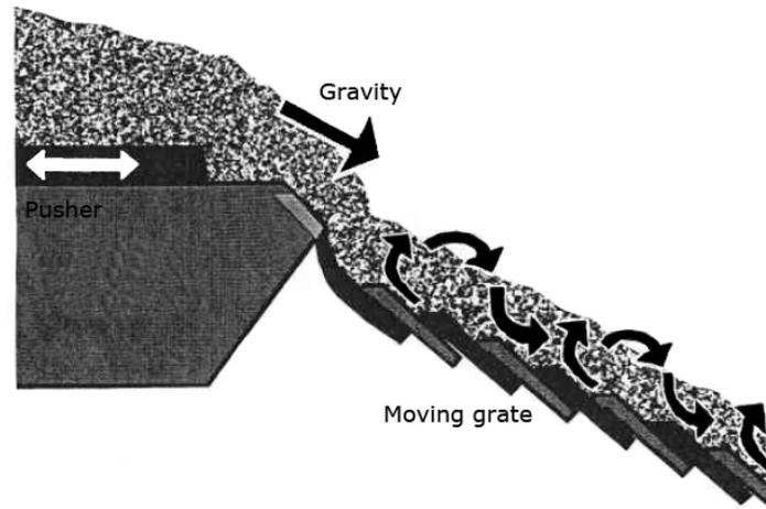
Figure 4.3: Principle of grate movement (MARTIN GmbH, 2008b).
