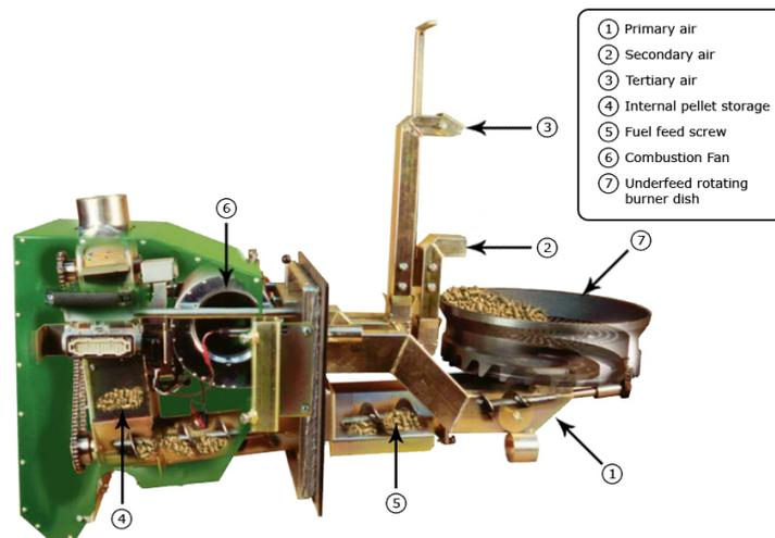
Figure 4.5: Illustration of EcoTec boiler (Sahlins EcoTec AB, 2008).
