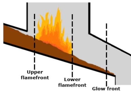
Figure 3.4: Illustration of the flame fronts and the glow front.
