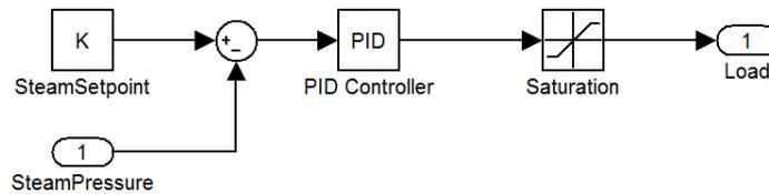
Figure 5.4: Block diagram of the load control system.
