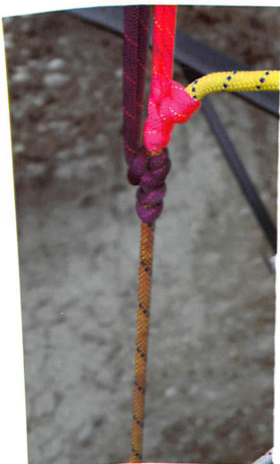
Drop testing Prusiks
