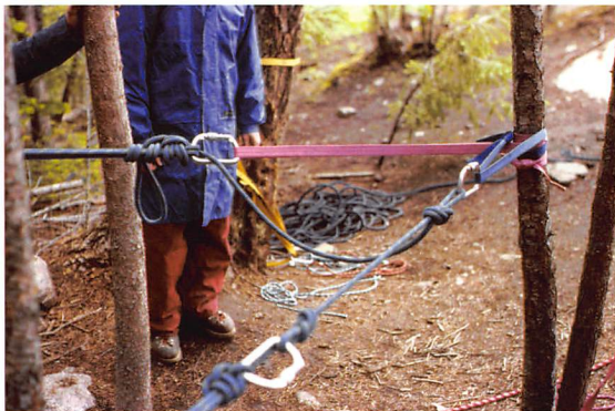
Fixed and focussed tie back anchor, Invermere B.C. Canada
